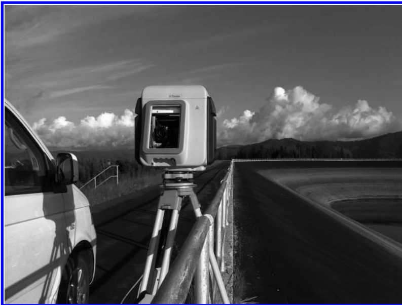
Figure 1. Pumping hydropower station Čierny Váh—3D laser scanning of asphalt-concrete surface of upper reservoir.
