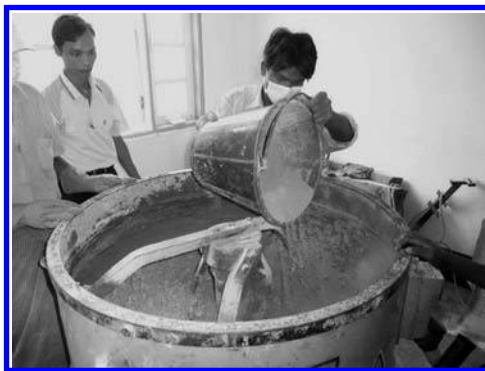
Figure 11. RCC trial mix in the laboratory.
