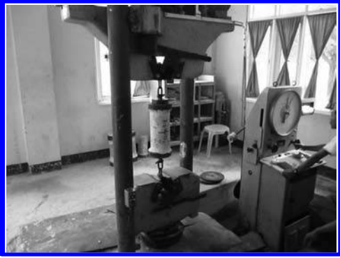
Figure 13. Tensile testing of RCC cores.
