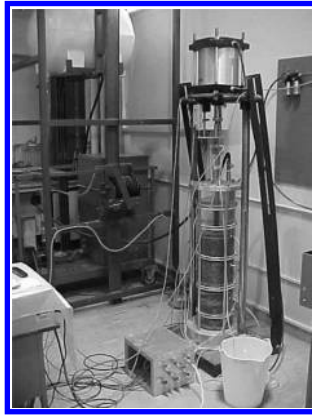
Figure 5. Photograph of permeameter test apparatus and setup.
