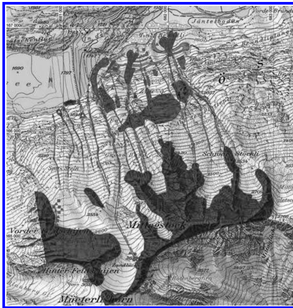
Figure 3. Map of rock fall, debris flow and selected transportation channels using standardized symbols and colours.
