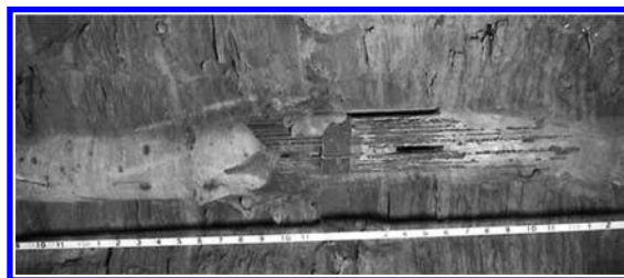
Figure 1. Section of test anchor installed using the Catagunya dam specification.
