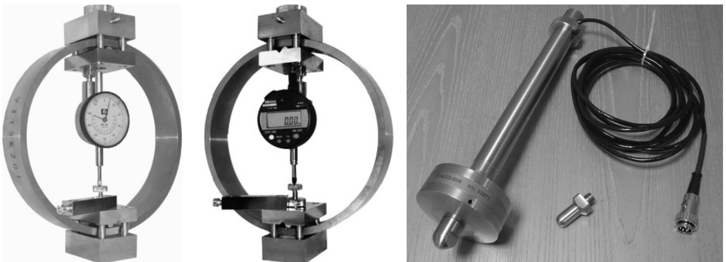
Figure 49.3 Triaxial load measuring equipment (Left: Load ring with manual dial gauge. Middle: Load ring with digital dial gauge. Right: Submersible electronic load cell) Courtesy of VJ Tech Ltd
