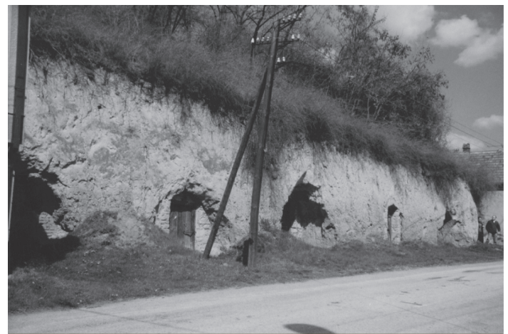
Figure 32.1 Example of loess in its pre-collapsed state exhibiting its relatively stiff soft rock state when dry, allowing the formation of man-made caves, Slovakia
