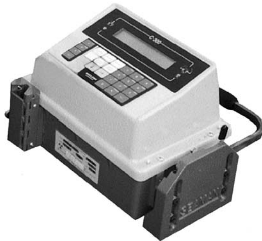
FIGURE 5.10 Nuclear density meter. (Photo courtesy of Seaman Nuclear Corp.)
