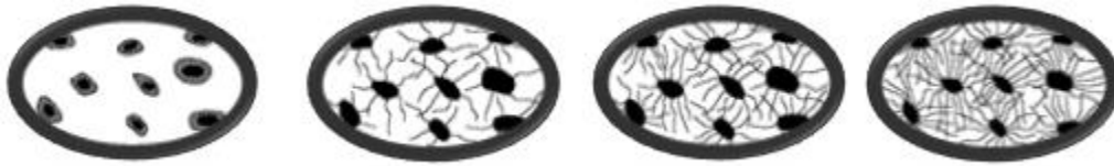
Fig: Structure of cement paste constituents
