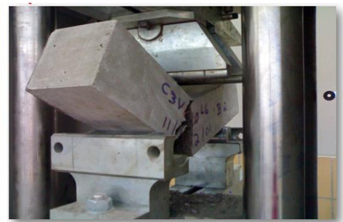
Destructive tests a) Bending test
