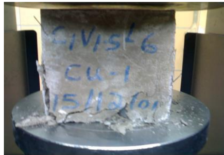
Destructive tests b) Compressive test
