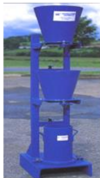
Compacting factor test
