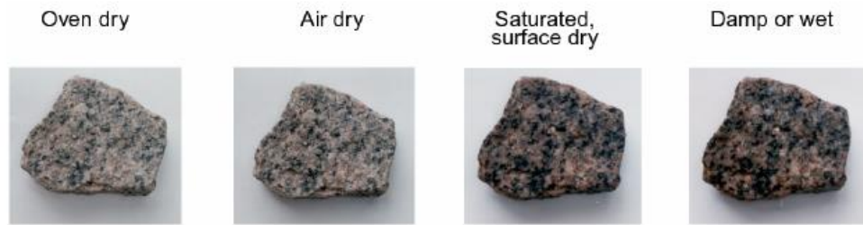
Granite aggregate at various moisture conditions
