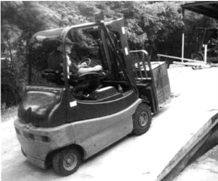
Figure 5-2. An Electric Outdoor Lift Truck Drives Up a Ramp With Ease at Springer Equipment Company in Birmingham, AL. (Source: Alabama Power Company)
