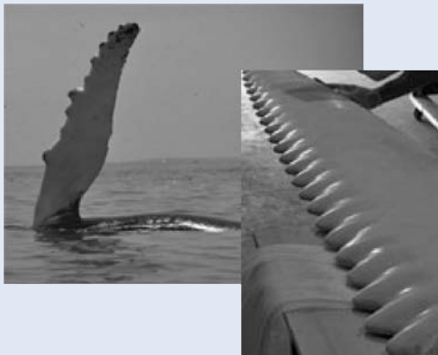
Humpback whale flipper and new airfoil design.
