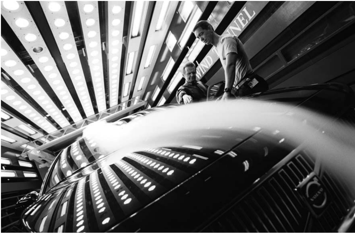
Fig. 7.4 Full-scale automobile under test in Volvo wind tunnel, using smoke streaklines for flow visualization. (Photograph courtesy of Volvo Cars of North America, Inc.)
