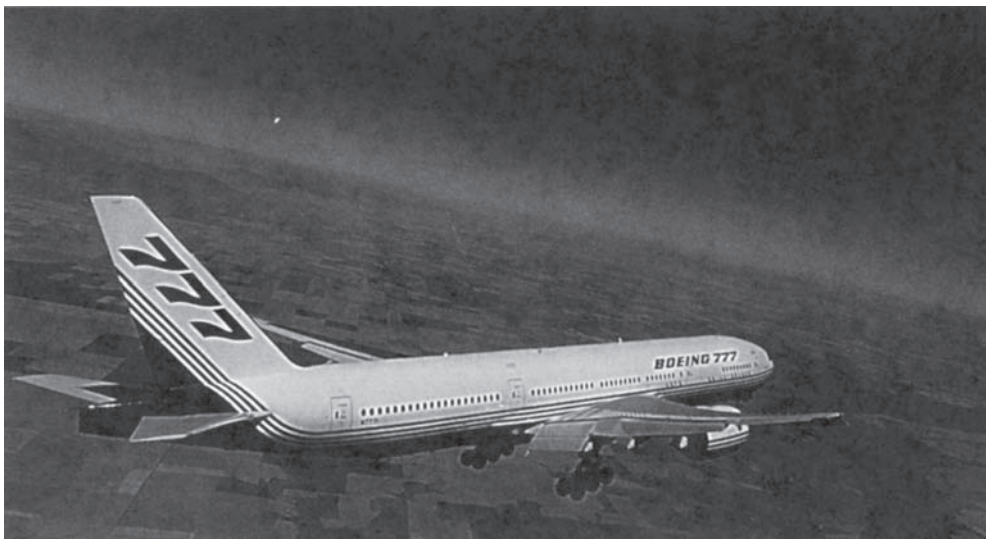
Fig. 9.24 (a) Application of high-lift boundary-layer control devices to reduce landing speed of a jet transport aircraft. The wing of the Boeing 777 is highly mechanized. In the landing configuration, large slotted trailing-edge flaps roll out from under the wing and deflect downward to increase wing area and camber, thus increasing the lift coefficient. Slats at the leading edge of the wing move forward and down, to increase the effective radius of the leading edge and prevent flow separation, and to open a slot that helps keep air flow attached to the wing's upper surface. After touchdown, spoilers (not shown in use) are raised in front of each flap to decrease lift and ensure that the plane remains on the ground, despite use of the lift-augmenting devices. (This photograph was taken during a flight test. Flow cones are attached to the flaps and ailerons to identify regions of separated flow on these surfaces.) (Photograph courtesy of Boeing Airplane Company.)
