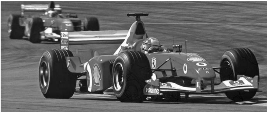
Fig. 9.26 Contemporary racing car (Schumacher's Formula 1 Ferrari) showing aerodynamic features. The car's front and rear wings are designed to provide significant downforce at speed to improve traction. Also visible are fairings to direct hot air from the radiators around the rear tires, and at the front of the car, cool air toward the brakes. Not shown are other aerodynamic features such as the fuselage bottom, which is designed to route the airflow carefully, using diffusers, to develop the most negative pressure, and to cause this negative pressure to act over the largest possible area under the car, to develop additional downforce. (Photograph © Wayne P. Johnson)
