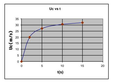
Note that the limiting case occurs when the cart velocity reaches the jet velocity. At this point, the jet can impart no more momentum to the cart, the acceleration is now zero, and the terminal velocity has been reached.
