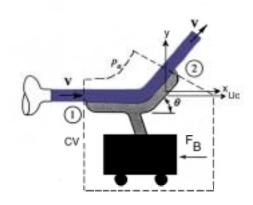
The transient term in the momentum equation is still zero. With the coordinate system on the cart, the momentum of the cart relative to the coordinate system is still zero. The fluid stream is still moving relative to the coordinate system, however, the flow is steady with constant velocity and the time rate of change of momentum of the fluid stream is therefore also zero. Thus
