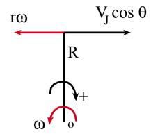
Taking the moment about the center of rotation, the moment of the inlet flow is zero since the moment arm is zero for the inlet flow.
