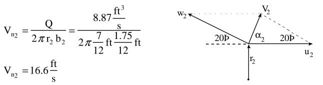
$$V_{t_2} = u_2 - w_2 \cos \beta_2 = 88 - 48.54 \cos 20^\circ = 42.4 \frac{\text{ft}}{\text{s}}$$
