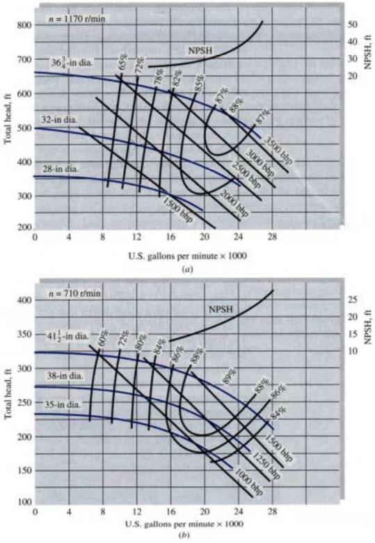
Fig. 11.7 Measured performance curves for two models of a centrifugal water pump
