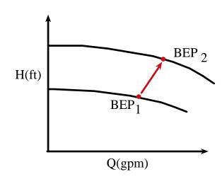
For the D = 38 in impeller of Fig. 11.7b operating at 710 rpm, we read the best efficiency point (BEP) values as
