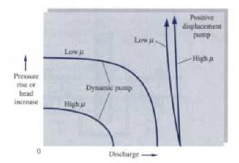
Fig. 11.2 Performance curves for dynamic and positive displacement pumps
