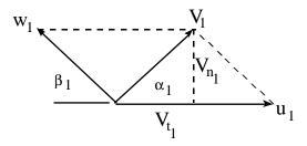
The absolute velocity can be resolved into two absolute velocity components:
