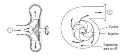
Fig. 11.3 Cutaway schematic of a typical centrifugal pump
