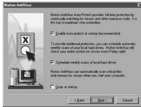
Figure 6.7 Auto-protection, weekly scans, and startup scan options for NAV 2000 during installation.
