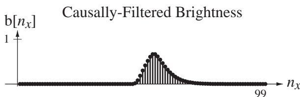
Figure 11.68 Brightness of the top row of pixels after being lowpass filtered by a causal lowpass filter
