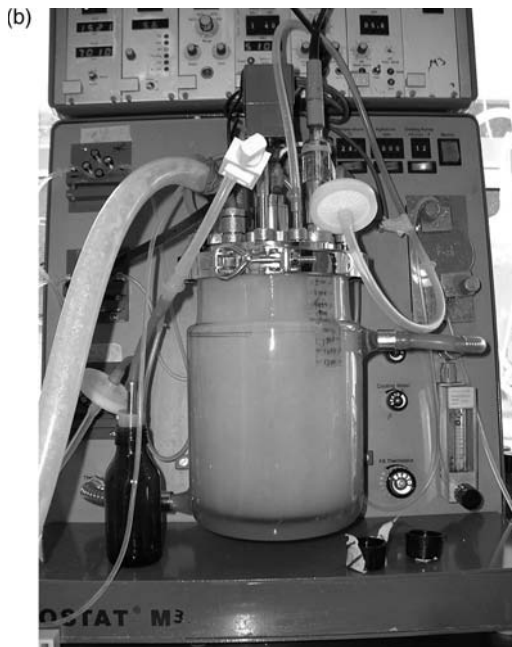
FIGURE 29.1 (a) Schematic of a bioreactor as used for fungal chemostat fermentations. (b) A typical laboratory chemostat fermenter.
