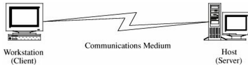
Figure 7-1. Simple View of Network.
