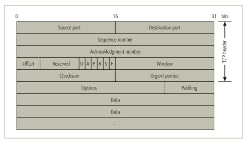
Figure 6-8 TCP packet structure
