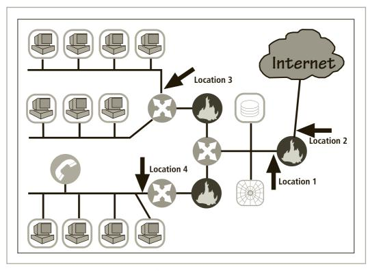
**Figure 7-8** Network IDPS sensor locations<sup>23</sup> Source: Adapted from Scarfone and Mell. NIST SP 800-94.
