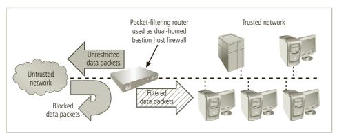
Figure 6-10 Packet-filtering router
