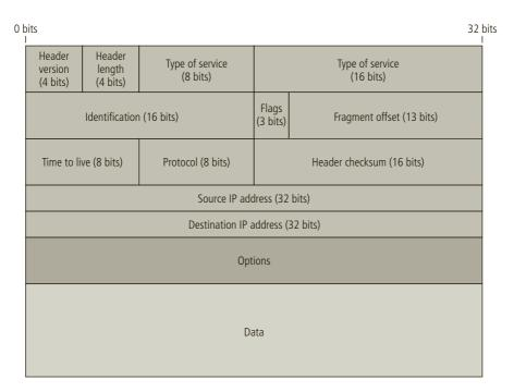
Figure 6-7 IP packet structure
