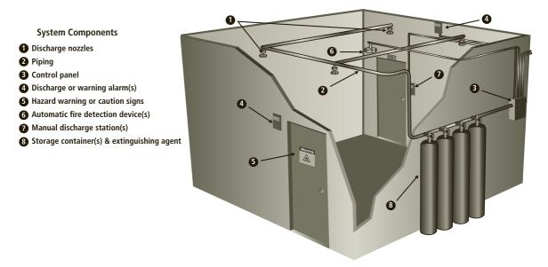
Figure 9-5 Gaseous fire suppression system
