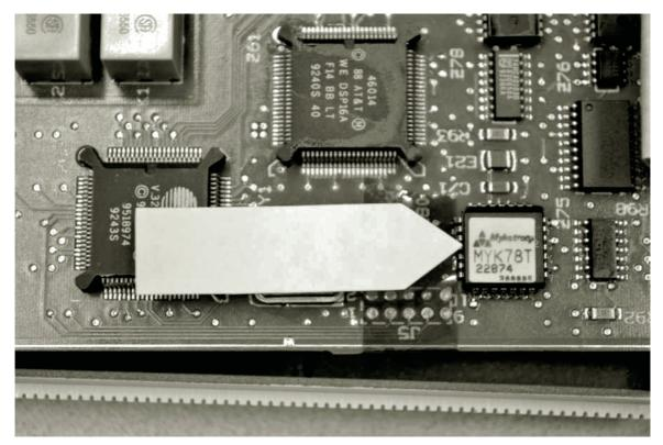
Figure 3-1 The Clipper chip<sup>7</sup>
