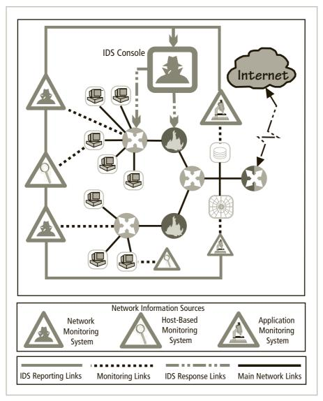
Figure 7-5 Centralized IDPS control<sup>20</sup>
