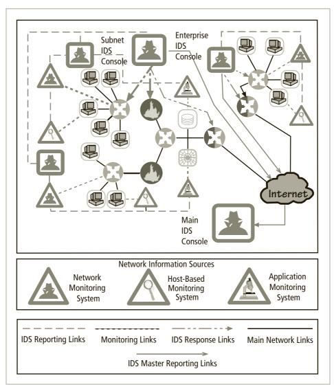
Figure 7-7 Partially distributed IDPS control<sup>22</sup>
