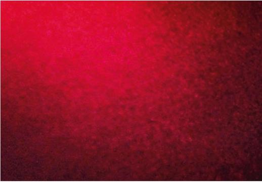
**Laser Speckle, Fig. 1** Laser speckle pattern observed for laser light scattered from a diffuse sample
