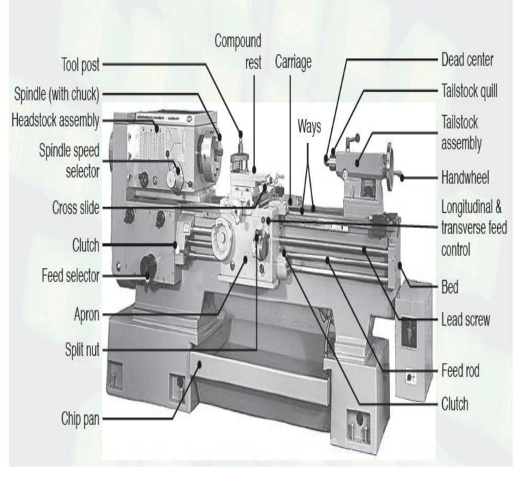
Figure.4 parts of lathe machine
