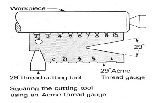
Figure 53. Square the cutting tool using an Acme thread gauge
