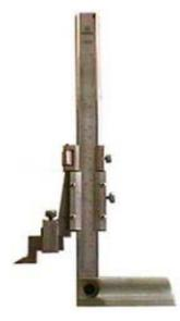
Figure62. vernier height gauge
