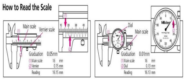
Figure 58. Vernier Reading system
