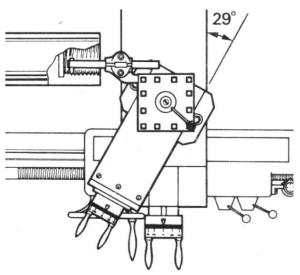
COMPOUND REST SET AT 29° TO THE LEFT TO CUT A 60° INCLUDED ANGLE RIGHT HAND INTERAL THREAD
