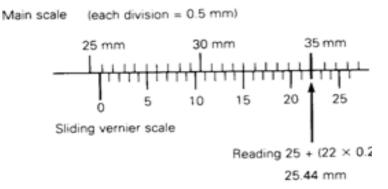
Figure 78. Taking a measurement with the vernier caliper.
