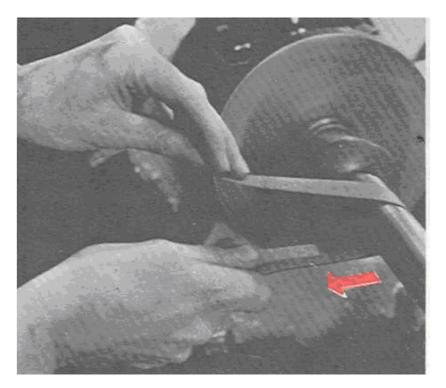
Figure 46. Using a strip of aluminum oxide (emery) cloth to polish the turned surface of a work piece.
