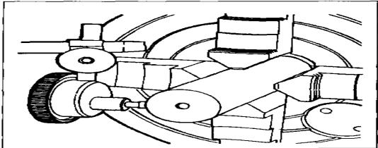
Figure7. Mounting work in a 4-jaw independent chuck
