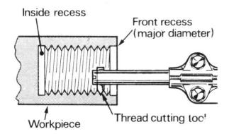
Cutting an internal thread
