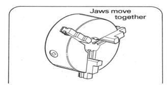
Figure16. Three – Jaw Self Centering Chick
