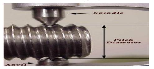
Figure 68. Screw thread micrometer
