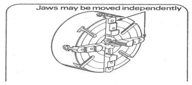
Figure 17. Four jaw independent chuck
