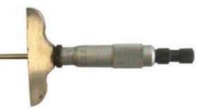
Figure 65. Depth Micrometer
