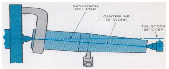
Figure38.Taper turning by offset tailstock method
