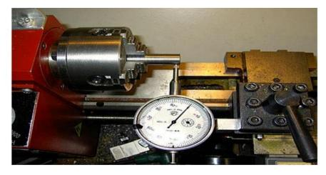
Figure13.center work in a 4-jaw chuck
