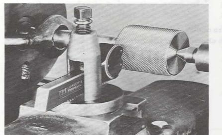
Figure 42. Diamond – point knurling of a cylindrical work piece
