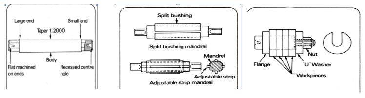
Figure23a. Standard solid mandrel Figure23b. Expansion mandrel
