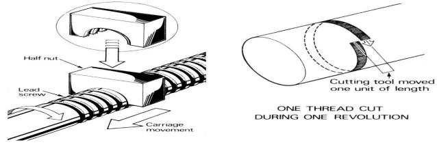
Figure44.Half nut engages lead screw to move carriage
