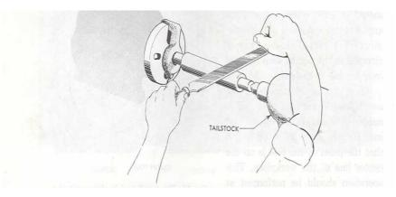
Figure 45. Filling a work piece mounted on a lathe
