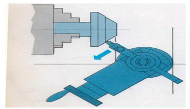
Figure37.Taper turning with compound rest
