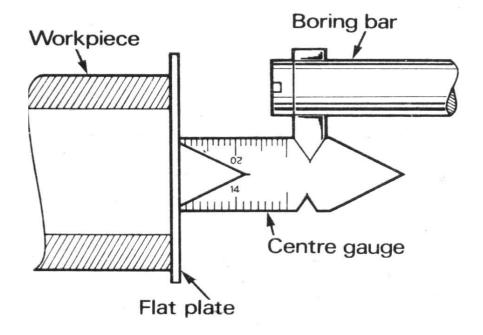
Figure 52. Squaring the cutting tool with a center gauge
