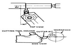
Figure36.Set up for straight turning
