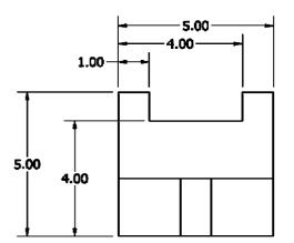
Figure.3 views using 3rd angle projection
