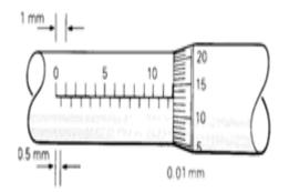
Figure 80. Micrometer reading
