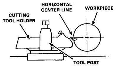
Figure35. Positioning tool bit for facing
