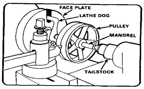
Figure 11.Pulley mounted on a mandrel
