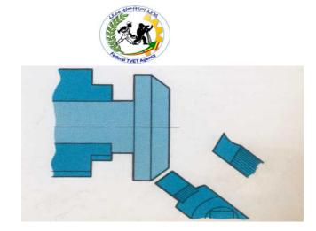
Figure40.Turning a tapper with form tool
