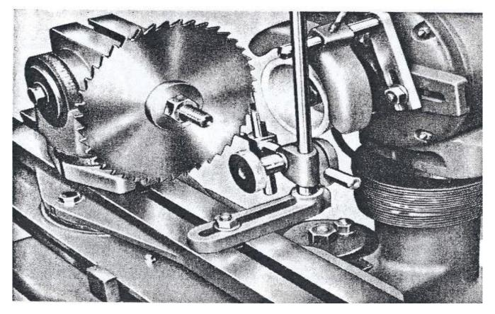
Figure 40. Sharpening Slitting Saw
