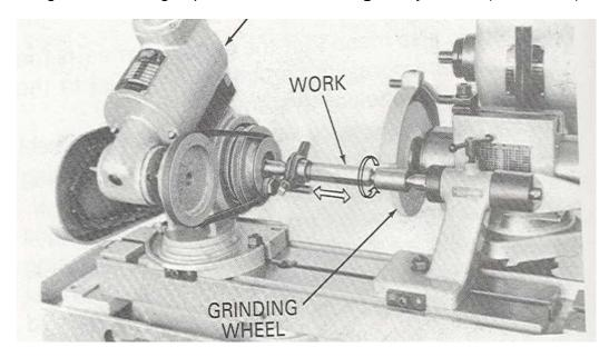
Figure 4.Tooth rest is being used to position teeth of cutter
