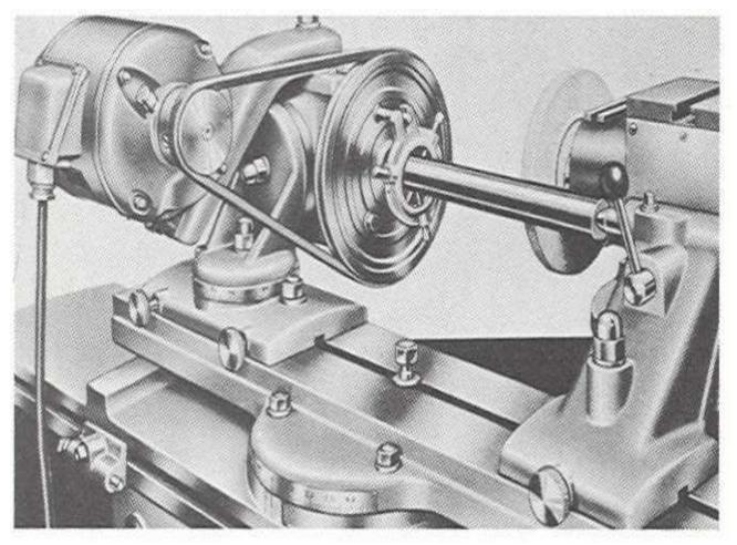
Figure32. Cylindrical grinding
