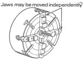
Figure 16.Four-Jaw Self Independent Chuck
