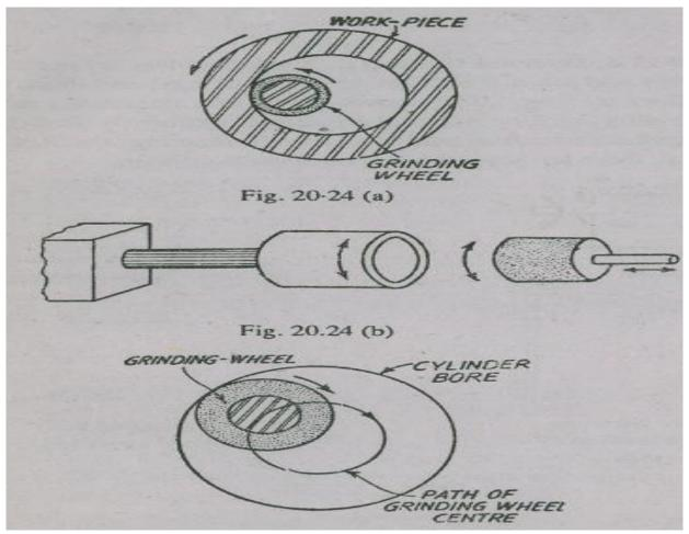
Figure35. Planetary type of grinding
