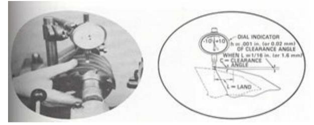
Figure 50. measuring the clearance angle with a dial indicator
