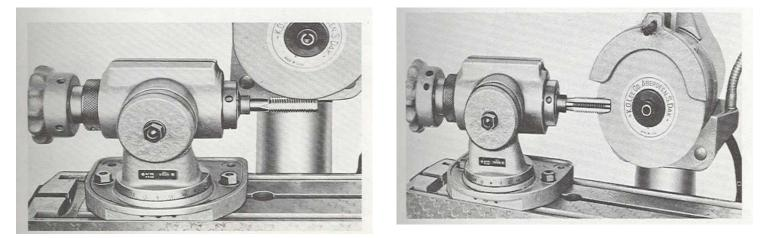
Figure30. Grinding Taps
