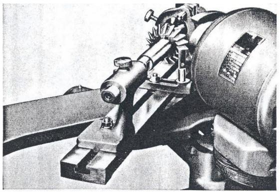
Figure 45. Sharpening Angle Cutter
