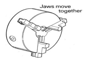
Figure 15. Three-Jaw Self Centering Chuck
