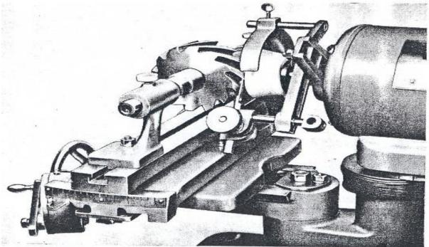
Figure 42. Grinding Periphery of Helical Slab Cutter
