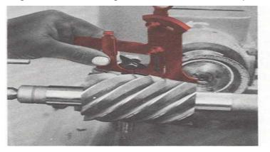
Figure 49.Checking the clearance angle with a Starrett cutter clearance gage
