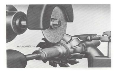
Figure 29. Grinding form cutters
