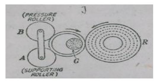
Figure36. Internal centre less grinding
