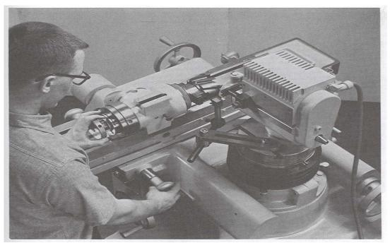
Figure28. Grinding end mills
