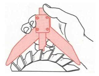
Figure 48. Checking the clearance angle with a brawn and sharpe clearance gage
