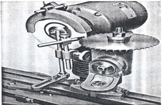
Figure 41. Regashing Slitting Saw
