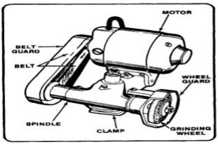
Figure24. Tool post grinding machine
