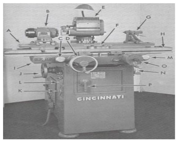
Figure 25. Parts of tool and cutter grinder
