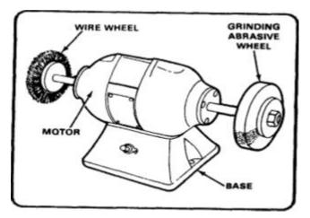
Figure 22. Bench-type utility grinding and buffing machine
