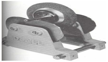
Figure10.A grinding wheel balancing stand
