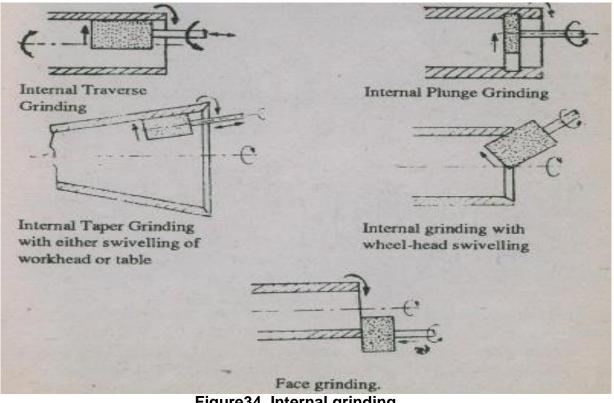
Figure34. Internal grinding
