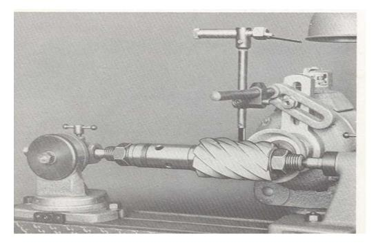
Figure27. Setup & grinding helical teeth cutters
