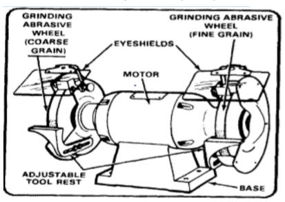
Figure 21. Bench type utility grinding machine
