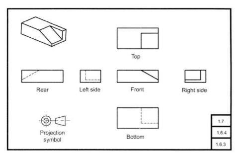
Fig 3 shows the six views of an object using 3<sup>rd</sup> angle projection
