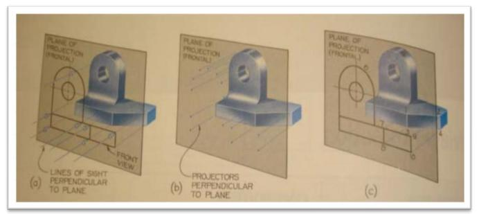
Fig. 1. projection of an object using front view
