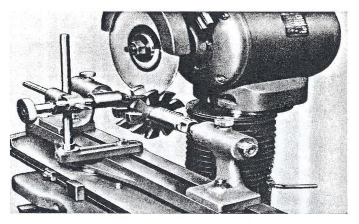
Figure 44. Sharpening Formed Milling Cutter
