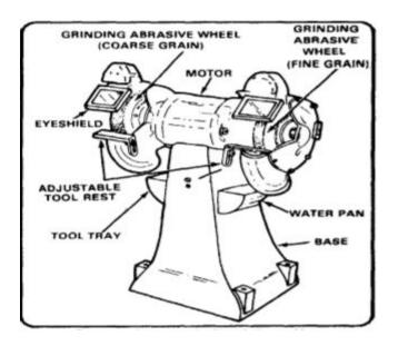
Figure 20. Floor-mounted utility grinding machine
