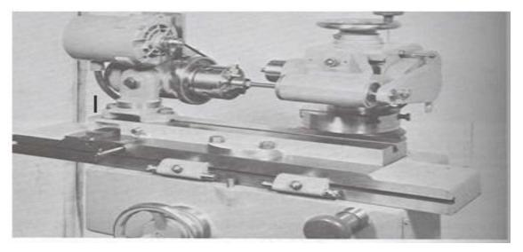
Figure33. Internal grinding
