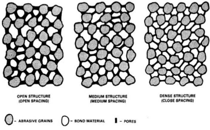
Figure7. Grinding wheel abrasive
