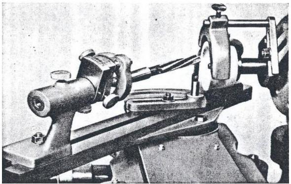
Figure 3. Grinding lead of reamer
