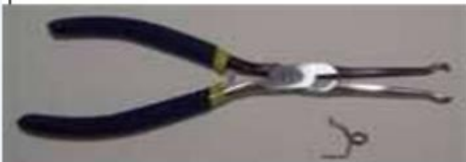
Long Nose Pliers with damage jaw
