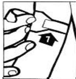
7 CORRECT TAPE TENSION
