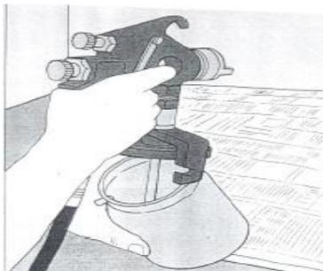
**Fig.6. Spraying lacquer thinner through a spray gun to clean it.**
