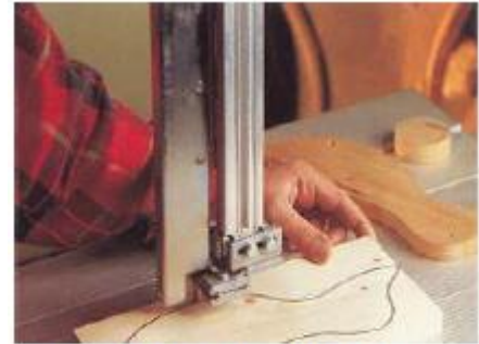
1. Freehand Cutting, guide the workpiece with both hands.
