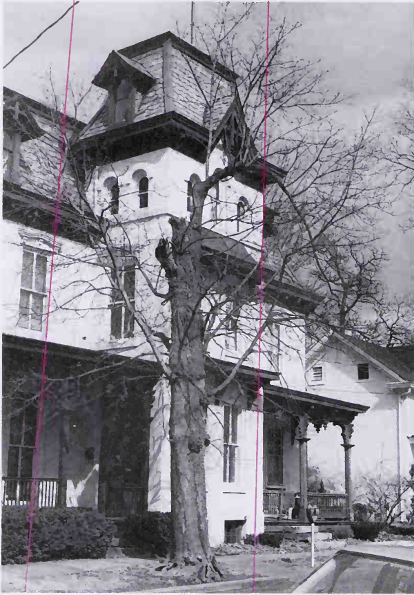
Photograph of a Victorian House in Doylestown, Pennsylvania, taken with a 50mm lens. Notice how vertical lines converge at the top because the camera had to be tilted to include the Italianate tower. This photo is not usable for a truthful interpretation.
