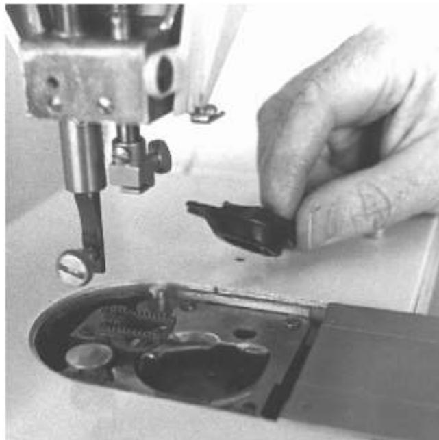
Fig. Bobbin Area – clean carefully to remove lint using a soft brush. Tweezers may be helpful in removing stray threads.
