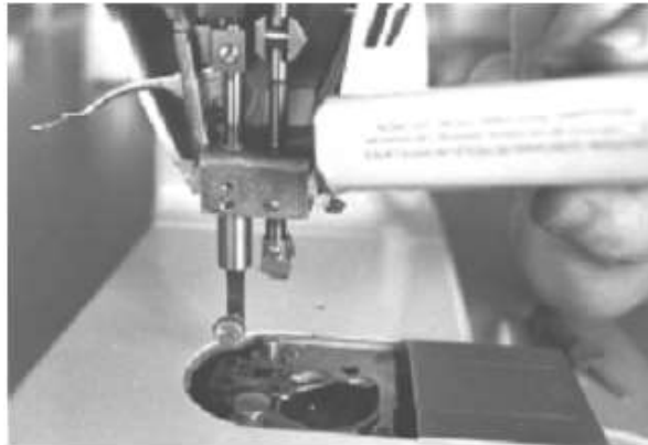
Fig. Faceplate Area – remove lint from faceplate area using a soft brush. A cloth dipped in solvent can be used to remove grease and grime.
