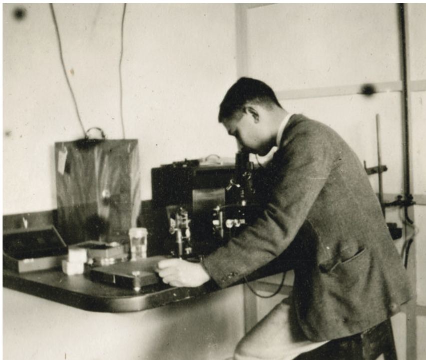
Fig. 3.7 J. Yudkin, as a graduate student working with the micromanipulator for isolating single bacteria (Archive of the Department of Biochemistry, University of Cambridge. Picture reproduced with the permission of the Archive)
