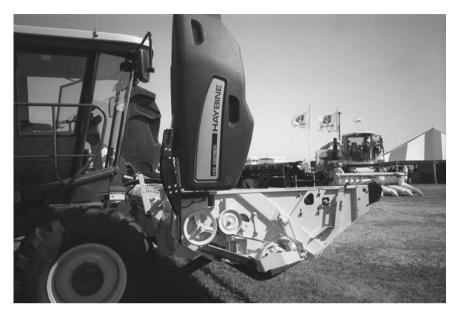
FIGURE 6.1. Hinged shield in raised (open) position for access.
