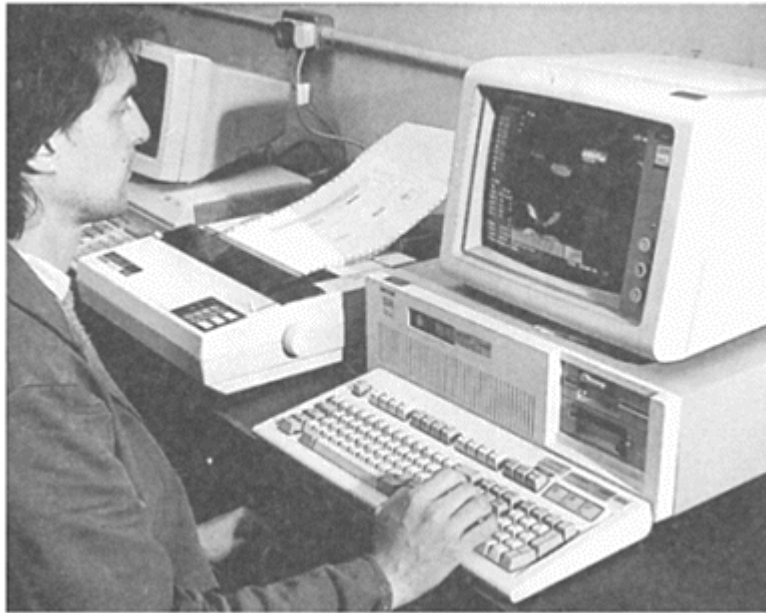
FIG. 5. Analysis and reporting of data stored on floppy disk by the P-scan system, using a personal computer.
