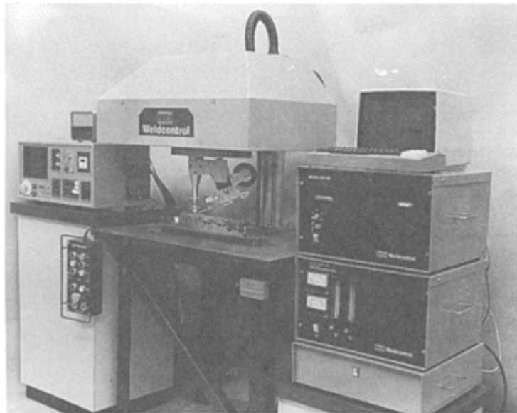
FIG. 19. TIG plus filler blade tipping system incorporating weld control, microprocessor controlled transistorised power source and PNC four-axis controller.
