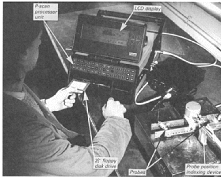
FIG. 4. Ultrasonic testing using the portable computerised P-scan system, being operated in ultrasonic pitch-catch mode.
