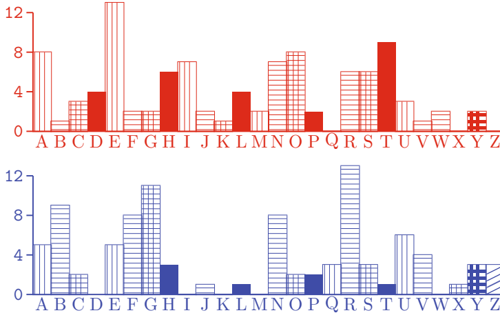
FIGURE 7.2. Comparison of plaintext and ciphertext frequencies for the shift cipher example
