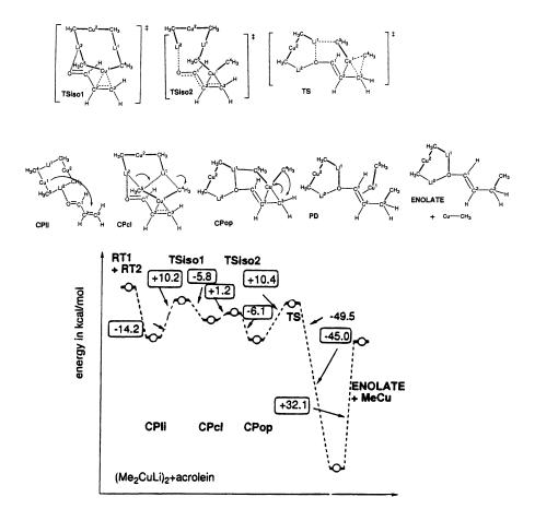
Fig. 8.5. Computational reaction profile (B3LYP/631A) for reaction of  $[(CH_3)_2CuLi]_2$  with acrolein. Adapted from *J. Am. Chem. Soc.*, **119**, 4900 (1997), by permission of the American Chemical Society.
