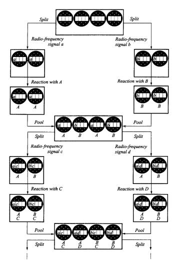
Fig. 13.3. Radio-frequency tagging of microreactors for combinatorial synthesis on a solid support. Reproduced from K. C. Nicolaou, X.-Y. Xiao, Z. Parandoosh, A. Senyei, and M. P. Nova, *Angew. Chem. Int. Ed. Engl.*, **34**, 2289 (1995), by permission of Wiley-VCH.
