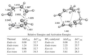
Fig. 6.6. Relative energies of four possible transition structures for Diels-Alder reaction of 1,3-butadiene and propenal, with and without  $BF_3$ catalyst. Geometric parameters of the most stable transition structures (*endo-cis*) are shown. Adapted from *J. Am. Chem. Soc.*, **120**, 2415 (1998), by permission of the American Chemical Society.
