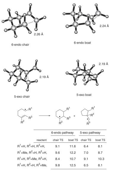
Fig. 10.14. Relative energies of 5-*exo* and 6-*endo* transition structures. Insert shows the effect of methyl substituents. Reproduced from *J. Am. Chem. Soc.*, **125**, 4271 (2003), by permission of the American Chemical Society.
