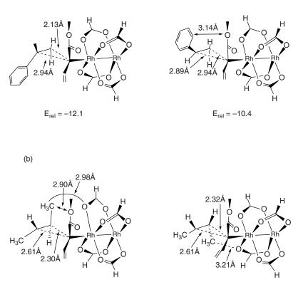
Fig. 10.10. Steric interactions in rhodium-catalyzed addition of methyl 2-diazobut-3-enoate to styrene (a) and *cis* and *trans* butene (b). Reproduced from *J. Am. Chem. Soc.*, **125**, 15902 (2003), by permission of the American Chemical Society.
