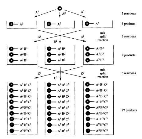
Fig. 13.1. Splitting method for combinatorial synthesis on solid support. Reproduced from F. Balkenhohl, C. von dem Bussche-Huennefeld, A. Lansky, and C. Zechel, *Angew. Chem. Int. Ed. Engl.*, **35**, 2288 (1996), by permission of Wiley-VCH.
