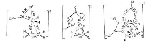
Fig. 10.5. Transition structures for  $CH_2$  transfer from  $ClCH_2ZnCl_2$  and  $ClZnCH_2Cl-ZnCl_2$  to ethene and to coordinated allyl alcohol. Reproduced from *J. Am. Chem. Soc.*, **125**, 2341 (2003), by permission of the American Chemical Society.
