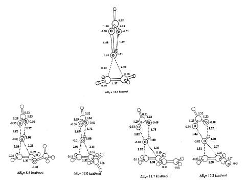
Fig. 12.8. Comparison of epoxidation transition structures and activation energies for ethene and substituted ethenes. Reproduced from *J. Am. Chem. Soc.*, **119**, 10147 (1997), by permission of the American Chemical Society.
