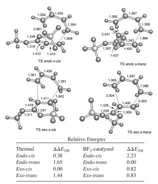
Fig. 6.7. Transition structures for the reaction between 1,3butadiene and the methyl acrylate $-BF_3$  complex calculated at the ab initio HF/6-31G\* level. Relative energies are in kcal/mol. Adapted from *Tetrahedron*, **53**, 6057 (1997), by permission of Elsevier.
