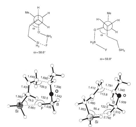
Fig. 9.2. Most favorable transition structures for reaction of allylsilane with acetaldehydefluoroborane: (left) *anti* synclinal; (right) *syn* synclinal. Reproduced from *J. Am. Chem. Soc.*, **119**, 12131 (1997), by permission of the American Chemical Society.
