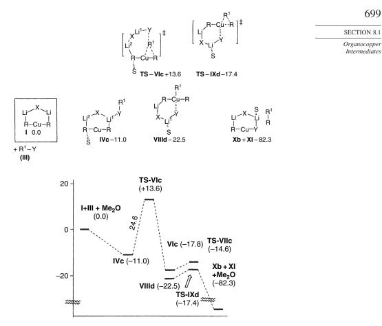
Fig. 8.2. Computational energy profile (B3LYP/631A) for reaction of  $(CH_3)_2$ CuLi-LiCl with  $CH_3Br$  including one solvent ( $CH_3OCH_3$ ) molecule. Adapted from *J. Am. Chem. Soc.*, **122**, 7294 (2000), by permission of the American Chemical Society.
