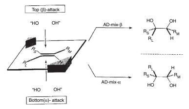
Fig. 12.1. Predictive model for enantioselective dihydroxylation by dimeric alkaloid catalysts. (DHQD)<sub>2</sub> catalysts give  $\beta$ -approach; (DHQ)<sub>2</sub> catalysts give  $\alpha$ -approach. Reproduced from *J. Org. Chem.*, **57**, 2768 (1992), by permission of the American Chemical Society.
