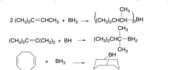
Hydroboration is a stereospecific *syn* addition that occurs through a four-center TS with simultaneous bonding to boron and hydrogen. The new C–B and C–H bonds are thus both formed from the same face of the double bond. In molecular orbital terms, the addition is viewed as taking place by interaction of the filled alkene  $\pi$  orbital with the empty *p* orbital on boron, accompanied by concerted C–H bond formation.<sup>158</sup>
