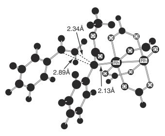
Fig. 10.9. Computed transition structure for addition of methyl phenyldiazoacetate to styrene from B3LYP/6-31G\*/LANL2DZ computations. Reproduced from *J. Am. Chem. Soc.*, **125**, 15902 (2003), by permission of the American Chemical Society.
