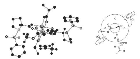
Fig. 10.11. General schematic model for favored approach of alkenes to 1-arenesulfonylprolinate catalysts (right); and B3LYP/6-31G\*/LANL2DZ computational model of preferred approach of propene to 1-carbomethoxyprop-2-enylidene complex with Rh<sub>2</sub>(1-benzenesulfonylprolinate)<sub>2</sub>(isobutyrate)<sub>2</sub> (left). Reproduced from *J. Am. Chem. Soc.*, **125**, 15902 (2003), by permission of the American Chemical Society.
