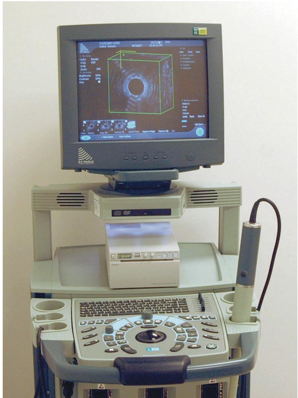
FIGURE 4-9. B-K Medical (Herlev, Denmark) three-dimensional anorectal ultrasound equipment.
