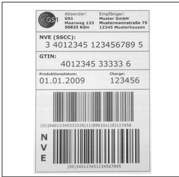
Fig. 9.8 EAN-128 transport label – concrete example of SSCC (Cf. GS1 Germany (2009a), p. 25)
