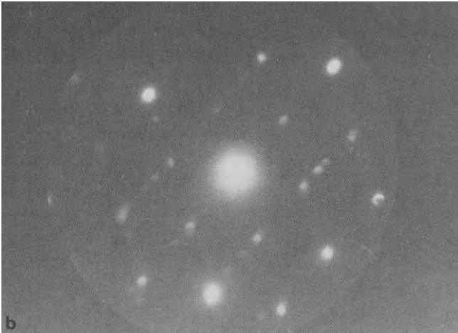
Fig.8.4a,b. Single-twinned gold particle produced by evaporated onto NaCl. a) Weak-beam image, b) microdiffraction pattern
