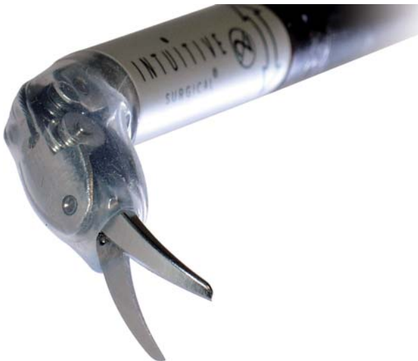
FIGURE 2.13. da Vinci Endowrist with three additional DoF.
