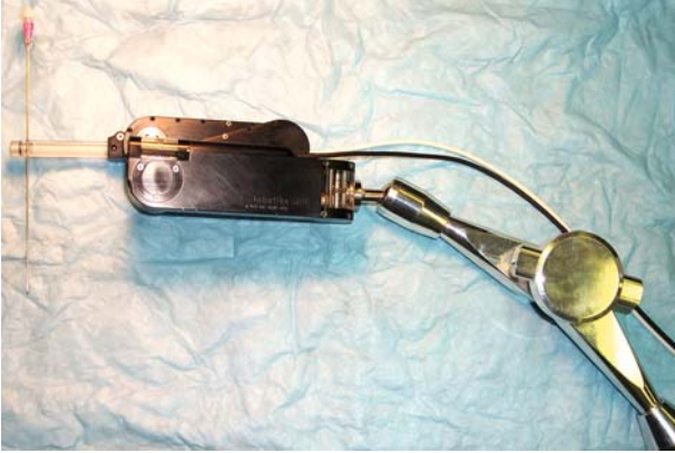
FIGURE 2.5. The RCM robot (Courtesy of: URobotics Laboratory, Johns Hopkins University).
