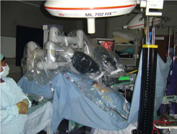
FIGURE 9.2. Robot docked in position during RALP. The patient's head is towards the right of the picture, concealed under drapes. Note the steep Trendelenburg position.
