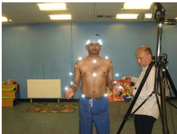
FIGURE 5.10 Assessment of surgical fatigue by motion analysis in a gait laboratory (Courtesy of: Adam Shortland).
