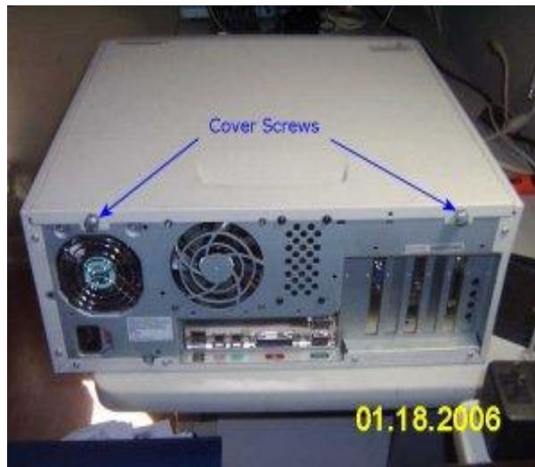
Fig 6.7 Location of Cover screws.
