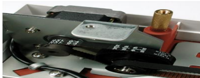
Fig1.28 The precision of the stepper motor determines the y-direction Sampling rate
