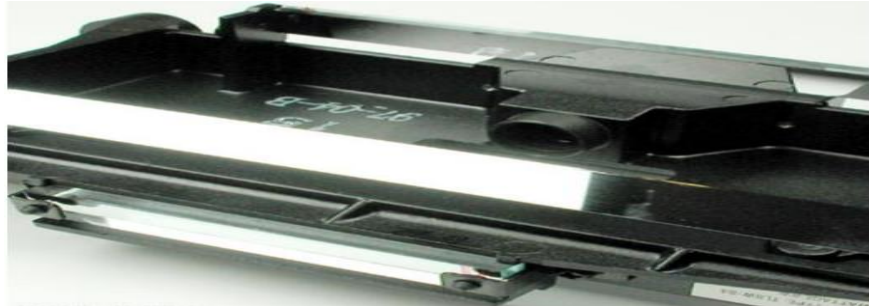
Fig1.26 Look carefully at the image above and you can see all three of the mirrors plus the lens assembly in this scan head.
