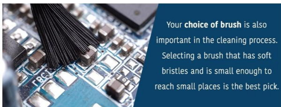
Fig 6.3 using brush to clean PCB
