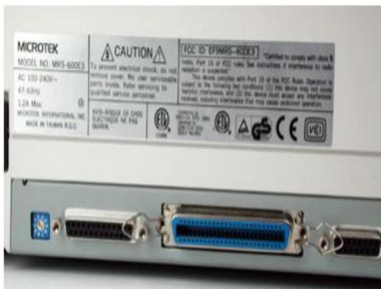
Fig 1.29 scanner may have more than one way of connecting to your computer. On your computer, you need software, called a driver that knows how to communicate with the scanner.
