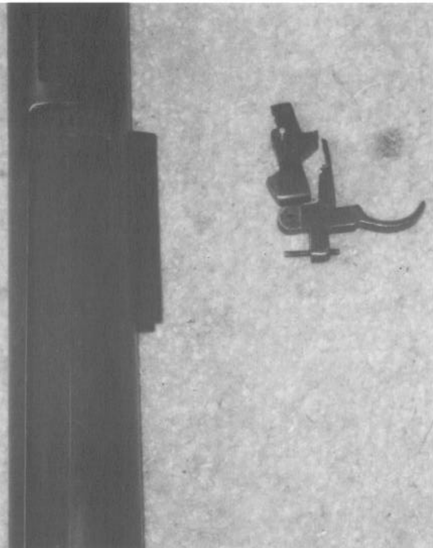
Trigger and sear ready for mounting.
