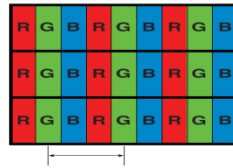
Figure 4.Stripe-shaped subpixels in a linear arrangement, where pixel pitch is the distance between same color subpixel stripes.
