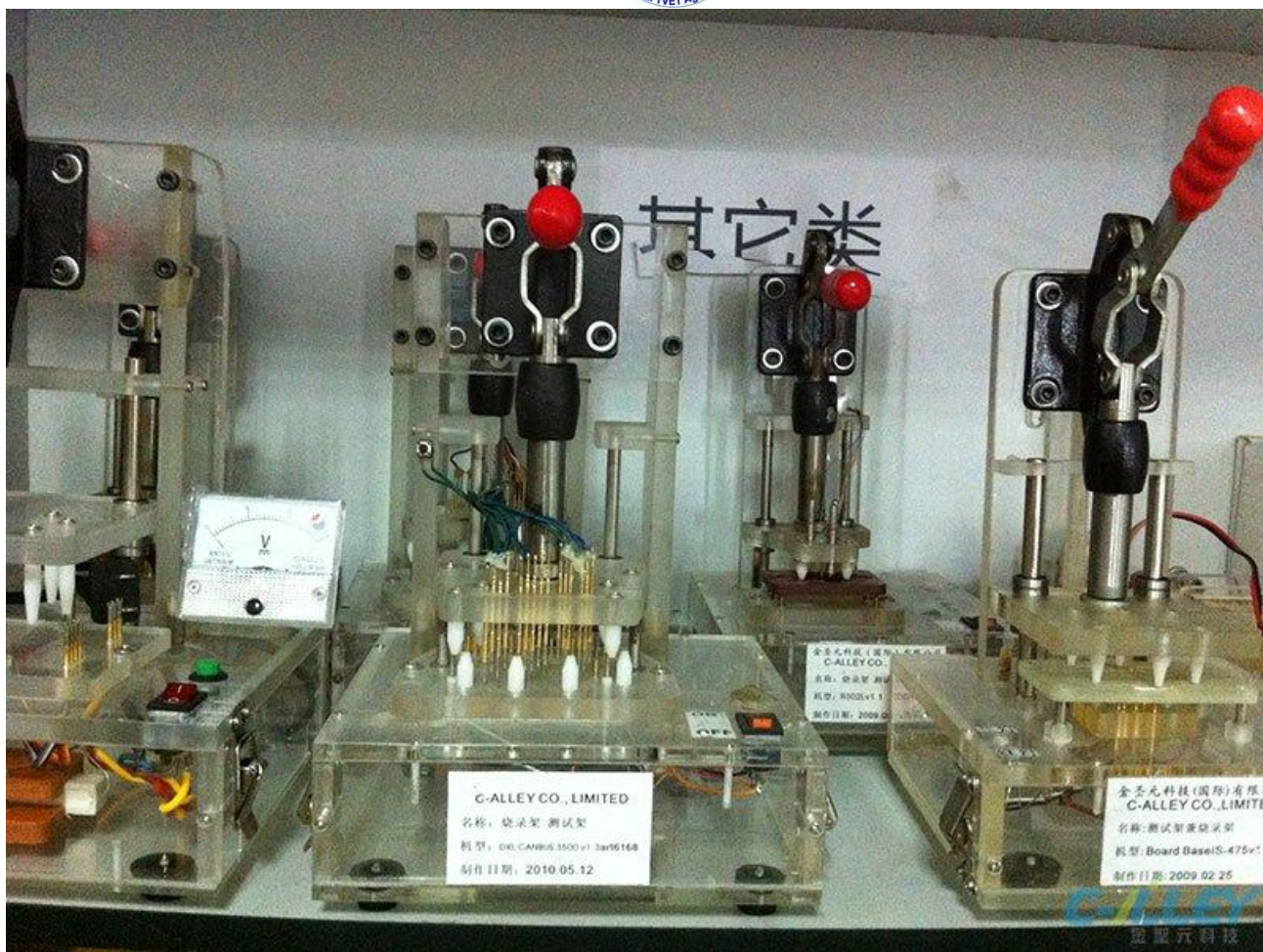
Figure. testing jig
