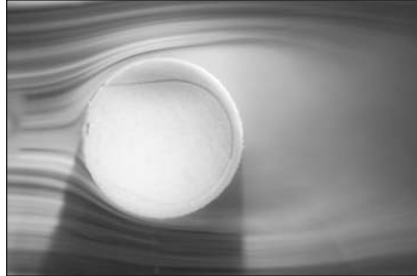
FIGURE 1–16 External flow over a tennis ball, and the turbulent wake region behind. Courtesy NASA and Cislunar Aerospace, Inc.
