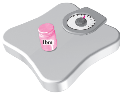
FIGURE 1-33 A mass of 1 lbm weighs 1 lbf on earth.
