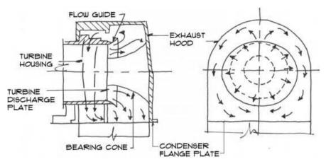
Figure 6.8 Exhaust diffuser of an LP turbine
