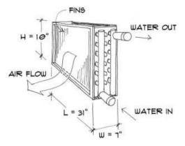
A detailed schematic drawing that shows an exploded view of the heat exchanger is also shown. It is not typical to show, in routine design problems, this type of schematic drawing with an exploded view. However, it will be required for fabrication of the coil. Additional information on dimensions would also be required.
