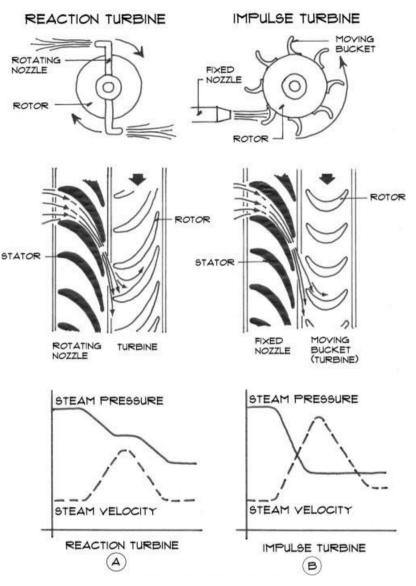
Figure 6.7 Turbine operation
