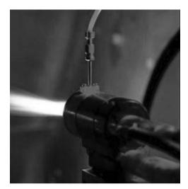
Figure 5.1 A Praxair SG-100 plasma spray torch in operation
