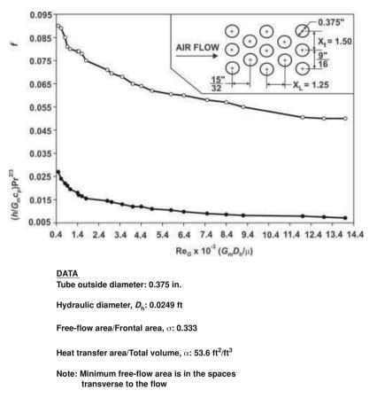
Figure 4.17 Data for flow normal to a staggered tube bank (Kays and London (2))
