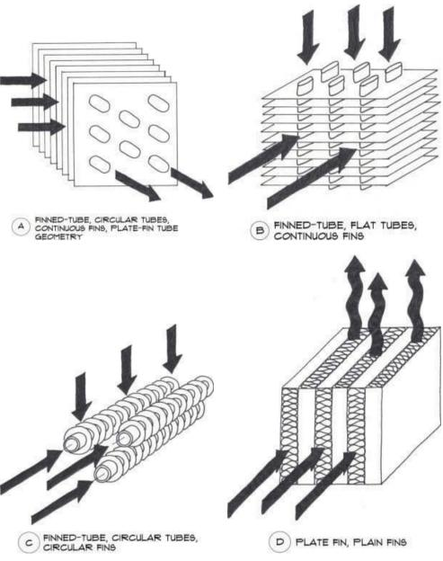
Figure 4.19 Examples of finned heat exchangers
