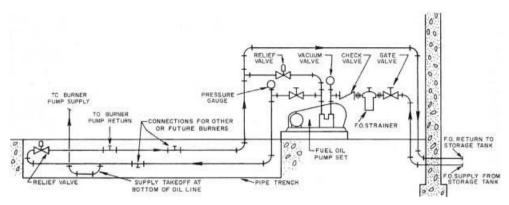
**Figure 3.2** A typical fuel oil piping system complete with a pump set (*ASHRAE Handbook*, Fundamentals Volume, 2005; reprinted with permission)
