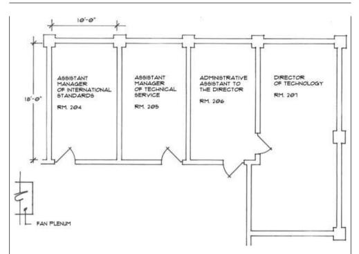
For the offices shown in the plan above (complete with the occupant and work function), the architect has requested the design of a ductwork system to provide air at 75°F to heat the occupied spaces. A HVAC engineer has determined the amount of air required to maintain the space temperature, and they are shown in the following table.
