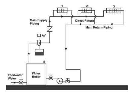
Figure 5.14 Schematic of a two-pipe direct return system
