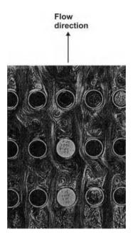
Figure 4.14 Flow pattern for an in-line tube bank (Çengel (3), reprinted with permission)
