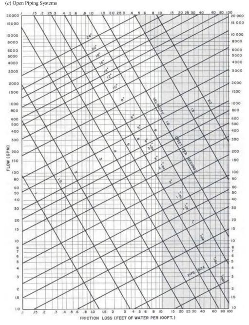
**Figure A.4** Commercial steel pipe (Schedule 40) friction loss. (a) *Open piping systems* (Carrier Corp.; reprinted with permission); (b) *closed piping systems* (Carrier Corp.; reprinted with permission)
