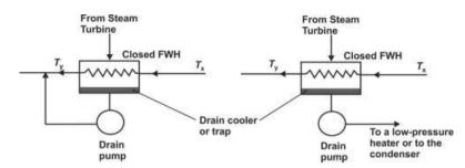
Figure 6.6 Drain disposals for closed feedwater heaters (surface heaters)
