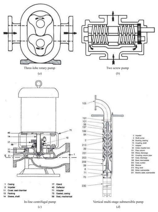
**Figure 3.6** Types of industrial pumps: (a) three-lobe rotary pump; (b) two-screw pump; (c) in-line centrifugal pump; (d) vertical mutistage submersible pump (Hydraulic Institute, Parsippany, NJ, www.pumps.org; reprinted with permission)
