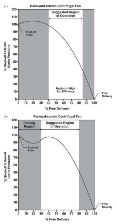
Figure 2.7 Typical performance curves of centrifugal fans
