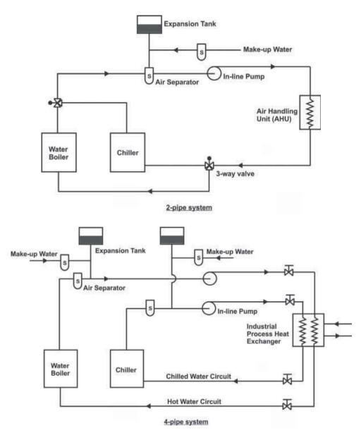
Figure 3.13 Diagrams of closed-loop piping systems
