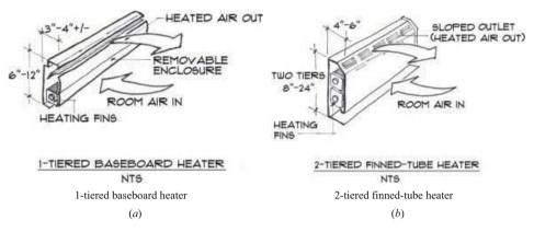
Figure 5.18 Diagrams of baseboard heaters. (a) 1-tiered baseboard heater; (b) 2-tiered finned-tube heater
