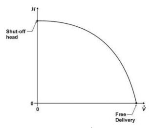
Figure 3.7 Schematic of a  $H_{pump}$  versus  $\dot{V}$  curve for a centrifugal pump
