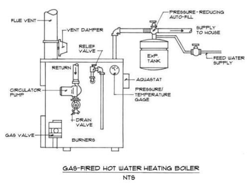
Figure 5.6 A typical gas-fired hot water boiler
