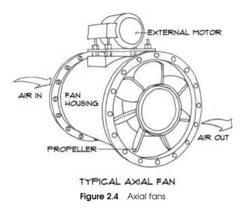
enclosure. A tubeaxial or vaneaxial fan is a propeller fan that is enclosed within a ducted system.
