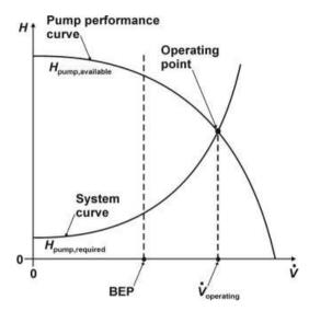
Figure 3.9 Schematic of a system curve intersecting a pump performance curve
