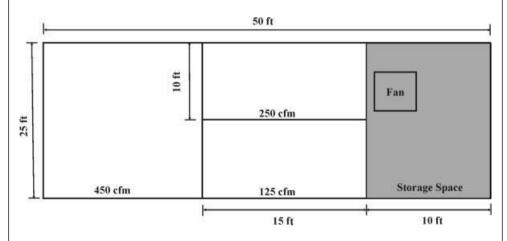
A new Greenheck fan will be located on top of the roof, and the new duct system will be connected to this fan. The roof is 3 ft above the dropped ceiling. The wall partitions shown in the sketch do not extend beyond the dropped ceiling. Layout an appropriate rectangular duct system to deliver the air to the private rooms.
