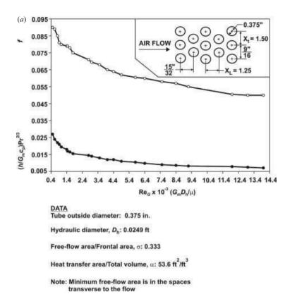
**Figure C.2** *j*-factor versus  $Re_G$  charts for staggered tube banks. Transient tests (6 charts): (a) For  $X_t = 1.50$  and  $X_L = 1.25$ ; (b) For  $X_t = 1.25$  and  $X_L = 1.25$ ; (c) For  $X_t = 1.50$  and  $X_L = 1.0$ ; (d) For  $X_t = 1.5$  and  $X_L = 1.5$ ; (e) For  $X_t = 2$  and  $X_L = 1$ ; (f) For  $X_t = 2.5$  and  $X_L = 0.75$ .
