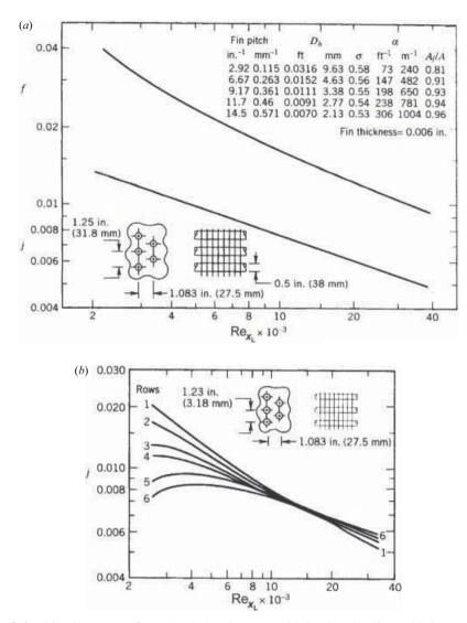
**Figure C.3** *j*-factor versus  $\text{Re}_{x_L}$  charts for staggered tube banks (finned tubes): (a) five rows of tubes (*ASHRAE Transactions*, vol. 79, Part II, 1973; reprinted with permission); (b) multiple rows of tubes (*ASHRAE Transactions*, vol. 81, Part I, 1975; reprinted with permission)
