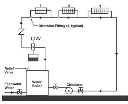
Figure 5.12 Schematic of a one-pipe "monoflow" series loop system
