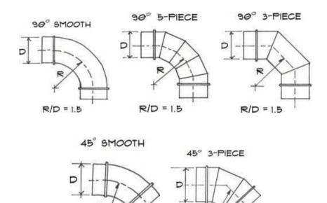
R/D = 1.5 Figure A.2 Schematics elbows in ducts
