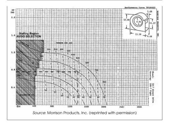
The details of the fan housing and wheel are provided with the curves. The fan speed must be **1100 rpm**. It is important to note that the operating point falls within the recommended region of operation shown in Figure 2.7. Operating points that fall below 570 cfm (30% of free delivery) or above 1520 cfm (80% of free delivery) should not be matched with this fan operating at 1100 rpm.
