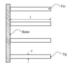
Figure 4.20 General constant area, straight fins attached to a surface
