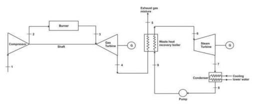
Figure 6.15 Schematic of a combined-cycle power plant
