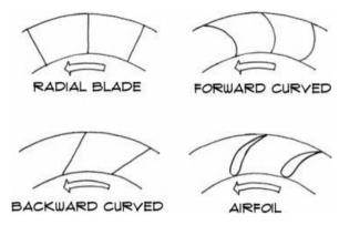
Figure 2.6 Classification of centrifugal fans based on blade types
