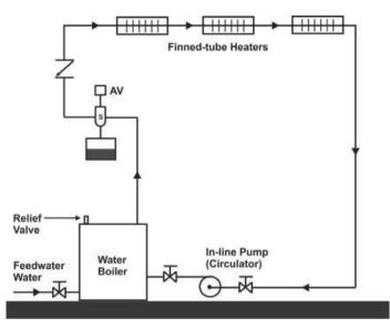
Figure 5.5 Schematic of a closed-loop hydronic heating system complete with a boiler
