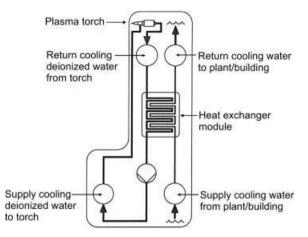
**Figure 5.4** Flow diagram for cooling a typical plasma torch (modified from Sulzer Metco, Product Manual MAN 41292 EN 05; reprinted with permission)
