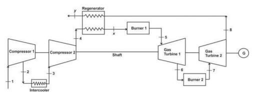
Figure 6.14 Regenerative Brayton cycle with intercooling
