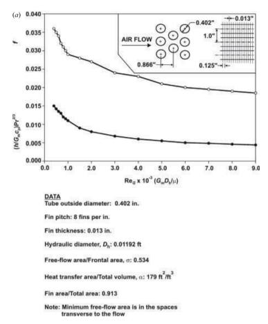
**Figure C.4** *j*-factor versus  $\text{Re}_{G}$  charts for staggered tube banks (finned tubes). (a) Tube outer diameter = 0.402 in.; (b) tube outer diameter = 0.676 in. (Kays, W. and London, A. (1964) *Compact Heat Exchangers,* 2nd edn, McGraw-Hill, Inc., New York)
