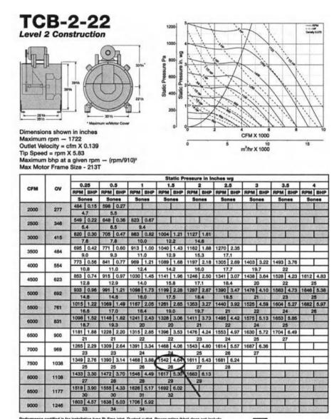
Performance certified is for installation type B: Previnet, Ducted outlet. Power rating (bhg) does not include transmission losses. Performance ratings do not include the effects of appurtenances (accessories) in the ainstream. The sound ratings shown are for installation type B: free inite fan sone ievels.
