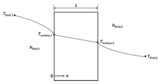
Figure 4.5 Temperature distribution around and through a 1D plane wall
