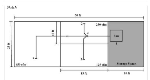
This sketch will be used to provide *estimates* of the duct lengths, and will serve as justification of these estimates. All the fittings are shown (except bellmouth at the entrance to the duct system). All attempts were made to center the ductwork in the rooms to promote uniform distribution of air in the spaces.
