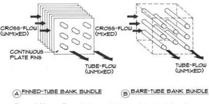
Figure 4.13 (a) Finned tube and (b) bare tube bank bundles
