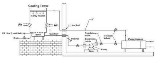
Figure 3.12 A typical open-loop condenser piping system for water
