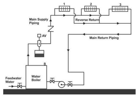
Figure 5.15 Schematic of a two-pipe reverse return system
