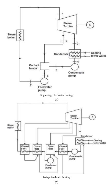
**Figure 6.3** Ideal regenerative Rankine cycles. (a) Single-stage feedwater heating; (b) four-stage feedwater heating
