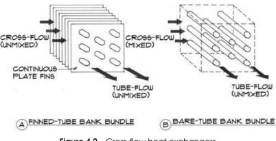
Figure 4.2 Cross-flow heat exchangers
