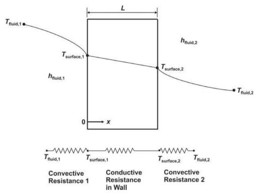
Figure 4.6 Thermal resistance network around a plane wall
