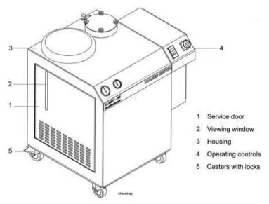
**Figure 5.2** The Sulzer Metco Climet-HE<sup>™</sup>-200 heat exchanger (Sulzer Metco, Product Manual MAN 41292 EN 05; reprinted with permission)
