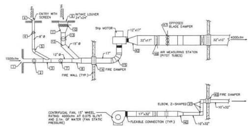
**Figure 2.3** A ductwork system to transport air (*ASHRAE Handbook*, Fundamentals Volume, 2005; reprinted with permission)
