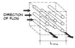
Figure 4.18 Schematic drawing of tube bank showing the total length, Ltotal
