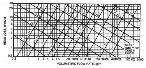
**Figure 3.3** Plastic pipe (Schedule 80) friction loss chart (*ASHRAE Handbook*, Fundamentals Volume, 2005; reprinted with permission)
