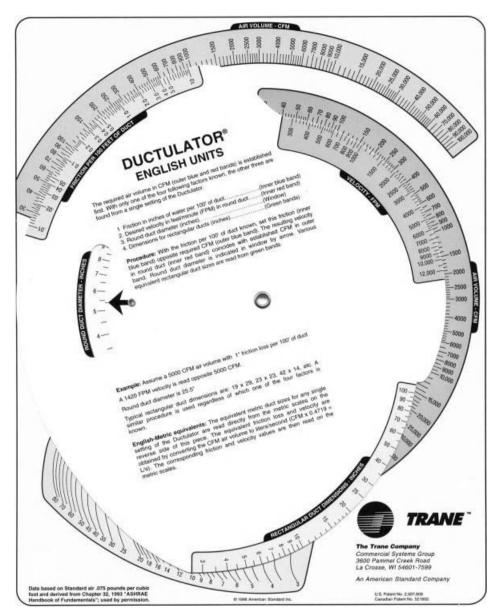
Figure 2.2 Photo of a typical air duct calculator
