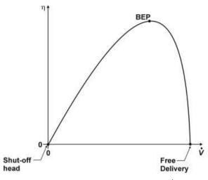
**Figure 3.8** Schematic of a  $\eta_{\text{pump}}$  versus  $\dot{V}$  curve
