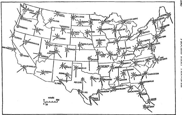
FIG. 17.6. Summer wind data. The length of each line indicates the number of hours in a normal July that the wind blows toward the center circles at each of 71 stations. Figures in circles are average July velocities in miles per hour. (The Marley Company.)
