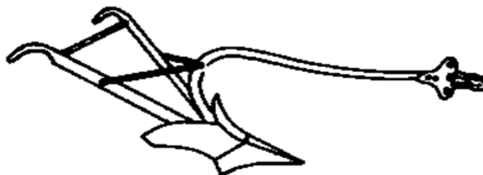
Figure.3: Ridger plough: (c) hand-drawn version
