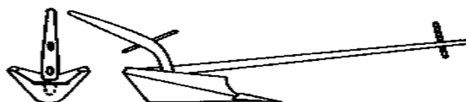
Figure.1: Ridger plough: (a) wooden body, animal-drawn
