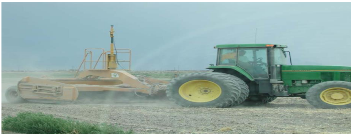
Fig.5. Laser Guided Land Leveling Equipment positioning in irrigation area.
