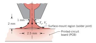
For your study, consider a round nozzle with a diameter of 1 mm located a distance of 2 mm from the region of the surface mount, which has a diameter of 2.5 mm.
