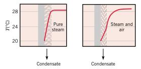
For the air–steam mixture, determine the partial pressure of air as a function of distance from the condensate film.
