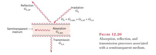
reflected, absorbed, and transmitted. From a radiation balance on the medium, it follows that
