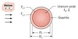
Consider steady-state conditions for which radiation effects may be neglected, the gas velocity and temperature are V=20 m/s and  $T_{\infty}=500$  K, the pellet and shell diameters are  $D_i=10$  mm and  $D_o=12$  mm, and the shell surface temperature is  $T_{s,o}=1300$  K. The uranium oxide and graphite each have a thermal conductivity of  $k_p=k_g=2$  W/m·K.
