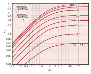
FIGURE 13.4 View factor for aligned parallel rectangles.
