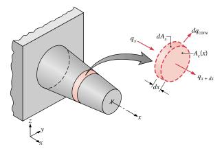
**FIGURE 3.15** Energy balance for an extended surface.
