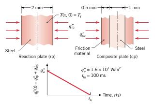
(a) On T-t coordinates, sketch the temperature history at the midplane of the reaction plate, at the interface between the clutch pair, and at the midplane of the composite plate. Identify key features.
