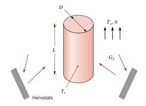
(a) Consider representative operating conditions for which solar irradiation at  $G_S = 80,000 \text{ W/m}^2$  is
