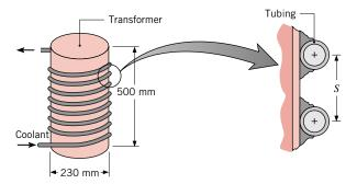
Assuming the maximum allowable temperature rise of the coolant to be  $6^{\circ}$ C, determine the required coolant flow rate, the total length of tubing, and the coil pitch S between turns of the tubing.
