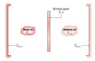
If the glass has an emissivity of  $\varepsilon = 1$ , what is its temperature T? What is the rate of heat loss through the glass?
