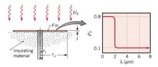
Heat is conducted to the fin through a solid rod of radius  $r_i$ , and the exposed upper surface of the fin radiates to free space, which is essentially at absolute zero temperature.
