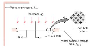
Assuming one-dimensional conduction and using a finite-difference method representing the grid by ten nodes in the x direction, estimate the temperature distribution for the grid. *Hint:* For each node requiring an energy balance, use the linearized form of the radiation rate equation, Equation 1.8, with the radiation coefficient  $h_x$ , Equation 1.9, evaluated for each node.
