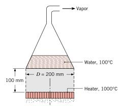
(a) By what factor could the vapor production rate be increased if the cylindrical sides (dashed surface) were insulated rather than open to the surroundings maintained at 27°C?
