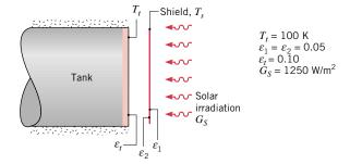
Find the temperature of the shield  $T_s$  and the heat flux  $(W/m^2)$  to the end of the tank.
