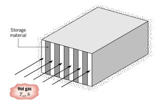
Each layer of the storage material is an aluminum slab of width W=0.05 m, which is at an initial temperature of 25°C. Consider conditions for which the storage unit is charged by passing a hot gas through the passages, with the gas temperature and the convection coefficient assumed to have constant values of  $T_{\infty}=600$ °C and  $h=100 \text{ W/m}^2 \cdot \text{K}$  throughout the channel. How long will it take to achieve 75% of the maximum possible
