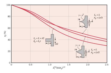
FIGURE 3.18 Efficiency of straight fins (rectangular, triangular, and parabolic profiles).
