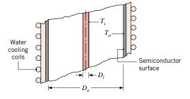
Assuming diffuse, gray surfaces, determine the heat transfer rate per unit area of the outer cylinder. The electrical output of the semiconductor surface is 10% of the absorbed irradiation in the wavelength region 0.6 to 2.0  $\mu$ m. For the prescribed conditions,
