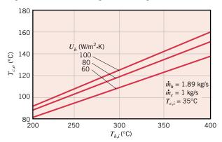
If the intent is to maintain a fixed water outlet temperature of  $T_{c,o} = 125$ °C, adjustments in the flow rates,  $\dot{m}_c$  and  $\dot{m}_h$ , could be made to compensate for the variations. The model equations could be used to determine the adjustments and hence as a basis for designing the requisite *controller*.
