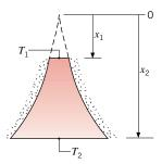
The sides are well insulated, while the top surface of the cone at  $x_1$  is maintained at  $T_1$  and the bottom surface at  $x_2$  is maintained at  $T_2$ .
