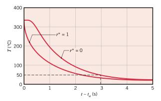
**3.** The *IHT Models, Transient Conduction, Sphere* option could be used to analyze the cooling processes experienced by the sphere in air and water, steps 1 and 2. The *IHT Models, Lumped Capacitance* option may only be used to analyze the air-cooling process, step 1.
