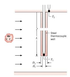
for steel, k = 35 W/m·K, and, for air,  $\rho = 0.774$  kg/m³,  $\mu = 251 \times 10^{-7}$  N·s/m², k = 0.0373 W/m·K, and Pr = 0.686.
