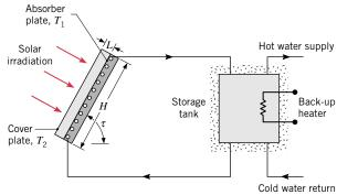
Although much of the solar energy collected by the absorber plate is transferred to a working fluid passing through a coiled tube brazed to the back of the absorber, some of the energy is lost by free convection and net radiation transfer across the air gap. In Chapter 13, we will evaluate the contribution of radiation exchange to this loss. For now, we restrict our attention to the free convection effect.
