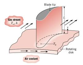
The blades, which are fabricated from Inconel,  $k \approx 20$  W/m·K, have a length of L=50 mm. The blade profile has a uniform cross-sectional area of  $A_c=6\times 10^{-4}$  m² and a perimeter of P=110 mm. A proposed blade-cooling scheme, which involves routing air through the supporting disc, is able to maintain the base of each blade at a temperature of  $T_b=300^{\circ}\mathrm{C}$ .
