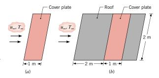
(a) What is the rate of convective heat loss from the plate?
