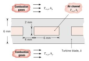
Under operating conditions for which  $h_o = 1000 \text{ W/m}^2 \cdot \text{K}$ ,  $T_{\infty,o} = 1700 \text{ K}$ ,  $h_i = 200 \text{ W/m}^2 \cdot \text{K}$ , and  $T_{\infty,i} = 400 \text{ K}$ , determine the temperature field in the turbine blade and the rate of heat transfer per unit length to the channel. At what location is the temperature a maximum?
