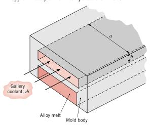
To minimize corrosion damage to the expensive mold, it is customary to use a heat transfer fluid such as ethylene glycol, rather than process water. Compare the convection coefficients of water and ethylene glycol for this application. What is the trade-off between thermal performance and minimizing corrosion?
