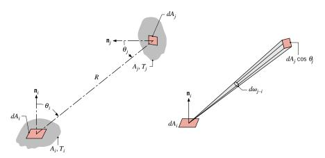
**FIGURE 13.1** View factor associated with radiation exchange between elemental surfaces of area  $dA_i$  and  $dA_j$ .
