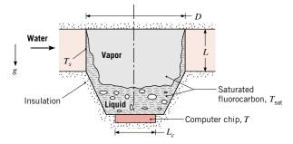
The nucleate boiling constants and the properties of the fluorocarbon are provided in Problem 10.23. In addition,  $k_l = 0.054 \text{ W/m} \cdot \text{K}$ .
