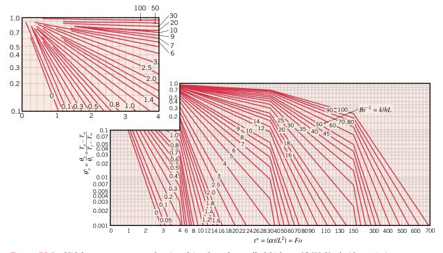
**FIGURE 58.1** Midplane temperature as a function of time for a plane wall of thickness 2*L*[1]. Used with permission.
