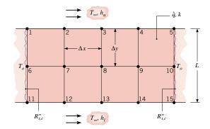
Consider steady-state conditions for which heat is uniformly generated at a volumetric rate  $\dot{q}$  due to passage of an electric current. Using the energy balance method, derive finite-difference equations for nodes 1 and 13.
