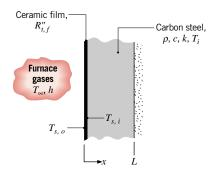
At furnace start-up the wall is at an initial temperature of  $T_i = 300$  K, and combustion gases at  $T_\infty = 1300$  K enter the furnace, providing a convection coefficient of h = 25 W/m<sup>2</sup>·K at the ceramic film. Assuming the film to have negligible thermal capacitance, how long will it take for the inner surface of the steel to achieve a temperature of  $T_{s,i} = 1200$  K? What is the temperature  $T_{s,o}$  of the exposed surface of the ceramic film at this time?
