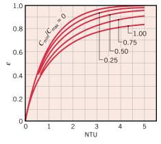
**FIGURE 11.11** Effectiveness of a counterflow heat exchanger (Equation 11.29).
