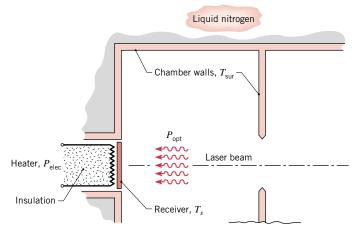
Consider a radiometer with a 15-mm-diameter receiver having a blackened surface with an emissivity of 0.95 and an absorptivity of 0.98 for the optical beam. When operating in the optical mode, conduction heat losses from the backside of the receiver are negligible. In the electrical mode, the loss amounts to 5% of the electrical power. What is the optical power of a beam when the indicated electrical power is 20.64 mW? What is the corresponding receiver temperature?
