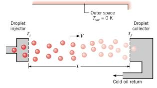
Consider conditions for which droplets of emissivity  $\varepsilon=0.95$  and diameter D=0.5 mm are injected at a temperature of  $T_i=500$  K and a velocity of V=0.1 m/s. Properties of the oil are  $\rho=885$  kg/m³, c=1900 J/kg·K, and k=0.145 W/m·K. Assuming each drop to radiate to deep space at  $T_{\rm sur}=0$  K, determine the distance L required for the droplets to impact the collector at a final temperature of  $T_f=300$  K. What is the amount of thermal energy rejected by each droplet?
