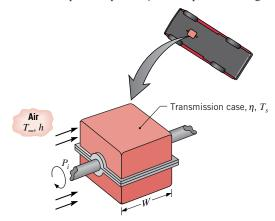
If the transmission efficiency is  $\eta=0.93$  and air flow over the case corresponds to  $T_{\infty}=30^{\circ}\mathrm{C}$  and  $h=200~\mathrm{W/m^2} \cdot \mathrm{K}$ , what is the surface temperature of the transmission?
