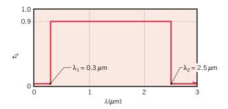
What is the total transmissivity of the cover glass to solar radiation?
