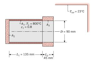
Determine the power required to maintain the furnace operating conditions with the surroundings at 23°C.
