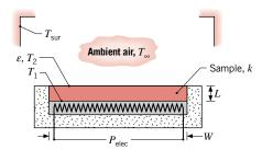
Consider a sample of thickness L = 25 mm and a square planform of width W = 250 mm. In an experi-
