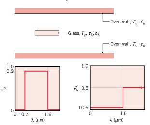
12.71 A horizontal semitransparent plate is uniformly irradiated from above and below, while air at  $T_{\infty} = 300 \text{ K}$  flows over the top and bottom surfaces, providing a uniform convection heat transfer coefficient of
