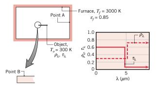
For the specified points on the furnace wall (A) and the object (B), indicate values for  $\varepsilon$ ,  $\alpha$ , E, G, and J.
