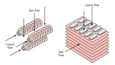
**FIGURE 3.13** Schematic of typical finned-tube heat exchangers.
