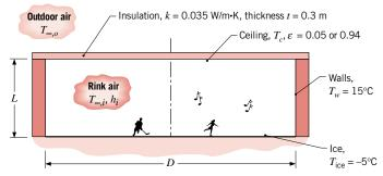
The rink has a diameter of D=50 m and a height of L=10 m, and the temperatures of the ice and walls are  $-5^{\circ}$ C and 15°C, respectively. The rink air temperature is 15°C, and a convection coefficient of  $5 \text{ W/m}^2 \cdot \text{K}$  characterizes conditions on the ceiling surface. The thickness and thermal conductivity of the ceiling insu-
