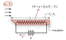
FIGURE 7.1 Experiment for measuring the average convection heat transfer coefficient  $\bar{h}_L$ .
