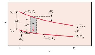
**FIGURE 11.8** Temperature distributions for a counterflow heat exchanger.
