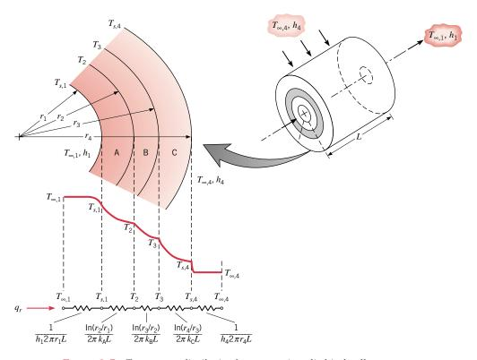
**FIGURE 3.7** Temperature distribution for a composite cylindrical wall.
