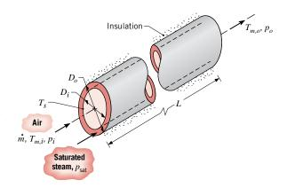
Consider conditions for which air enters a 50-mm-diameter tube at a pressure of 5 atm, a temperature of  $T_{m,i} = 17^{\circ}\text{C}$ , and a flow rate of  $\dot{m} = 0.03 \text{ kg/s}$ , while saturated steam at 2.455 bars condenses on the outer surface of the tube. If the length of the annulus is L = 5 m, what are the outlet temperature  $T_{m,o}$  and pressure  $p_o$  of the air? What is the mass rate at which condensate leaves the annulus?
