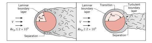
**FIGURE 7.7** The effect of turbulence on separation.
