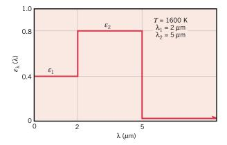
Determine the total, hemispherical emissivity and the total emissive power. At what wavelength will the spectral emissive power be a maximum?
