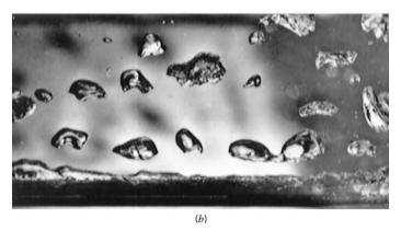
FIGURE 10.5 Boiling of methanol on a horizontal tube.
