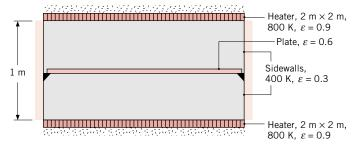
The heaters and the plate are 2 m by 2 m on a side, and each heater is separated from the plate by a distance of 0.5 m. Each heater is well insulated on its back side and has an emissivity of 0.9 at its exposed surface. The plate and the sidewalls have emissivities of 0.6 and 0.3, respectively. Sketch the equivalent radiation network for the system and label all pertinent resistances and potentials. For the prescribed conditions, obtain the required electrical power and the plate temperature.
