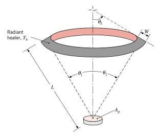
For  $\theta_1 = 30^\circ$ ,  $\theta_2 = 60^\circ$ , L = 3 m, and W = 30 mm, what is the rate at which radiant energy emitted by the heater is incident on the part?
