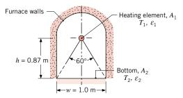
Neglecting convection and treating the furnace walls as isothermal, determine the power per unit length that must be provided to the heating element to maintain steady-state conditions. Calculate the temperature of the furnace wall.
