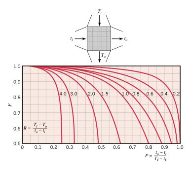
**FIGURE 11S.3** Correction factor for a single-pass, cross-flow heat exchanger with both fluids unmixed.
