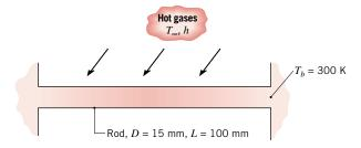
(a) Using an appropriate numerical technique, determine the thermal response of the rod to the convective heating. Plot the midspan temperature as a function of elapsed time. Using an appropriate analytical model of the rod, determine the steady-state temperature distribution and compare the result with that obtained numerically for very long elapsed times.
