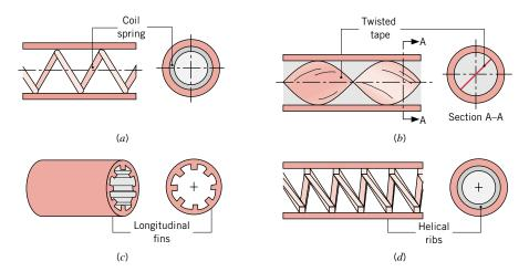
**FIGURE 8.12** Internal flow heat transfer enhancement schemes: (a) longitudinal section and end view of coil-spring wire insert, (b) longitudinal section and cross-sectional view of twisted tape insert, (c) cut-away section and end view of longitudinal fins, and (d) longitudinal section and end view of helical ribs.
