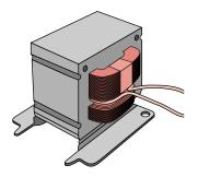
The external transformer geometry is approximately cubical, with a length of 32 mm to a side. The combined
