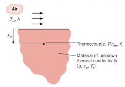
If the convection coefficient associated with the air flow is  $h = 200 \text{ W/m}^2 \cdot \text{K}$  and a temperature of 60°C is recorded 5 min after the onset of cooling, what is the thermal conductivity of the material?
