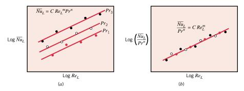
**FIGURE 7.2** Dimensionless representation of convection heat transfer measurements.
