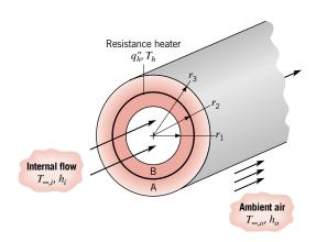
Liquid pumped through the tube is at a temperature  $T_{\infty,i}$  and provides a convection coefficient  $h_i$  at the inner surface of the composite. The outer surface is exposed to ambient air, which is at  $T_{\infty,o}$  and provides a convection coefficient of  $h_o$ . Under steady-state conditions, a uniform heat flux of  $q_n^n$  is dissipated by the heater.
