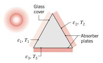
During operation the surface temperatures are known to be  $T_1 = 25$ °C,  $T_2 = 60$ °C, and  $T_3 = 70$ °C. What is the net rate at which radiation is transferred to the cover due to exchange with the absorber plates?
