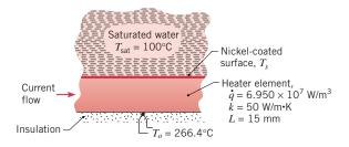
(a) From the foregoing data, calculate the surface temperature,  $T_s$ , and the heat flux at the exposed surface.
