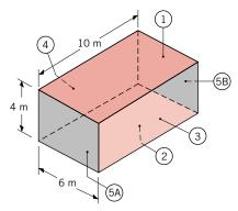
Assuming the surfaces are diffuse and gray, find the net radiation heat transfer from each surface.
