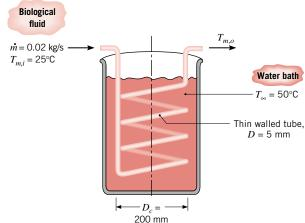
corresponding variation of the exit temperature of the biological fluid could influence the downstream process. What variation would you expect in  $T_{m,o}$  for a  $\pm 10\%$  change in  $\dot{m}$ ?
