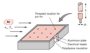
Measured temperatures for five pin-fin configurations are tabulated.
