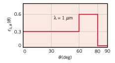
Determine corresponding values of the spectral, normal emissivity; the spectral, hemispherical emissivity; the spectral intensity of radiation emitted in the normal direction; and the spectral emissive power.
