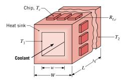
If N = 120 chips attached to the outer surfaces of the heat sink maintain an approximately uniform surface temperature of  $T_2 = 50$ °C and all of the heat dissipated by the chips is assumed to be transferred to the coolant, what is the heat dissipation per chip? If the contact resistance between each chip and the heat sink is  $R_{t,c} = 0.2$  K/W, what is the chip temperature?
