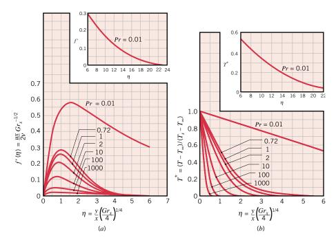
**FIGURE 9.4** Laminar, free convection boundary layer conditions on an isothermal, vertical surface. (a) Velocity profiles. (b) Temperature profiles [3].
