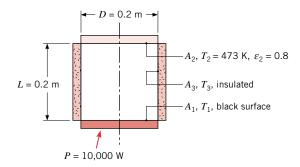
Determine the operating temperature of the lower plate  $T_1$  and the temperature of the insulated side  $T_3$ .
