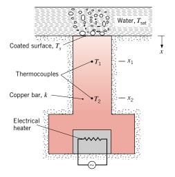
(a) An experiment is performed to determine the boiling characteristics of a special coating applied to the exposed surface. Under steady-state conditions, nucleate boiling is maintained in saturated water at
