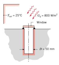
12.108 Consider the evacuated tube solar collector described in part (d) of Problem 1.73 of Chapter 1. In the interest of maximizing collector efficiency, what spectral radiative characteristics are desired for the outer tube and for the inner tube?
