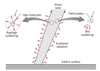
FIGURE 12.29 Scattering of solar radiation in the earth's atmosphere.
