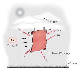
Determine the temperature  $T_s$  of the towel. What is the corresponding evaporation rate for a towel that is 0.75 m wide by 1.50 m long?
