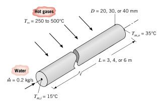
Your assignment is to develop a series of design graphs that can be used to demonstrate acceptable combinations of tube dimensions (D and L) and of hot gas conditions ( $T_{\infty}$  and V) that satisfy this requirement. In your analysis, consider the following parameter ranges: D=20, 30, or 40 mm; L=3, 4, or 6 m;  $T_{\infty}=250$ , 375, or 500°C; and  $20 \le V \le 40$  m/s.
