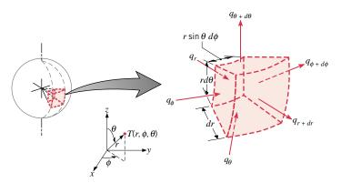
**FIGURE 2.13** Differential control volume,  $dr \cdot r \sin \theta \, d\phi \cdot r \, d\theta$ , for conduction analysis in spherical coordinates  $(r, \phi, \theta)$ .
