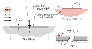
Use the finite-element method of *FEHT* to analyze a symmetrical half-section of the gage and the quartz substrate. Assume that the lower and end surfaces of the substrate are perfectly insulated, while the upper surface experiences convection with the fluid.
