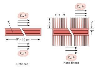
3.134 As more and more components are placed on a single integrated circuit (chip), the amount of heat that is dissipated continues to increase. However, this increase is limited by the maximum allowable chip operating temperature, which is approximately 75°C. To maximize heat dissipation, it is proposed that a 4 × 4 array of copper pin fins be metallurgically joined to the outer surface of a square chip that is 12.7 mm on a side.
