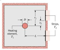
Thermal conditions in the oven are maintained by a long silicon carbide rod (heating element), which is of diameter D=20 mm and is operated at  $T_1=1700$  K. Each of two strips on one side wall has the same orientation relative to the rod ( $s_1=60$  mm,  $s_2=20$  mm,  $s_2=20$  mm) and is operated at  $s_2=600$  K. All surfaces are
