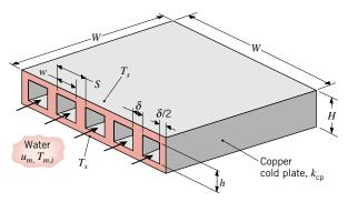
Consider conditions for which *equivalent* heat-generating systems are attached to the top and bottom of the cold plate, maintaining the corresponding surfaces at the same temperature  $T_s$ . The mean velocity and inlet temperature of the coolant are  $u_m$  and  $T_{m,i}$ , respectively.
