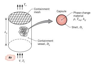
Consider an application for which air is chilled by passing it through a packed bed ( $\varepsilon = 0.5$ ) of capsules ( $D_c = 50$  mm) containing an organic compound with a melting point of  $T_{\rm mp} = 4^{\circ}{\rm C}$ . The air enters a cylindrical vessel ( $L_v = D_v = 0.40$  m) at  $T_i = 25^{\circ}{\rm C}$  and V = 1.0 m/s.
