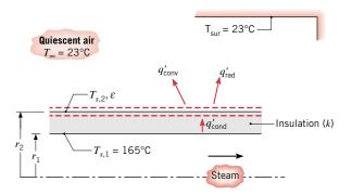
Free convection heat transfer to the ambient air and net radiation transfer to the surroundings depend on the temperature  $T_{s,2}$  of the insulation, which may be obtained by performing an energy balance at the outer surface:
