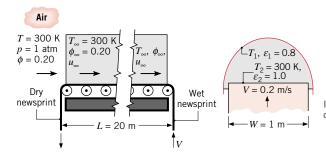
Since the velocity of the air is large, its temperature and relative humidity can be assumed to be constant over the entire duct length. Calculate the required evaporation rate, air velocity  $u_{\infty}$ , and temperature  $T_1$  that will ensure steady-state conditions for the process.
