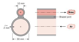
11.29 A twin-tube, counterflow heat exchanger operates with balanced flow rates of 0.003 kg/s for the hot and cold airstreams. The cold stream enters at 280 K and must be heated to 340 K using hot air at 360 K. The average pressure of the airstreams is 1 atm and the maximum allowable pressure drop for the cold air is 10 kPa. The tube walls may be assumed to act as fins, each with an efficiency of 100%.
