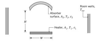
The heater is at  $T_1 = 1000$  K and has an emissivity of  $\varepsilon_1 = 0.9$ , while the absorber is at  $T_2 = 600$  K and has an emissivity of  $\varepsilon_2 = 0.5$ . The system is in a large room whose walls are at 300 K. What is the net rate of heat transfer to the absorber surface?
