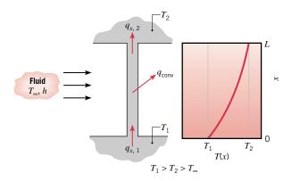
**FIGURE 3.11** Combined conduction and convection in a structural element.
