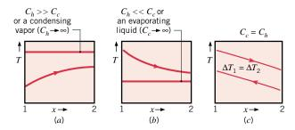
**FIGURE 11.9** Special heat exchanger conditions. (a)  $C_h \gg C_c$  or a condensing vapor. (b) An evaporating liquid or  $C_h \ll C_c$ . (c) A counterflow heat exchanger with equivalent fluid heat capacities  $(C_h = C_c)$ .
