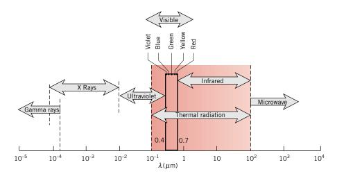
FIGURE 12.3 Spectrum of electromagnetic radiation.
