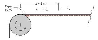
To maintain a uniform strip temperature, the irradiation G must be varied with x along the strip. For  $0 \le x \le 1$  m, compute and plot the variations  $h_{m,x}(x)$ ,  $N_A''(x)$ , and G(x).
