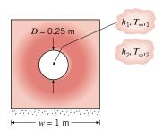
**4.24** In Chapter 3 we assumed that, whenever fins are attached to a base material, the base temperature is unchanged. What in fact happens is that, if the temperature of the base material exceeds the fluid temperature, attachment of a fin depresses the junction temperature  $T_j$  below the original temperature of the base, and heat flow from the base material to the fin is two-dimensional.
