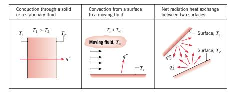
**FIGURE 1.1** Conduction, convection, and radiation heat transfer modes.
