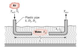
If air from the home enters the pipe at a temperature of  $T_{m,i} = 29^{\circ}\text{C}$  and a volumetric flow rate of  $V_i = 0.025 \text{ m}^3/\text{s}$ , what pipe length L is needed to provide a discharge temperature of  $T_{m,o} = 21^{\circ}\text{C}$ ? What is the fan power required to move the air through this length of pipe if its inner surface is smooth?
