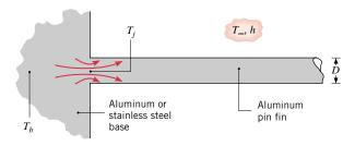
Consider conditions for which a long aluminum pin fin of diameter D=5 mm is attached to a base material whose temperature far from the junction is maintained at  $T_b=100^{\circ}\text{C}$ . Fin convection conditions correspond to  $h=50 \text{ W/m}^2 \cdot \text{K}$  and  $T_{\infty}=25^{\circ}\text{C}$ .
