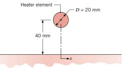
(a) Assuming both the element and the wall are black, estimate the maximum temperature reached by the wall when the surroundings are at 300 K. Problems 857
