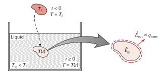
**FIGURE 5.1** Cooling of a hot metal forging.
