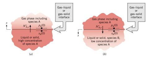
**FIGURE 14.6** Species concentration at a gas—liquid or gas—solid interface. (a) Evaporation or sublimation of species A from a liquid or solid into a gas. (b) Transfer of weakly soluble species A from the gas to a liquid or solid.
