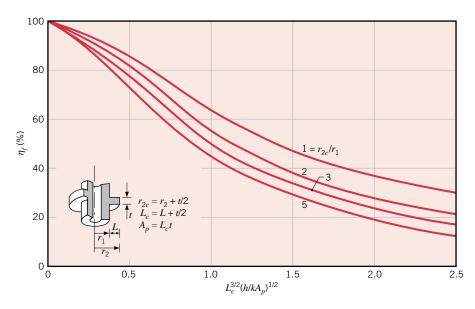
FIGURE 3.19 Efficiency of annular fins of rectangular profile.
