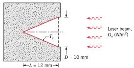
A fine-wire thermocouple attached to the surface indicates a temperature rise of 10.1°C when a laser beam is incident upon the meter. What is the optical (radiant) flux of the laser beam,  $G_a$  (W/m<sup>2</sup>)?
