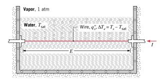
**FIGURE 10.2** Nukiyama's power-controlled heating apparatus for demonstrating the boiling curve.
