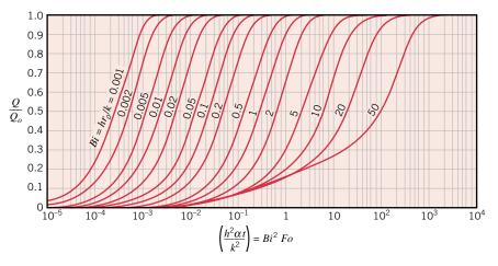
**FIGURE 58.9** Internal energy change as a function of time for a sphere of radius  $r_o$  [2]. Adapted with permission.
