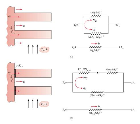
**FIGURE 3.21** Fin array and thermal circuit. (a) Fins that are integral with the base. (b) Fins that are attached to the base.
