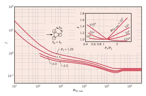
**FIGURE 7.14** Friction factor f and correction factor  $\chi$  for Equation 7.69. Staggered tube bundle arrangement [15]. Used with permission.
