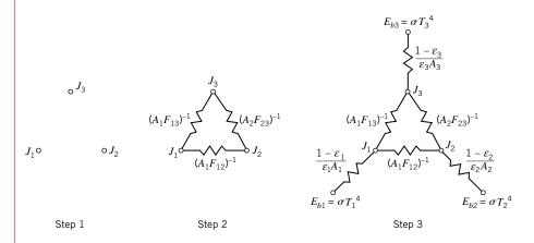
In this problem, the surface resistance associated with surface 3 is zero according to assumption 4; therefore,  $J_3 = E_{b3} = \sigma T_3^4 = 459 \text{ W/m}^2$ .
