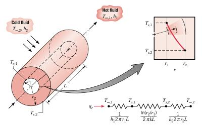
**FIGURE 3.6** Hollow cylinder with convective surface conditions.
