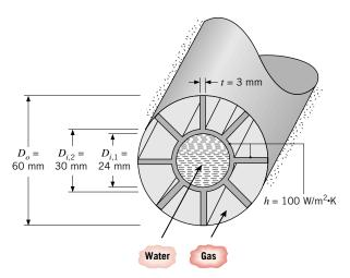
region to pressurized water flowing through the inner tube of the annulus. The inner tube has inner and outer diameters of 24 and 30 mm and is connected by eight struts to an insulated outer tube of 60-mm diameter. Each strut is 3 mm thick and is integrally fabricated with the inner tube from carbon steel ( $k = 50 \text{ W/m} \cdot \text{K}$ ).
