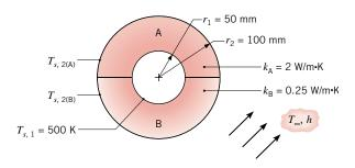
The interface between the two materials may be assumed to have an infinite contact resistance, and the entire outer surface is exposed to air for which  $T_{\infty} = 300 \text{ K}$  and  $h = 25 \text{ W/m}^2 \cdot \text{K}$ .
