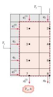
For the one-half symmetrical section shown schematically above, it follows that conduction into the nodal regions must be balanced by convection from the regions. Hence
