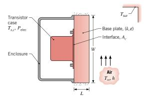
(a) If the air-filled aluminum-to-aluminum interface is characterized by an area of  $A_c = 2 \times 10^{-4} \,\mathrm{m}^2$  and a roughness of 10  $\mu\mathrm{m}$ , what is the maximum allowable power dissipation if the surface temperature of the case,  $T_{s,c}$ , is not to exceed 85°C?
