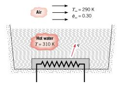
If the tub is well insulated on its sides and bottom and the temperature of the makeup water is equal to that of the tub water, at what rate must electrical heaters supply energy to maintain the tub water at 310 K?
