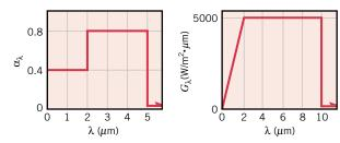
What is the total absorptivity of the surface for the prescribed irradiation? If the surface is at a temperature of 1250 K, what is its emissive power? How will the surface temperature vary with time, for the prescribed conditions?
