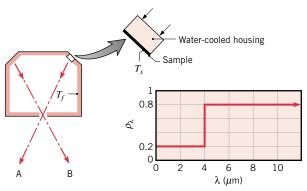
**12.90** A very small sample of an opaque surface is initially at 1200 K and has the spectral, hemispherical absorptivity shown.
