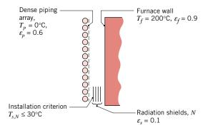
If the temperature of the shield closest to the piping  $T_{s,N}$  must be less than 30°C, how many radiation shields, N, must be installed between the piping and the furnace wall?
