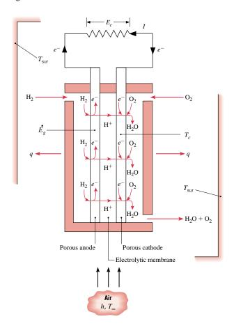
The membrane must operate in a moist state in order to conduct ions. However, the presence of liquid water in the cathode material may block the oxygen from reaching the cathode reaction sites, resulting in failure of the fuel cell. Therefore, it is critical to control the temperature of the fuel cell,  $T_c$ , so that the cathode side contains saturated water vapor.
