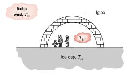
(a) Assuming that the occupants' body heat provides a continuous source of 320 W within the igloo, calculate the inside air temperature when the outside air temperature is  $T_{\infty} = -40^{\circ}$ C. Be sure to consider heat losses through the floor of the igloo.
