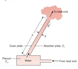
plate at a temperature  $T_s = 67^{\circ}\text{C}$ , while water returned to the reservoir from the heat sink is at  $T_{\infty} = 27^{\circ}\text{C}$ . The system operates as a *thermosyphon*, for which water flow is driven exclusively by buoyancy forces. The plate spacing and length are S = 15 mm and L = 1.5 m.
