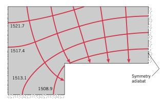
As expected, the maximum temperature exists at the location furthest removed from the coolant, which corresponds to node 1. Temperatures along the surface of the turbine blade exposed to the combustion gases are of particular interest, and using an interpolation scheme with the finite-difference predictions, the following distribution is obtained:
