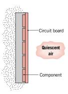
Assuming a uniform surface heat flux, what is the maximum temperature of the board? What is the temperature of the board for an isothermal surface condition?
