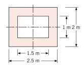
**4S.2** A hot pipe is embedded eccentrically as shown in a material of thermal conductivity 0.5 W/m·K. Using the flux plot method, determine the shape factor and the heat transfer per unit length when the pipe and outer surface temperatures are 150 and 35°C, respectively.
