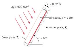
Consider conditions for which the incident solar radiation is collimated at an angle of  $60^{\circ}$  relative to the horizontal and the solar flux is  $900 \text{ W/m}^2$ . The cover plate is perfectly transparent to solar radiation ( $\lambda \leq 3 \mu \text{m}$ ) and is opaque to radiation of larger wavelengths. The cover and absorber plates are diffuse surfaces having the spectral absorptivities shown.
