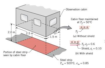
Determine the coolant system heat removal rate required to maintain the cabin floor at 50°C for the following conditions: (a) when the floor, with an emissivity of  $\varepsilon_f = 0.6$ , is directly exposed to the strip;
