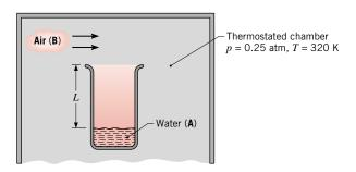
For calibration purposes, you've been asked to calculate the expected evaporation rate  $(kg/h \cdot m^2)$  for a test with water and air under the foregoing conditions, using the known value of  $D_{AB}$  for the vapor–air mixture.
