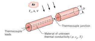
The thermal conductivity is determined by performing an experiment in which the specimen is heated to a uniform temperature of  $T_i = 100^{\circ}\text{C}$  and then cooled by passing air at  $T_{\infty} = 25^{\circ}\text{C}$  in cross flow over the cylinder. For the prescribed air velocity, the convection coefficient is  $h = 55 \text{ W/m}^2 \cdot \text{K}$ .
