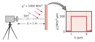
Calculate the total radiant power from a  $10^{-4}$  m<sup>2</sup> area of the surface that reaches a radiation detector positioned along the normal to the area. The aperture of the detector is  $10^{-5}$  m<sup>2</sup>, and its distance from the surface is 1 m.
