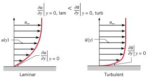
FIGURE 6.7 Comparison of laminar and turbulent velocity boundary layer profiles for the same free stream velocity.<sup>3</sup>
