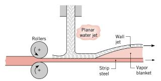
Consider conditions for which the strip steel beneath the vapor blanket is at a temperature of 907 K and has an emissivity of 0.35. Neglecting the effects of the strip and jet motions and assuming boiling within the film to be approximated by that associated with a large horizontal cylinder of 1-m diameter, estimate the rate of heat transfer per unit surface area from the strip to the wall jet.
