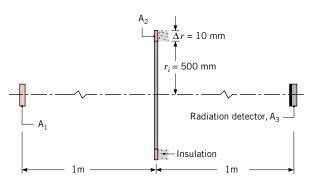
Calculate the rate at which radiation is incident on  $A_3$  due to emission and reflection from  $A_1$ .
