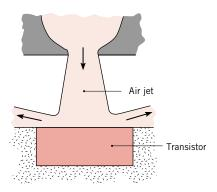
If the transistor is well insulated at all but its exposed surface and the surface temperature is not to exceed 85°C, what is the transistor's maximum allowable operating power?
