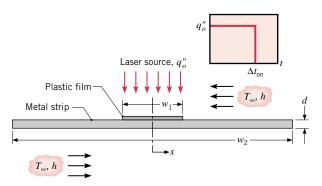
The strip is initially at 25°C and the laser provides a uniform flux of 85,000 W/m² over a time interval of  $\Delta t_{\rm on} = 10$  s. The system dimensions and thermophysical properties remain the same, but the convection coefficient to the ambient air at 25°C is now 100 W/m²·K and  $w_1 = 44$  mm.
