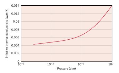
FIGURE 2.10 Measured thermal conductivity of carbon-doped silica aerogel as a function of pressure at  $T \approx 300 \text{ K} [10]$ .
