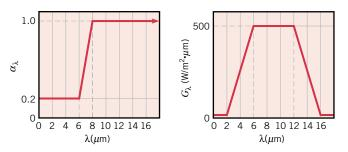
How does the spectral, hemispherical reflectivity vary with wavelength? What is the total, hemispherical absorptivity of the surface? If the surface is initially at 500 K and has a total, hemispherical emissivity of 0.8, how will its temperature change upon exposure to the irradiation?
