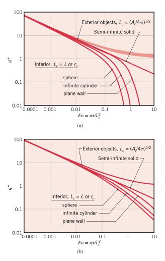
**FIGURE 5.10** Transient dimensionless conduction heat rates for a variety of geometries. (a) Constant surface temperature. Results for the geometries of Table 4.1 lie within the shaded region and are from [5]. (b) Constant surface heat flux.
