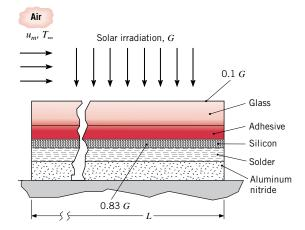
(a) Consider an L=1 m long, w=0.1 m wide solar cell that is placed on an insulated surface. Determine the silicon temperature and the electric power produced by the solar cell for an air velocity of 4 m/s parallel to the long direction, with air and surroundings temperatures of 25°C. The solar irradiation is 700 W/m<sup>2</sup>. The boundary layer is tripped to a turbulent condition at the leading edge of the panel.
