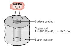
convection coefficient is determined. The following experimental arrangement uses the procedure to determine the convection coefficient for gas flow normal to a surface. Specifically, a long copper rod is encased in a super insulator of very low thermal conductivity, and a very thin coating is applied to its exposed surface.
