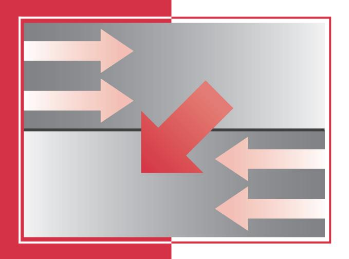
The process of heat exchange between two fluids that are at different temperatures and separated by a solid wall occurs in many engineering applications. The device used to implement this exchange is termed a *heat exchanger*, and specific applications may be found in space heating and air-conditioning, power production, waste heat recovery, and chemical processing.
