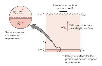
FIGURE 14.7 One-dimensional diffusion with heterogeneous catalysis.
