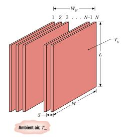
maintained at a fixed temperature  $T_s$  by embedded electrical heaters. The plates are of length and width L=W=300 mm and are in quiescent, atmospheric air at  $T_\infty=20$ °C. The total width of the array cannot exceed a value of  $W_{\rm ar}=150$  mm.
