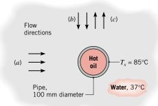
Investigate the effect of flow direction on the heat rate (W/m) for (a) horizontal, (b) downward, and (c) upward flow.
