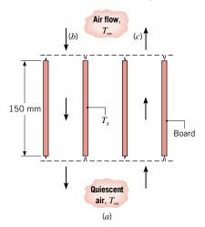
Assuming isothermal surface conditions, determine the allowable electrical power dissipation per board for the cooling arrangements:
