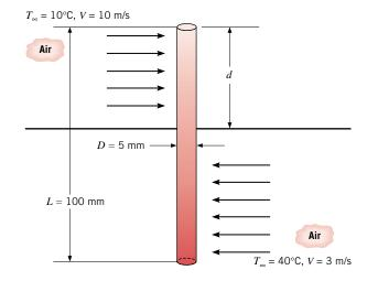
2024 aluminum pin fin through the wall separating the two fluids. The pin is inserted to a depth of d into fluid 1. Fluid 1 is air with a mean temperature of  $10^{\circ}$ C and nearly uniform velocity of 10 m/s. Fluid 2 is air with a mean temperature of  $40^{\circ}$ C and mean velocity of 3 m/s.
