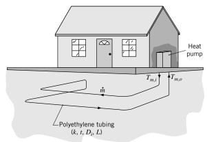
Consider winter conditions for which the liquid is discharged from the heat pump into high-density polyethylene tubing of thickness t = 8 mm and thermal conductivity k = 0.47 W/m·K. The tubing is routed through soil that maintains a uniform temperature of approximately  $10^{\circ}$ C at the tube outer surface. The properties of the fluid may be approximated as those of water.
