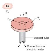
If an embedded electric heater maintains a surface temperature of  $T_s = 50^{\circ}\text{C}$ , what is the local heat flux at the surface of the disk? What is the total electric power requirement? What can you say about the nature of boundary layer development on the disk?
