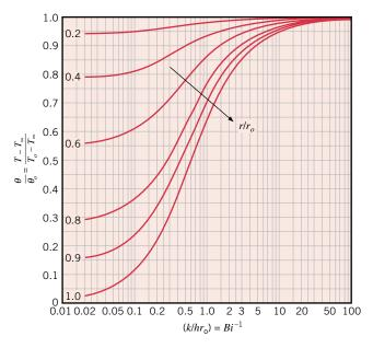
**FIGURE 58.5** Temperature distribution in an infinite cylinder of radius  $r_o$  [1]. Used with permission.
