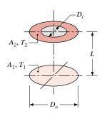
**13.31** A radiometer views a small target (1) that is being heated by a ring-shaped disk heater (2). The target has an area of  $A_1 = 0.0004 \text{ m}^2$ , a temperature of  $T_1 = 500 \text{ K}$ , and a diffuse, gray emissivity of  $\varepsilon_1 = 0.8$ . The heater operates at  $T_2 = 1000 \text{ K}$  and has a black surface. The radiometer views the entire sample area with a solid angle of  $\omega = 0.0008 \text{ sr}$ .
