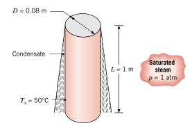
**Assumptions:** The condensate film thickness is small relative to the cylinder diameter.
