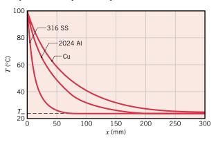
From these distributions, it is evident that there is little additional heat transfer associated with extending the length of the rod much beyond 50, 200, and 300 mm, respectively, for the stainless steel, the aluminum alloy, and the copper.
