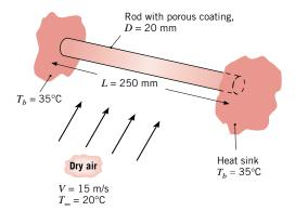
Perform a steady-state, finite-difference analysis of the rod–porous coating system, considering conduction in the rod as well as energy transfer from the surface by convection heat and mass transfer. Use the analysis to estimate the temperature at the midspan of the rod and the evaporation rate from the surface. (Suggestions: Use 10 nodes to represent the half-length of the system.
