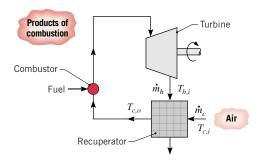
Consider a system for which the recuperator is a cross-flow heat exchanger with both fluids unmixed and the flow rates associated with the turbine exhaust and the air are  $\dot{m}_h = 6.5$  kg/s and  $\dot{m}_c = 6.2$  kg/s, respectively. The corresponding value of the overall heat transfer coefficient is  $U = 100 \text{ W/m}^2 \cdot \text{K}$ .
