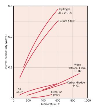
**FIGURE 2.8** The temperature dependence of the thermal conductivity of selected gases at normal pressures. Molecular weights  $(\mathcal{M})$  of the gases are also shown.
