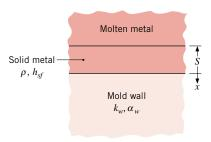
Just before the start of solidification (S=0), the mold wall is everywhere at an initial uniform temperature  $T_i$  and the molten metal is everywhere at its fusion (melting point) temperature of  $T_f$ . Following the start of solidification, there is conduction heat transfer into the mold wall and the thickness of the solidified metal, S, increases with time t.
