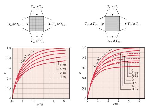
**FIGURE 11.14** Effectiveness of a single-pass, cross-flow heat exchanger with both fluids unmixed (Equation 11.32).
