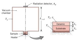
Consider conditions for which a ceramic coating of thickness  $L_c = 0.5$  mm and thermal conductivity  $k_c = 6 \text{ W/m} \cdot \text{K}$  has been sprayed on a metal substrate of thickness  $L_s = 8$  mm and thermal conductivity  $k_s = 25 \text{ W/m} \cdot \text{K}$ . The opaque surface of the ceramic may be approximated as diffuse and gray, with a total, hemispherical emissivity of  $\varepsilon_c = 0.8$ .
