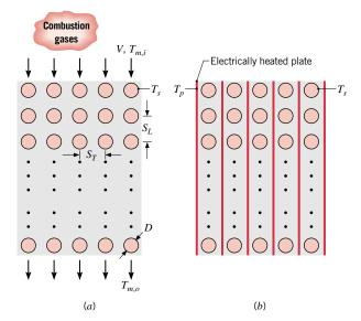
(a) Consider case (a) for which products of combustion *enter* the tube bank with velocity and temperature of V=10 m/s and  $T_{m,i}=1200$  K, respectively. Determine the average gas-side convection coefficient, the gas outlet temperature, and the rate of steam production in kg/s. Properties of the gas may be approximated to be those of atmospheric air at an average temperature of 900 K.
