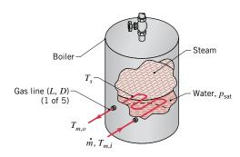
Determine the tube wall temperature  $T_s$  and the gas outlet temperature  $T_{mo}$  for the prescribed conditions. As a first approximation, the properties of the combustion gases may be taken as those of air at 700 K.
