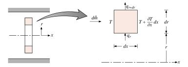
**FIGURE 8.9** Thermal energy balance on a differential element for laminar, fully developed flow in a circular tube.
