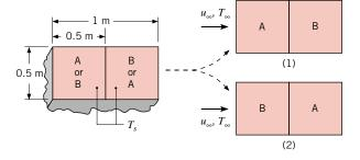
7.22 Consider weather conditions for which the prevailing wind blows past the penthouse tower on a tall building. The tower length in the wind direction is 10 m and there are 10 window panels.
