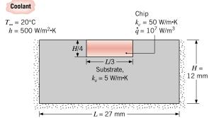
For the conditions shown on the sketch, will the maximum temperature in the chip exceed 85°C, the maximum allowable operating temperature set by industry standards? A grid spacing of 3 mm is suggested.
