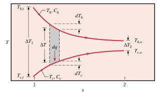
FIGURE 11.7 Temperature distributions for a parallel-flow heat exchanger.
