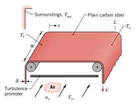
distribution, T(x), along the sheet. Consider the effects of radiation, as well as convection, and express your result in terms of the velocity, thickness, and properties of the sheet  $(V, \delta, \rho, c_p, \varepsilon)$ , the average convection coefficient  $\overline{h}_W$  associated with the cross flow, and the environmental temperatures  $(T_\infty, T_{\text{sur}})$ .
