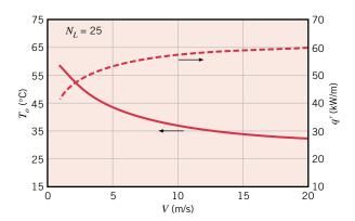
Although the heat rate increases with increasing V, the air outlet temperature decreases, approaching  $T_i$  as  $V \rightarrow \infty$ .
