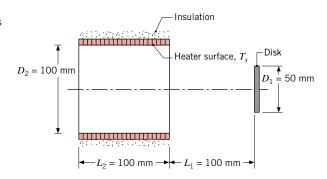
(a) Determine the radiant power from the heater, which is incident on the disk,  $q_{s\rightarrow 1}$ . What is the irradiation on the disk,  $G_1$ ?
