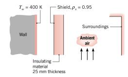
shield reflectivity,  $\rho_s$ , and insulation thermal conductivity, k. What influence do these parameters have on the heat loss from the hot wall? What is the effect of an increased overall coefficient on the heat loss? Show the results of your analysis in a graphical format.
