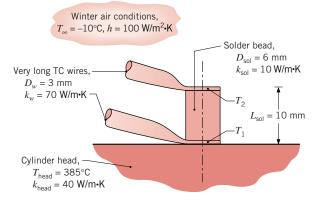
The objective of this problem is to develop a thermal model that can be used to determine the temperature difference  $(T_1 - T_2)$  between the two intermediatemetal TC junctions. Assume that the solder bead does not experience any heat loss from its lateral surface.
