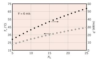
The air outlet temperature would asymptotically approach the surface temperature with increasing  $N_L$ , at which point the heat rate approaches a constant value and there is no advantage to adding more tube rows. Note that  $\Delta p$  increases linearly with increasing  $N_L$ . For  $N_L = 25$  and  $1 \le V \le 20$  m/s, we obtain
