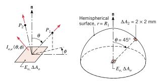
field due to emission into the hemispherical space above the surface is diffuse, thereby providing a uniform intensity  $I(\theta, \phi)$ . Moreover, if the space is a non-participating medium (nonabsorbing, nonscattering, and nonemitting), the intensity is independent of radius for any  $(\theta, \phi)$  direction. Hence intensities at any points  $P_1$  and  $P_2$  would be equal.
