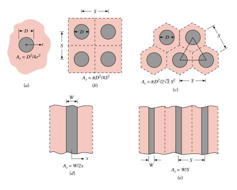
**FIGURE 7.17** Plan view of pertinent geometrical features for (a) single round jet, (b) in-line array of round jets, (c) staggered array of round jets, (d) single slot jet, and (e) array of slot jets.
