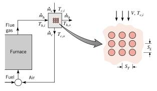
Eighty (80) silicon carbide ceramic tubes (k = 20 W/m·K) of inner and outer diameters equal to 55 and 80 mm, respectively, and of length L = 1.4 m are
