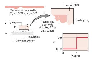
To stabilize the temperature of the pod and prevent overheating of the electronics, the inner surface of the pod is surrounded by a layer of a phase-change material (PCM) having a fusion temperature of 87°C and a heat of fusion of 25 kJ/kg. The pod has an
