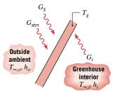
The irradiation comprises the total solar flux  $G_{S}$ , the flux  $G_{\text{atm}}$  due to atmospheric emission (sky radia-
