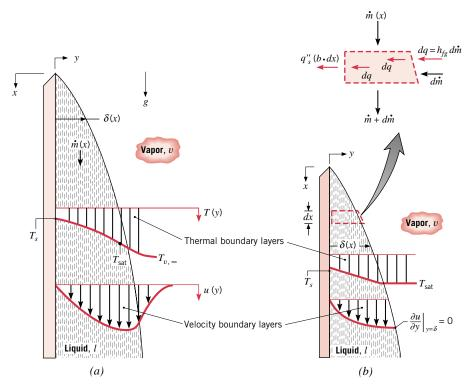
**FIGURE 10.11** Boundary layer effects related to film condensation on a vertical surface. (a) Without approximation. (b) With assumptions associated with Nusselt's analysis, for a vertical plate of width b.
