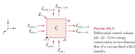
conservation in two-dimensional flow of a viscous fluid with heat transfer.
