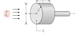
Obtain an expression for the average Nusselt number,  $\overline{Nu}_D = \overline{h}D/k$ , corresponding to heat transfer from an isothermal disk. Typically, boundary layer development from a stagnation point yields a decaying convection coefficient with increasing distance from the stagnation point. Provide a plausible explanation for why the opposite trend is observed for the disk.
