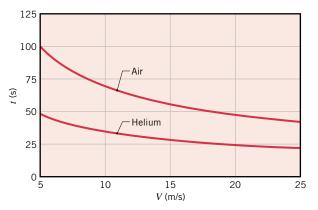
Although Reynolds numbers for He are much smaller than those for air, the thermal conductivity is much larger and, as shown below, convection heat transfer is enhanced.
