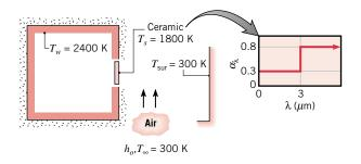
(a) If the temperature of the ceramic plate is not to exceed 1800 K, what is the minimum value of the outside convection coefficient,  $h_o$ , that must be maintained by the air-cooling system?
