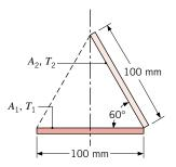
Determine the net radiation exchange between the surfaces per unit length of the surfaces. Consider the configuration when a black surface  $(A_3)$ , whose back side is insulated, is positioned along the dashed line shown. Calculate the net radiation transfer to surface  $A_2$  per unit length of the surface and determine the temperature of the insulated surface  $A_3$ .
