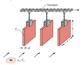
For an initial plate temperature of  $T_i = 300^{\circ}$ C, what is the rate of heat transfer from the plate? What is the corresponding rate of change of the plate temperature? The velocity of the air is much larger than that of the plate.
