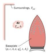
If an approximately uniform heat flux of  $q_h'' = 1.25 \times 10^4 \text{ W/m}^2$  is applied to the inner surface of the base plate and the convection coefficient at the outer surface is  $h = 10 \text{ W/m}^2 \cdot \text{K}$ , estimate the time required for the plate to reach a temperature of 135°C. *Hint:* Numerical integration is suggested in order to solve the problem.
