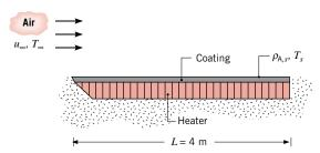
The molecular weight and the latent heat of vaporization of species A are  $\mathcal{M}_{\rm A}=150~{\rm kg/kmol}$  and  $h_{fg}=5.44\times10^6~{\rm J/kg}$ , respectively, and the mass diffusivity is  $D_{\rm AB}=7.75\times10^{-7}~{\rm m^2/s}$ . If the saturated vapor pressure of the substance is 0.12 atm at 134°C, what is the electrical power required to maintain steady-state conditions?
