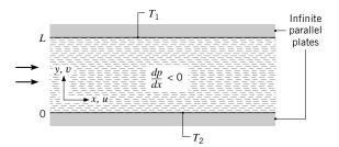
Referred to as *Poiseuille flow* with heat transfer, this special case of parallel flow is one for which the x velocity component is finite, but the y and z components (v and w) are zero.
