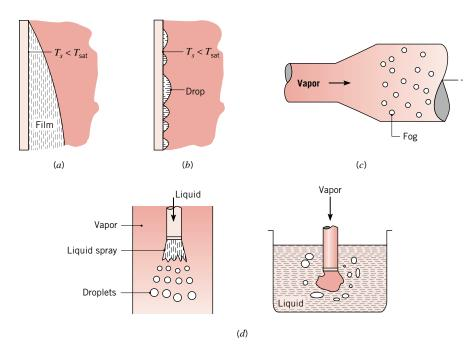
**FIGURE 10.9** Modes of condensation. (a) Film. (b) Dropwise condensation on a surface. (c) Homogeneous condensation or fog formation resulting from increased pressure due to expansion. (d) Direct contact condensation.
