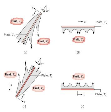
**FIGURE 9.6** Buoyancy-driven flows on an inclined plate: (a) side view of flows at top and bottom surfaces of a cold plate  $(T_s < T_{\infty})$ , (b) end view of flow at bottom surface of cold plate, (c) side view of flows at top and bottom surfaces of a hot plate  $(T_s > T_{\infty})$ , and (d) end view of flow at top surface of hot plate.
