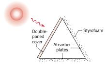
Identify all heat transfer processes associated with the cover plates, the absorber plate(s), and the air.
