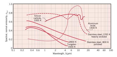
**FIGURE 12.17** Spectral dependence of the spectral, normal emissivity  $\varepsilon_{\lambda,n}$  of selected materials.
