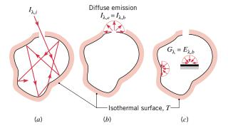
**FIGURE 12.11** Characteristics of an isothermal blackbody cavity. (a) Complete absorption. (b) Diffuse emission from an aperture. (c) Diffuse irradiation of interior surfaces.
