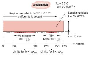
Use the finite-element method of *FEHT* to perform a conduction analysis on an axisymmetric EB of 340-mm diameter. The upper and lateral surfaces are exposed to the ambient fluid at  $T_{\infty} = 25^{\circ}\text{C}$  with a convection coefficient of  $10 \text{ W/m}^2 \cdot \text{K}$ . The lower surface of the EB is adiabatic, except for the ring sectors with the uniform applied heat fluxes,  $q_{\text{mh}}^{"}$  and  $q_{\text{th}}^{"}$ .
