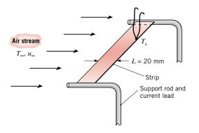
(a) Determine the relationship between the electrical power dissipation per unit width of the strip in the transverse direction, P' (mW/mm), and the airstream velocity. Show this relationship graphically for the specified range of  $u_{\infty}$ .
