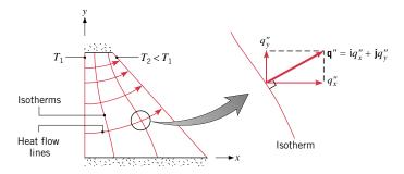
FIGURE 4.1 Two-dimensional conduction.
