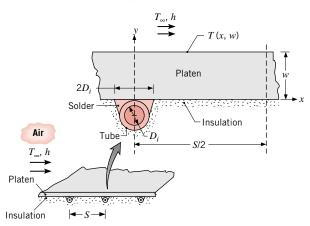
Considering the two-dimensional cross section of the platen shown in the inset, perform an analysis to determine the heating fluid temperature  $T_m$  and the tube spacing S required to maintain the surface temperature of the platen, T(x, w), at  $45 \pm 0.25$ °C, when the ambient temperature is 25°C and the convection coefficient is  $100 \text{ W/m}^2 \cdot \text{K}$ .
