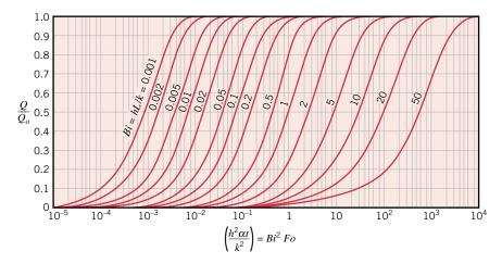
**FIGURE 58.3** Internal energy change as a function of time for a plane wall of thickness 2*L* [2]. Adapted with permission.
