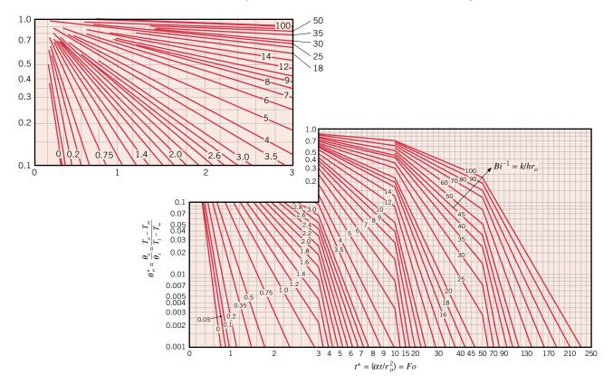
**FIGURE 58.7** Center temperature as a function of time in a sphere of radius  $r_o$  [1]. Used with permission.
