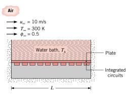
If the sides and bottom of the container are well insulated from the surroundings and heat is uniformly
