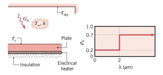
What is the electrical power  $(W/m^2)$  required to maintain the plate surface temperature at  $T_s = 60$ °C if the plate is diffuse and has the designated spectral, hemispherical reflectivity?
