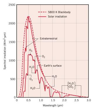
FIGURE 12.28 Spectral distribution of solar radiation.
