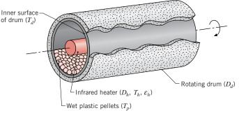
Consider the initial drying stage for a system comprised of a cylindrical heater aligned coaxially with a rotating drum of diameter  $D_d = 1$  m. Shortly after
