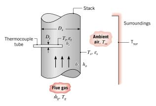
(b) Assuming the flue gas to have the properties of atmospheric air, evaluate the error for  $T_t = 300^{\circ}\text{C}$ ,  $D_s = 0.6 \text{ m}$ ,  $D_t = 10 \text{ mm}$ ,  $\dot{m}_g = 1 \text{ kg/s}$ ,  $T_{\infty} = T_{\text{sur}} = 27^{\circ}\text{C}$ ,  $\varepsilon_t = \varepsilon_s = 0.8$ , and  $h_o = 25 \text{ W/m}^2 \cdot \text{K}$ .
