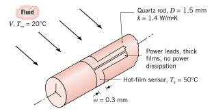
Proper operation is assured only if the heat generated in the film is transferred to the fluid, rather than conducted from the film into the quartz rod. Thermally, the film should therefore be strongly coupled to the fluid and weakly coupled to the quartz rod. This condition is satisfied if the Biot number is very large,  $Bi = \overline{h}D/2k \gg 1$ , where  $\overline{h}$  is the convection coefficient between the fluid and the film and k is the thermal conductivity of the rod.
