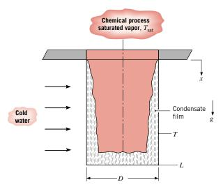
Derive an expression for the time,  $t_f$ , required to fill the container with condensate, assuming that the condensate film is laminar. Express your result in terms of D, L,  $(T_{\text{sat}} - T_s)$ , g, and appropriate fluid properties.
