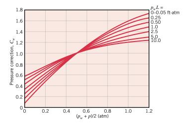
**FIGURE 13.16** Correction factor for obtaining water vapor emissivities at pressures other than 1 atm  $(\varepsilon_{w,p\neq 1 \text{atm}} = C_w \varepsilon_{w,p=1 \text{atm}})$  [13]. Used with permission.
