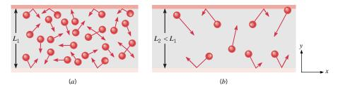
**FIGURE 2.6** Electron or phonon trajectories in (a) a relatively thick film and (b) a relatively thin film with boundary effects.
