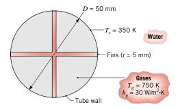
If the tube surface temperature is  $T_s = 350$  K and the gas-side convection coefficient is  $h_g = 30$  W/m<sup>2</sup> · K, what is the rate of heat transfer to the water per meter of pipe length?
