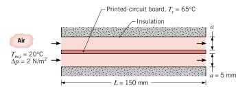
Calculate the average heat removal rate per unit area (W/m<sup>2</sup>) from the PCB.
