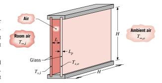
(a) Neglecting the thermal resistance associated with conduction heat transfer across each pane, determine the corresponding temperature of each pane and the rate of heat transfer through the window.
