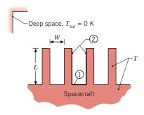
absolute zero temperature. The fins and the base may be assumed to be isothermal at a temperature *T*. Comment on your result. Does the engineer's proposal have merit?
