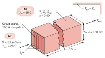
Your assignment is to develop a model to estimate the outlet temperature of the air,  $T_{m,o}$ , and the average surface temperature of the duct,  $\overline{T}_s$ .
