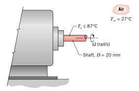
(a) For horizontal rotating cylinders, a suitable correlation for estimating the convection coefficient is of the form
