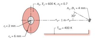
What is the irradiation on  $A_1$  due to radiation from  $A_2$ , which is a diffuse, gray surface with an emissivity of 0.7?
