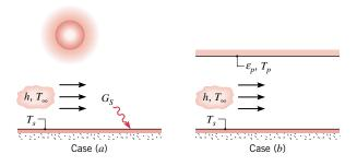
(b) In case (b) the surface is shielded from the sun by a large plate and an airflow is maintained between the plate and the surface. The plate is diffuse and gray with an emissivity of  $\varepsilon_p = 0.8$ . If  $T_\infty = 300$  K and the convection coefficient is equivalent to the result obtained in part (a), what is the plate temperature  $T_p$  that is needed to maintain the surface at  $T_s = 320$  K?
