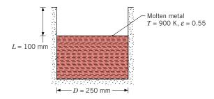
If the oxidized aluminum at the surface of the melt has an emissivity of 0.55, what is the net rate of radiation heat transfer from the melt?
