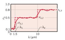
Determine the total, hemispherical emissivity and emissive power of the fire brick wall. What is the total absorptivity of the wall to irradiation resulting from emission by the coals?
