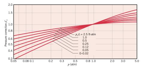
**FIGURE 13.18** Correction factor for obtaining carbon dioxide emissivities at pressures other than 1 atm  $(\varepsilon_{c,p\neq 1\text{atm}} = C_c\varepsilon_{c,p=1\text{atm}})$  [13]. Used with permission.
