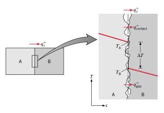
**FIGURE 3.4** Temperature drop due to thermal contact resistance.
