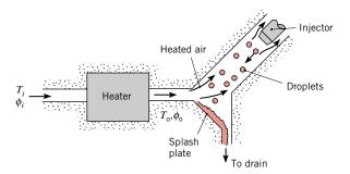
Consider conditions for which air enters the heater at a temperature and relative humidity of 17°C and 70%, respectively, and leaves the heater at a temperature of 47°C. The droplet diameter is 1 mm, and the relative velocity between the droplets and the heated air is 15 m/s. During the time-of-flight, the change in droplet diameter may be neglected and the droplet temperature may be assumed to remain at 47°C. What is the rate of evaporation from a single droplet?
