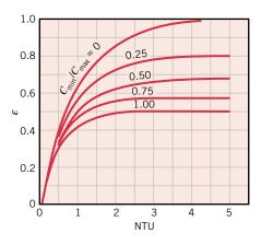
**FIGURE 11.10** Effectiveness of a parallel-flow heat exchanger (Equation 11.28).
