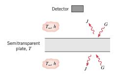
$h = 40 \text{ W/m}^2 \cdot \text{K}$ . The total, hemispherical absorptivity of the plate to the irradiation is 0.40. Under steady-state conditions measurements made with a radiation detector above the top surface indicate a radiosity (which includes transmission, as well as reflection and emission) of  $J = 5000 \text{ W/m}^2$ , while the plate is at a uniform temperature of T = 350 K.
