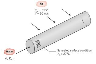
To maintain an approximately uniform surface temperature of 27°C, water at a prescribed flow rate and temperature passes through the tube.
