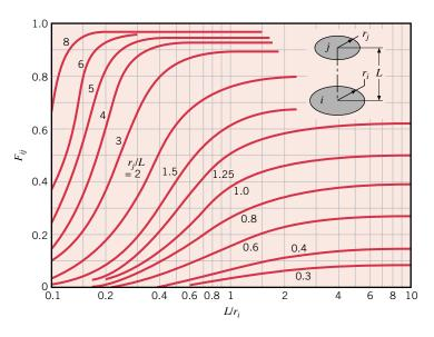
**FIGURE 13.5** View factor for coaxial parallel disks.
