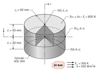
(a) Calculate the temperatures, T(r, x, t), after 3 min at the cylinder center, T(0, 0, 3 min), at the center of a circular face, T(0, L, 3 min), and the midheight of the side,  $T(r_o, 0, 3 \text{ min})$ .
