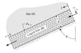
The flow is sustained by gravity, and the gas species A outside the film is absorbed at the liquid–gas interface. The film is in fully developed laminar flow over the entire plate, such that its velocity components in the y and z directions are zero. The mass density of A at y=0 in the liquid is a constant  $\rho_{A, \rho}$  independent of x.
