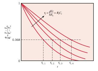
**FIGURE 5.2** Transient temperature response of lumped capacitance solids for different thermal time constants  $\tau_t$ .
