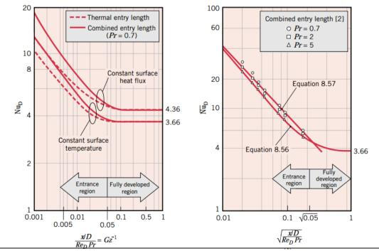
For the constant surface temperature condition, it is desirable to know the average convection coefficient, presents a correlation attributed to Hausen, which is of the form:
