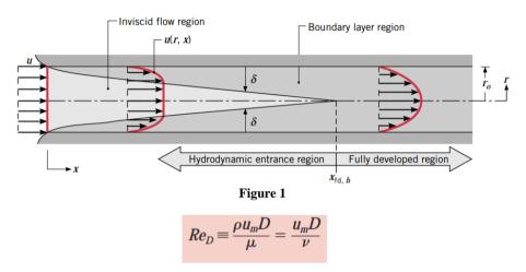
Where  $U_m$  is the mean fluid velocity over the cross section and D is the diameter.
