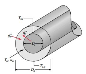
FIGURE 8.11 The concentric tube annulus.
