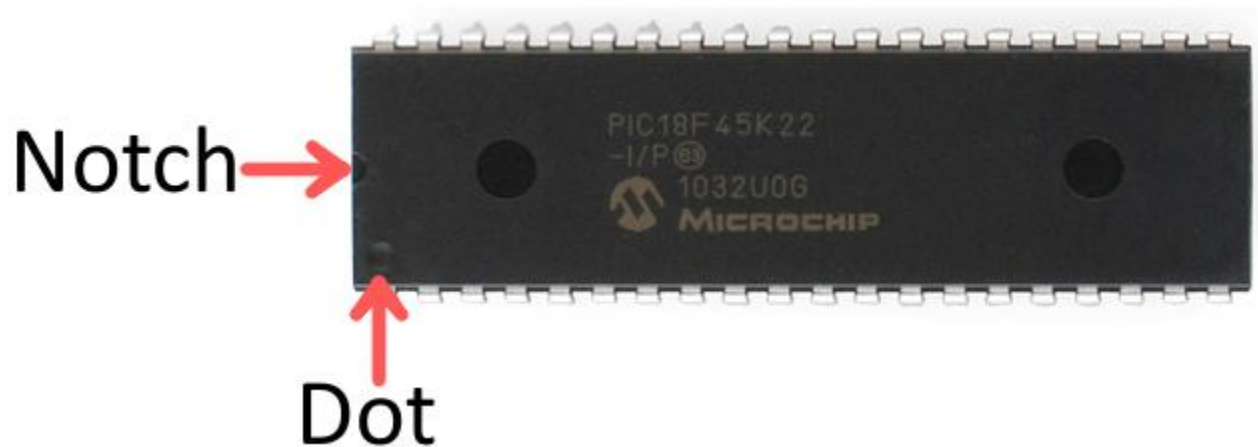
Fig 3.8. Polarity and pin numbering of ICs
