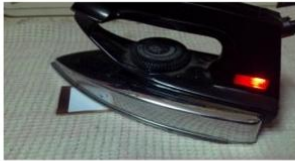
Iron the paper onto the plate
