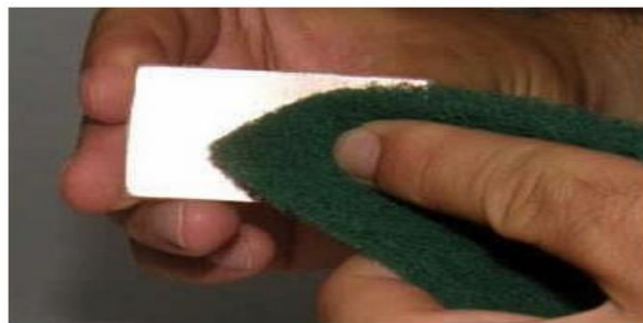
Rubbing away the top oxide layer
