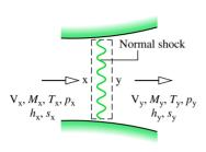
▲ **Figure 9.31** Control volume enclosing a normal shock.
