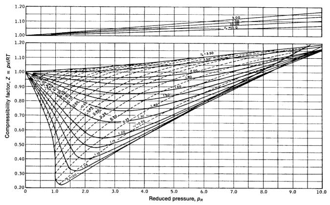
**Figure A-2** Generalized compressibility chart,  $p_R \le 10.0$ . Source: E. F. Obert, Concepts of Thermodynamics, McGraw-Hill, New York, 1960.
