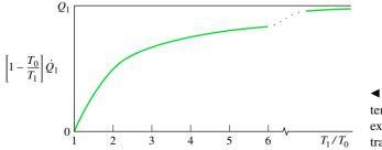
**Figure 7.9** Effect of the temperature ratio  $T_1/T_0$  on the exergy loss associated with heat transfer.
