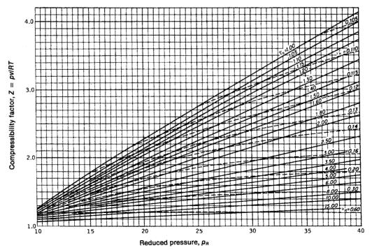
**Figure A-3** Generalized compressibility chart,  $10 \le p_R \le 40$ . Source: E. F. Obert. Concepts of Thermodynamics, McGraw-Hill, New York, 1960.
