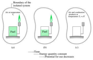
▲ **Figure 7.1** Illustration used to introduce exergy.
