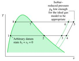
**Figure 11.4** *T*–v diagram used to discuss how *h* and *s* can be assigned to liquid and vapor states.
