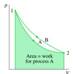
▲ Figure 2.8 Illustration that work depends on the process.
