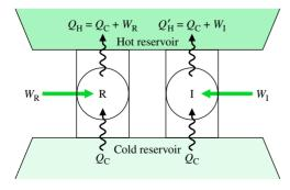
◄ Figure 5.8 Sketch for demonstrating that a reversible refrigeration cycle R has a greater coefficient of performance than an irreversible cycle I when they operate between the same two reservoirs.
