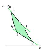
▲ **Figure 5.13** p-v diagram for a Carnot gas refrigeration or heat pump cycle.
