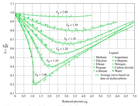
▲ Figure 3.12 Generalized compressibility chart for various gases.
