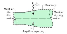
◄ Figure 12.10 System for conditioning moist air.
