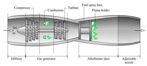
▲ **Figure 9.21** Schematic of a turbojet engine with afterburner.
