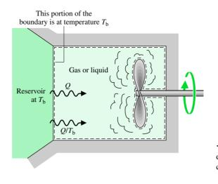
◄ Figure 6.8 Illustration of the entropy transfer and entropy production concepts.
