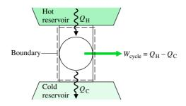
◄ Figure 5.5 System undergoing a power cycle while exchanging energy by heat transfer with two reservoirs.
