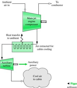
◄ Figure 10.15 An application of gas refrigeration to aircraft cabin cooling.
