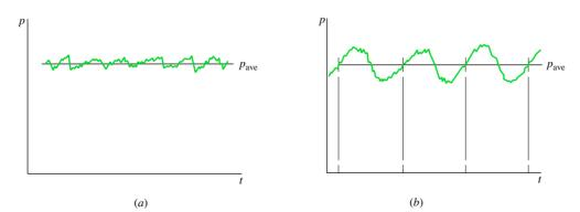
▲ Figure 4.5 Pressure variations about an average. (*a*) Fluctuation. (*b*) Periodic.
