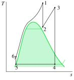
▲ **Figure 8.8** Supercritical ideal reheat cycle.
