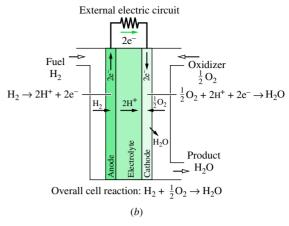
**Figure 13.3** Fuel cell power systems. (a) 25-kW solid oxide fuel cell module. (b) Schematic of a proton exchange membrane fuel cell.
