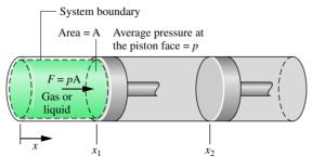
◄ Figure 2.4 Expansion or compression of a gas or liquid.
