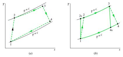
▲ Figure 9.13 Effects of irreversibilities on the air-standard gas turbine.
