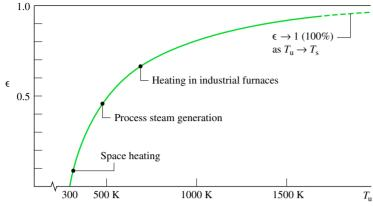
▲ Figure 7.8 Effect of use temperature  $T_{\rm u}$  on the exergetic efficiency  $\varepsilon$  ( $T_{\rm s} = 2200$  K,  $\eta = 100\%$ ).
