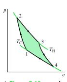
▲ **Figure 5.10** p-v diagram for a Carnot gas power cycle.
