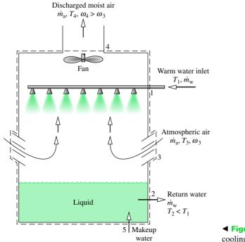
◄ Figure 12.15 Schematic of a cooling tower.
