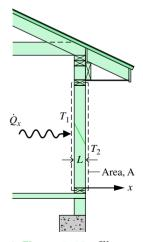
▲ Figure 2.12 Illustration of Fourier's conduction law.
