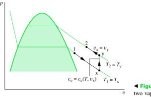
**← Figure 11.2** Integration path between two vapor states.
