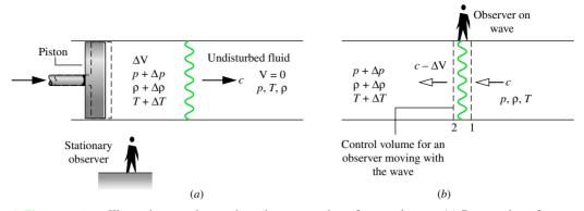
**Figure 9.27** Illustrations used to analyze the propagation of a sound wave. (*a*) Propagation of a pressure wave through a quiescent fluid, relative to a stationary observer. (*b*) Observer at rest relative to the wave.
