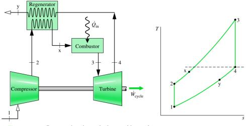
▲ **Figure 9.14** Regenerative air-standard gas turbine cycle.
