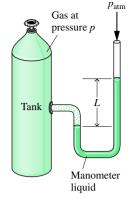
▲ Figure 1.6 Pressure measurement by a manometer.
