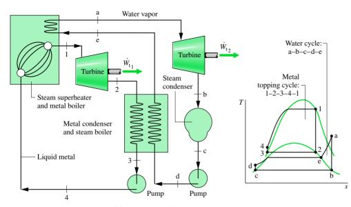
▲ **Figure 8.13** Water–metal binary vapor cycle.
