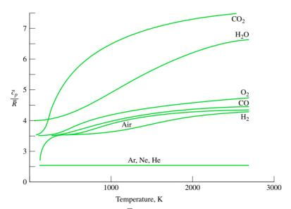
**Figure 3.13** Variation of  $\overline{c}_p/\overline{R}$  with temperature for a number of gases modeled as ideal gases.
