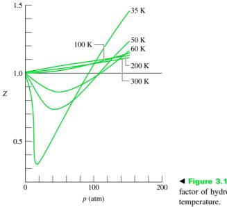
◄ Figure 3.11 Variation of the compressibility factor of hydrogen with pressure at constant temperature.
