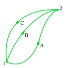
▲ Figure 6.2 Two internally reversible cycles.
