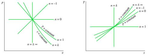
**Figure 6.11** Polytropic processes on p-v and T-s diagrams.
