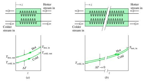
▲ **Figure 9.15** Temperature distributions in counterflow heat exchangers. (*a*) Actual. (*b*) Reversible.
