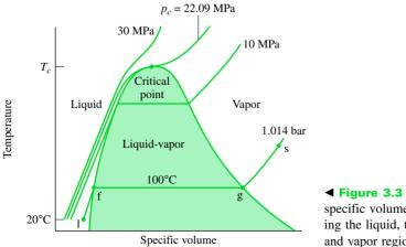
◄ Figure 3.3 Sketch of a temperature– specific volume diagram for water showing the liquid, two-phase liquid–vapor, and vapor regions (not to scale). saturation temperature
