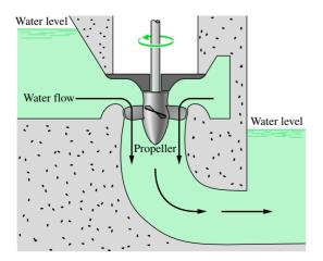
**Figure 4.9** Hydraulic turbine installed in a dam.
