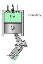
▲ **Figure 1.1** Closed system: A gas in a piston–cylinder assembly.
