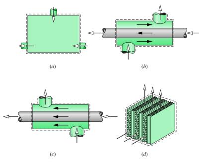
**Figure 4.12** Common heat exchanger types. (*a*) Direct contact heat exchanger. (*b*) Tube-within-a-tube counterflow heat exchanger. (*c*) Tube-within-a-tube parallel flow heat exchanger. (*d*) Cross-flow heat exchanger.
