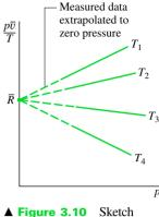
• Figure 3.10 Sketch of  $p\overline{v}/T$  versus pressure for a gas at several specified values of temperature.
