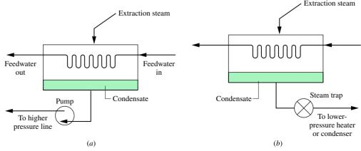
▲ Figure 8.10 Examples of closed feedwater heaters.
