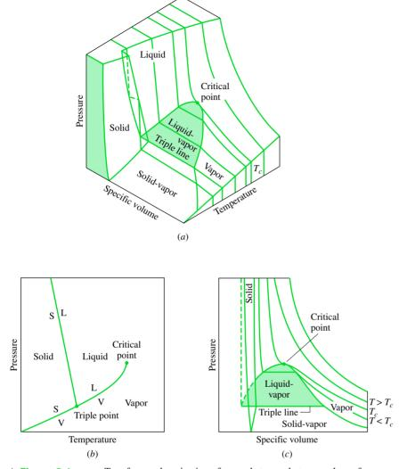
▲ Figure 3.1 p-v-T surface and projections for a substance that expands on freezing. (*a*) Three-dimensional view. (*b*) Phase diagram. (*c*) p-v diagram.
