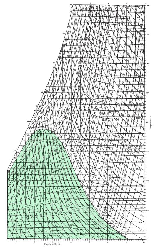
**Figure A-7** Temperature–entropy diagram for water (SI units). *Source:* J. H. Keenan, F. G. Keyes, P. G. Hill, and J. G. Moore, *Steam Tables*, Wiley, New York, 1978.
