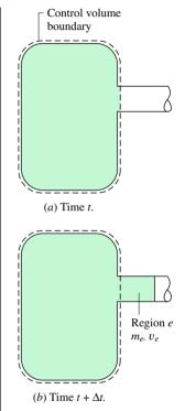
▲ **Figure 7.6** Illustration used to introduce the flow exergy concept.
