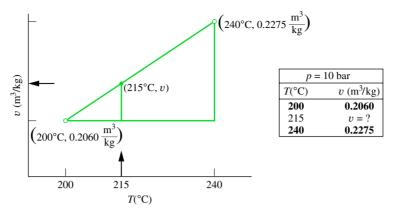
▲ Figure 3.7 Illustration of linear interpolation.
