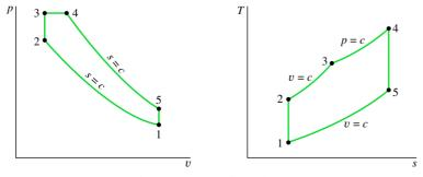
**Figure 9.7** p-v and T-s diagrams of the air-standard dual cycle.
