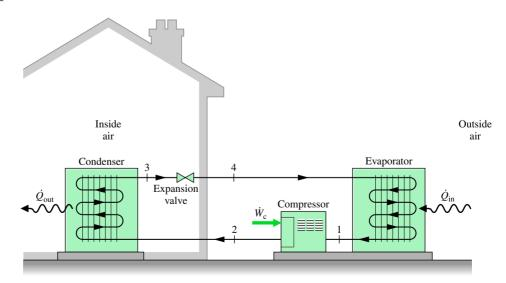
▲ Figure 10.11 Air-source vapor-compression heat pump system.
