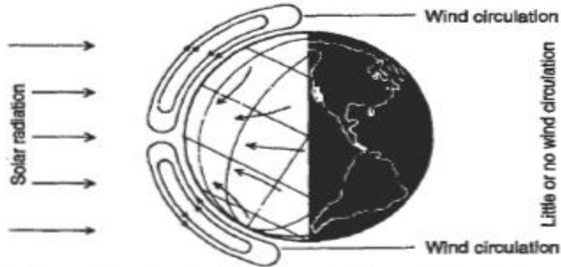
A. If the earth did not turn, the air would circulate in a fixed pattern
