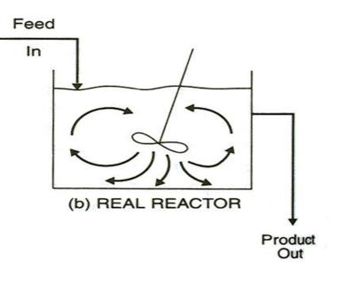
For time-dependent reactions, the time that a fluid particle remains in the reactor obviously affects the degree to which the reaction goes to completion.
