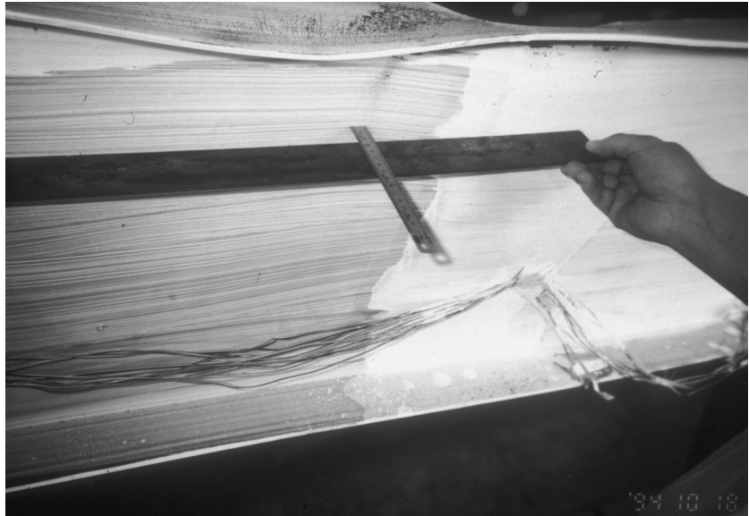
Fig. 8.42 Local buckling of web. (Courtesy of Structures/Materials Laboratory, Virginia Tech.)
