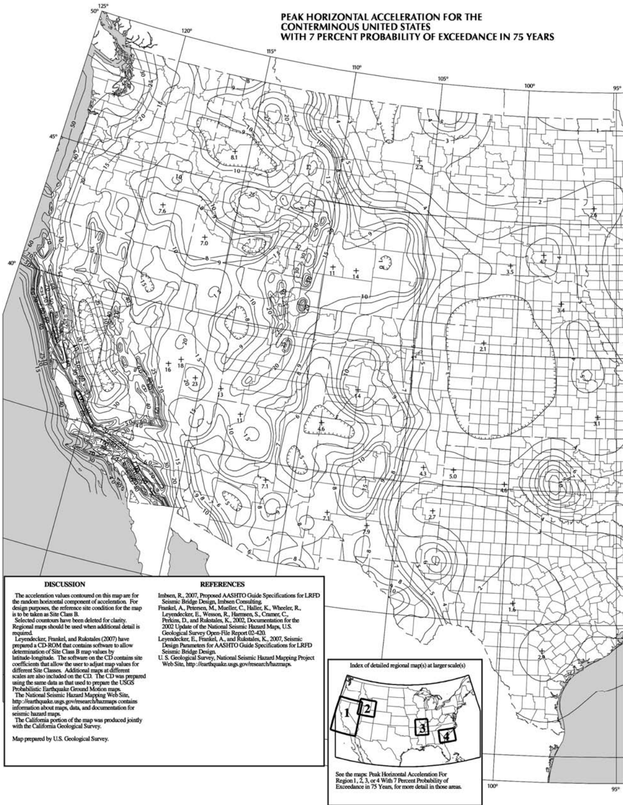
Figure 3.4.1-2a—Horizontal Peak Ground Acceleration Coefficient for the Conterminous United States (PGA) with Seven Percent Probability of Exceedance in 75 yr (Approx. 1000-yr Return Period)
