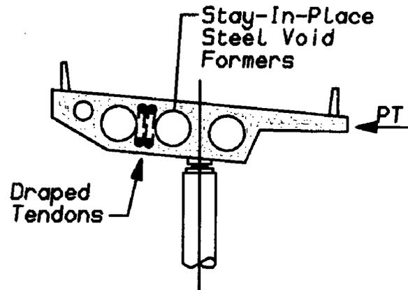
Figure C5.14.4.2.1-1—Cross-Section of Typical Voided Concrete Deck System
