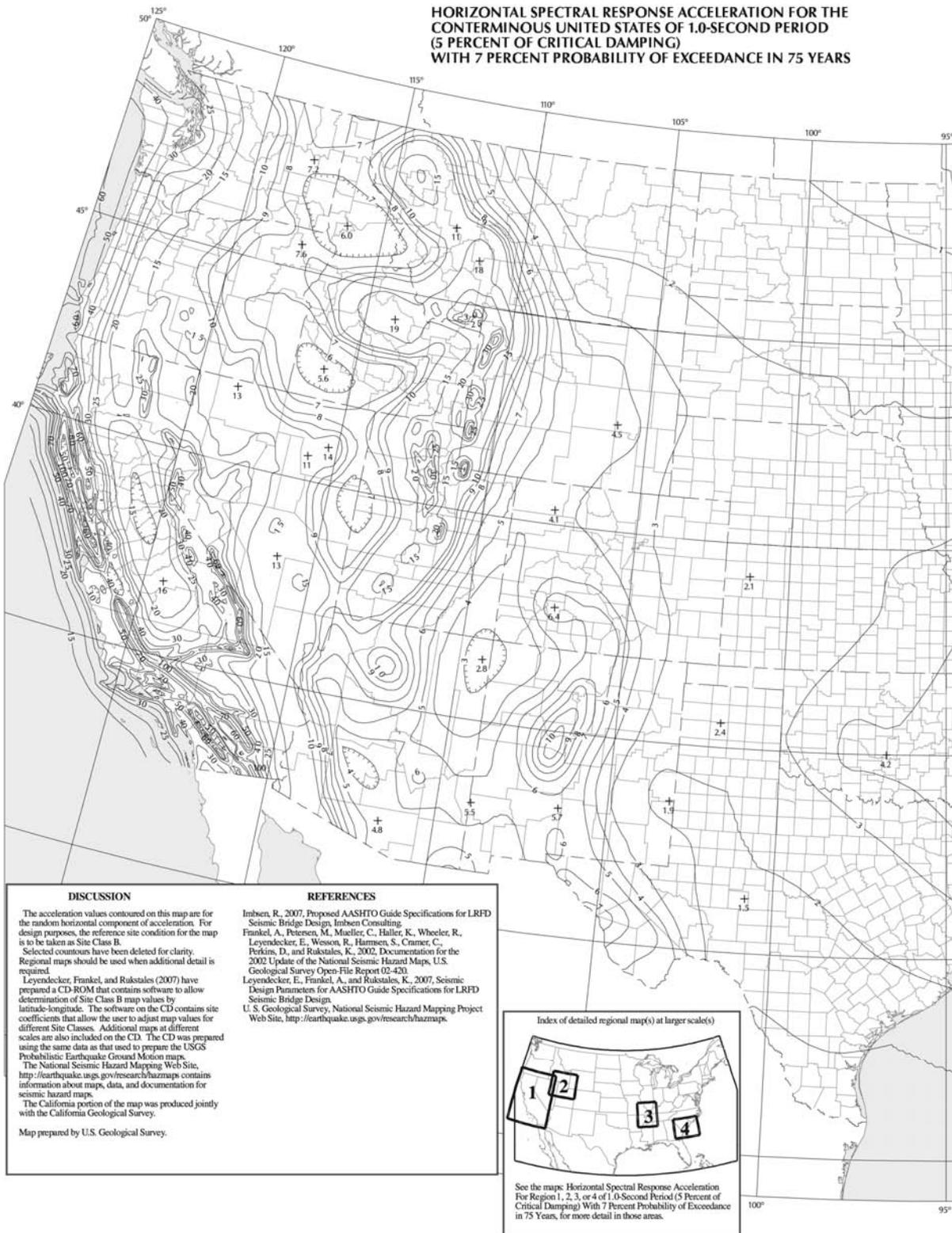
**Figure 3.10.2.1-3—Horizontal Response Spectral Acceleration Coefficient for the Conterminous United States at Period of 1.0 s ( $S_1$ ) with Seven Percent Probability of Exceedance in 75 yr (Approx. 1000-yr Return Period) and Five Percent Critical Damping**
