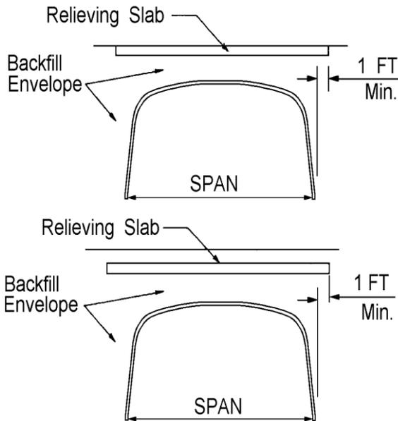
**Figure 12.9.4.6-1—Metal Box Culverts with Concrete Relieving Slab**
