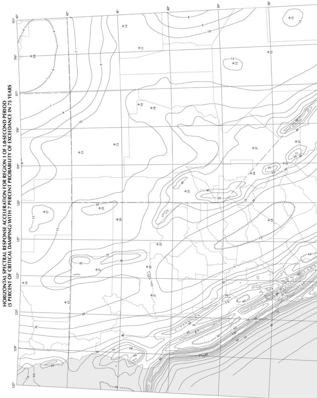
**Figure 3.10.2.1-6—Horizontal Response Spectral Acceleration Coefficient for Region 1 at Period of 1.0 s ( $S_1$ ) with Seven Percent Probability of Exceedance in 75 yr (Approx. 1000-yr Return Period) and Five Percent Critical Damping**
