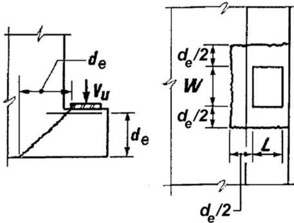
Figure 5.13.2.5.4-1—Design of Beam Ledges for Punching Shear
