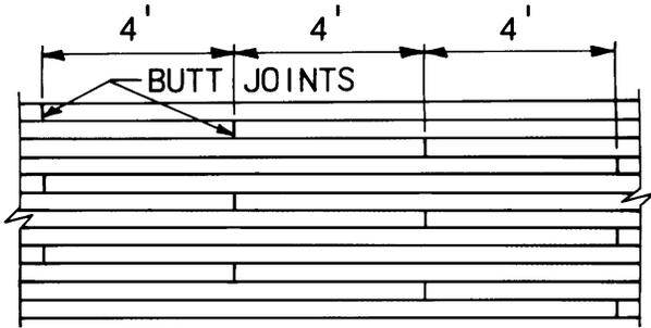
**Figure 9.9.5.3-1—Minimum Spacing of Lines of Butt Joints**
