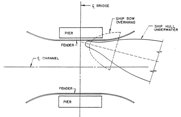
Figure C3.14.14.1-1—Plan of Ship Bow Overhang Impacting Pier
