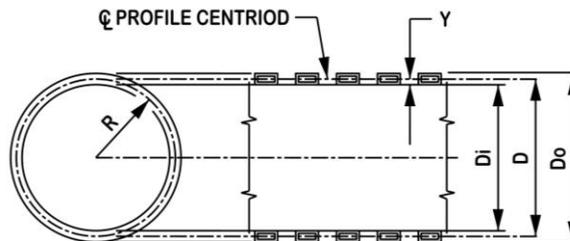
Figure C12.12.2.2-1—Schematic for Thermoplastic Pipe Terms
