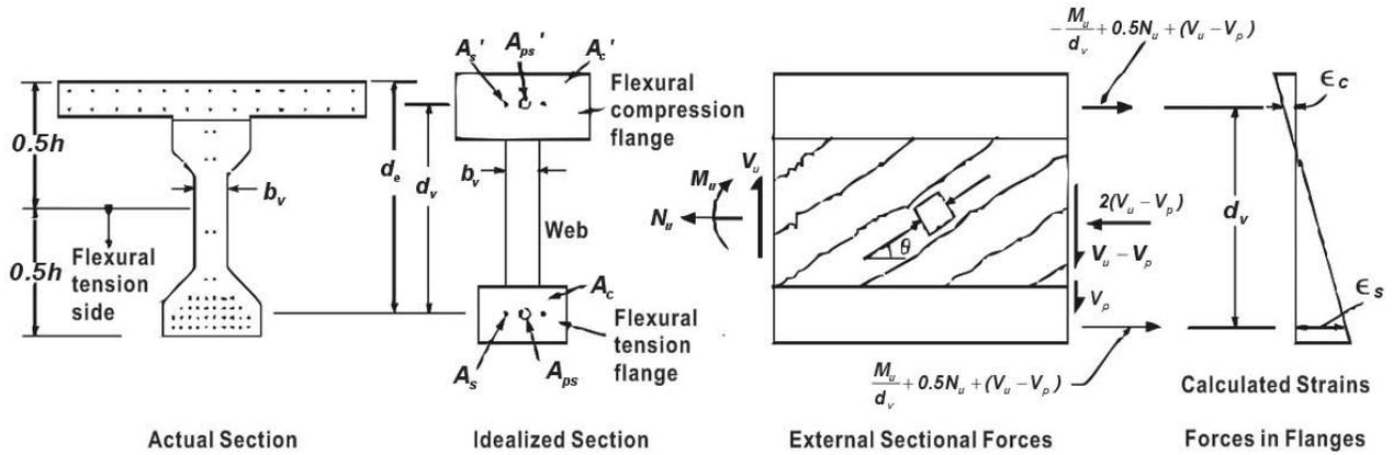
Figure C5.8.3.4.2-3—More Accurate Calculation Procedure for Determining  $\epsilon_s$
