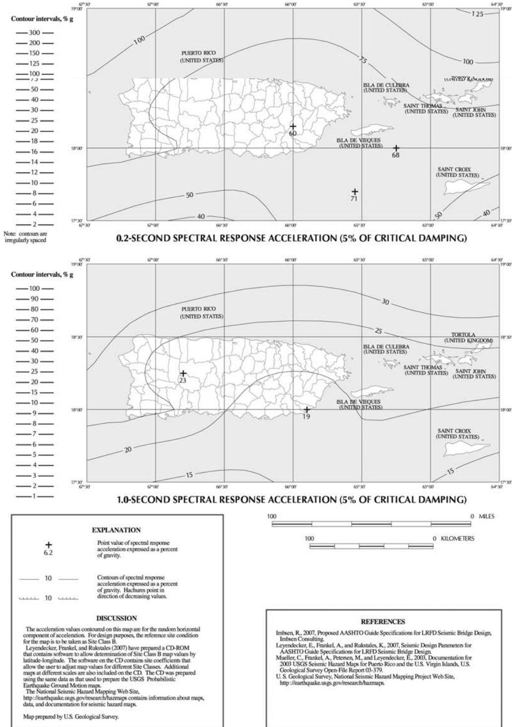
**Figure 3.10.2.1-21—Horizontal Response Spectral Acceleration Coefficients for Puerto Rico, Culebra, Vieques, St. Thomas, St. John, and St. Croix at Periods of 0.2 s ( $S_0$ ) and 1.0 s ( $S_1$ ) with Seven Percent Probability of Exceedance in 75 yr (Approx. 1000-yr Return Period) and Five Percent Critical Damping**
