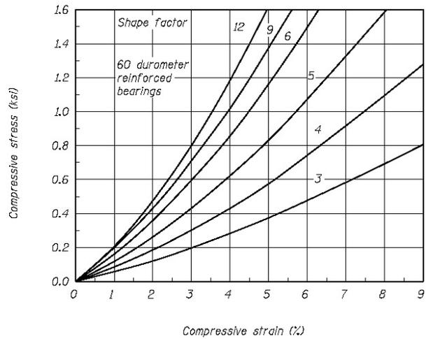
Figure C14.7.6.3.3-1—Stress-Strain Curves
