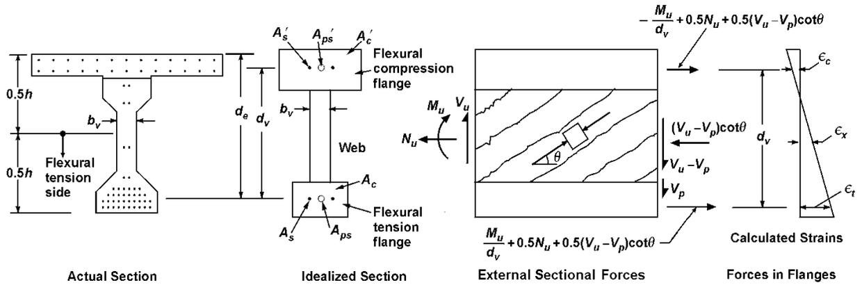
Figure CB5.2-3—More Accurate Calculation Procedure for Determining  $\epsilon_x$
