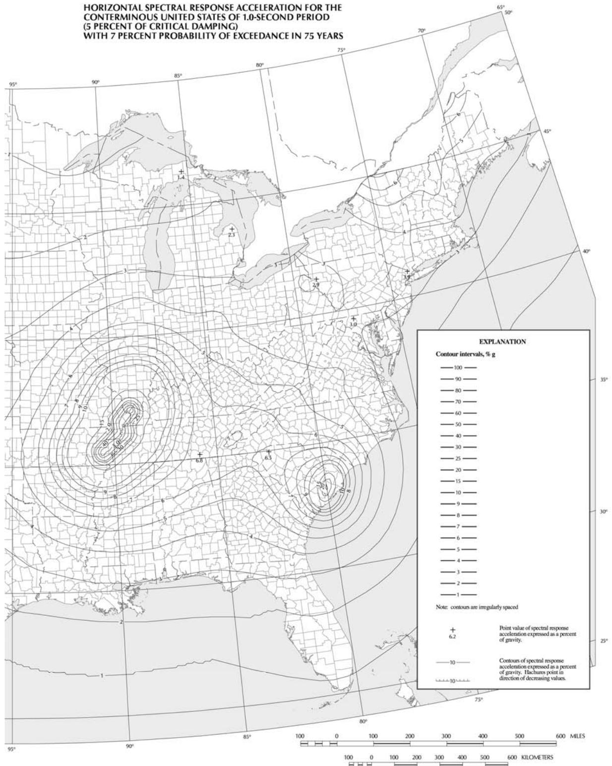
**Figure 3.10.2.1-3 (continued)—Horizontal Response Spectral Acceleration Coefficient for the Conterminous United States at Period of 1.0 s ( $S_1$ ) with Seven Percent Probability of Exceedance in 75 yr (Approx. 1000-yr Return Period) and Five Percent Critical Damping**
