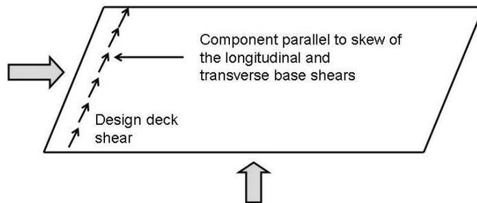
Figure C6.16.4.2-1—Design Deck Shear,  $F_{px}$ , at Skewed Supports
