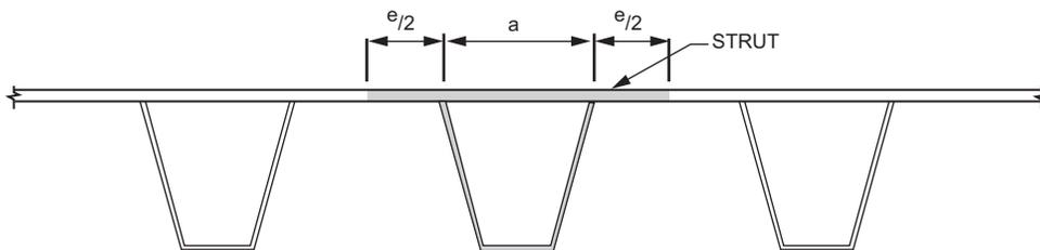
Figure 6.14.3.2.3-1—Idealized Strut for Evaluation of Compressive Resistance
