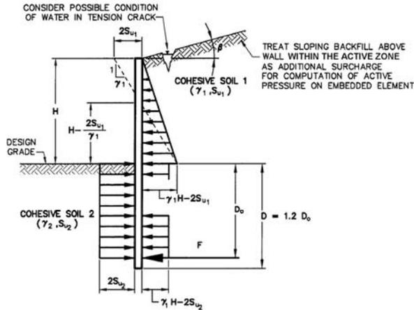
**Figure 3.11.5.6-7—Unfactored Simplified Earth Pressure Distributions for Temporary Nongravity Cantilevered Walls with Continuous Vertical Wall Elements Embedded in Cohesive Soil and Retaining Cohesive Soil Modified after Teng (1962)**
