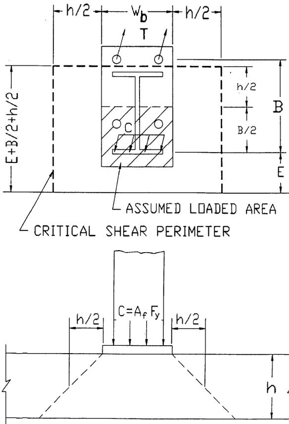
Figure A13.4.3.2-1—Punching Shear Failure Mode
