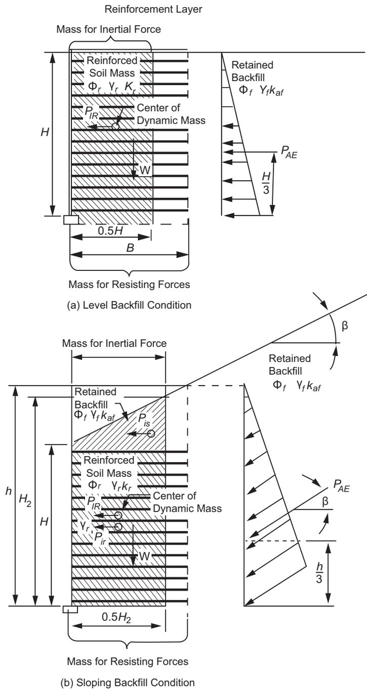
Figure 11.10.7.1-1—Seismic External Stability of an MSE Wall
