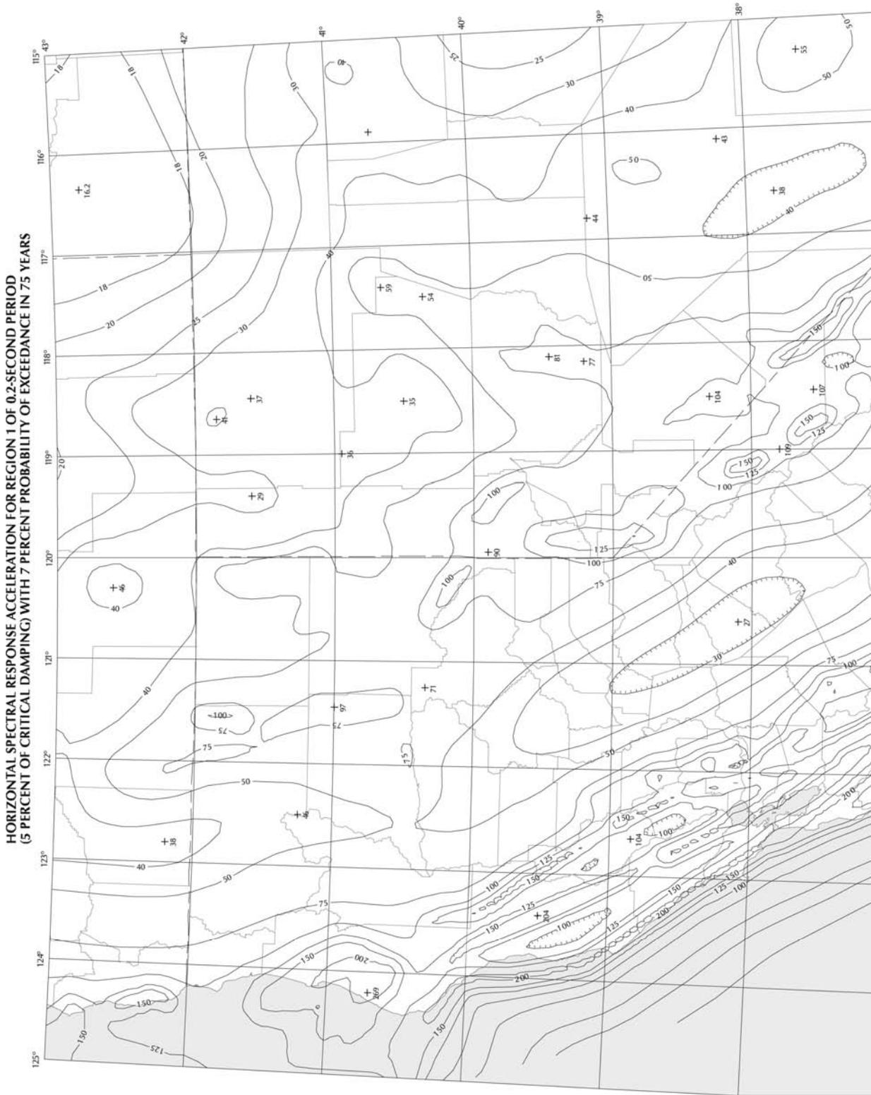
**Figure 3.10.2.1-5—Horizontal Response Spectral Acceleration Coefficient for Region 1 at Period of 0.2 s ( $S_S$ ) with Seven Percent Probability of Exceedance in 75 yr (Approx. 1000-yr Return Period) and Five Percent Critical Damping**
