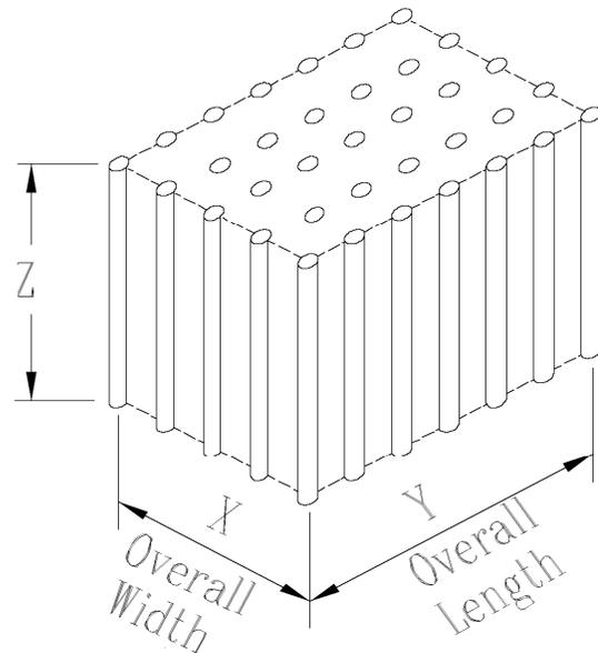
**Figure C10.7.3.9-1—Pile Group Acting as a Block Foundation**
