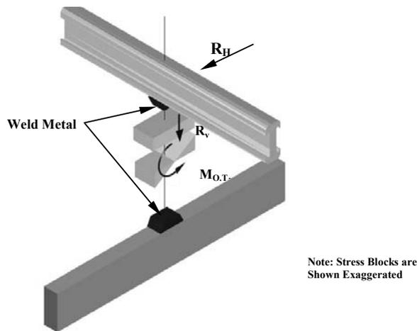
Figure 14.5.6.9.7b-3—Force Effects Associated with Type C Cracking
