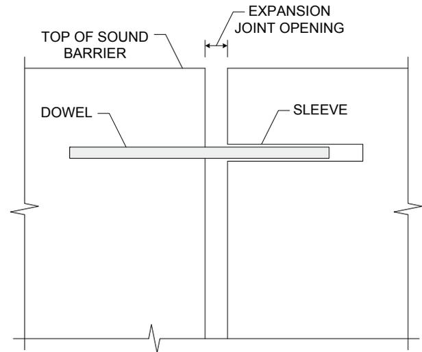
Figure C15.6.3-1—Sliding Dowel-and-Sleeve Connection
