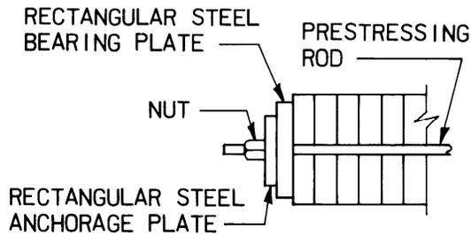
C. BEARING PLATE ANCHORAGE CONFIGURATION.
