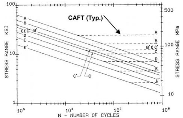
Figure C6.6.1.2.5-1—Stress Range Versus Number of Cycles
