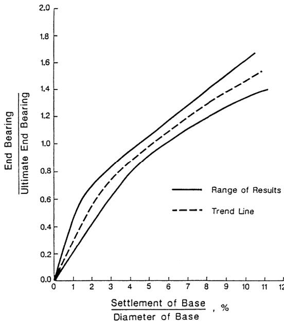
Figure 10.8.2.2.2-4—Normalized Load Transfer in End Bearing versus Settlement in Cohesionless Soils (from O’Neill and Reese, 1999)
