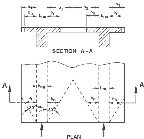
Figure 4.6.2.6.2-4—Effective Flange Widths,  $b_n$ , for Normal Forces
