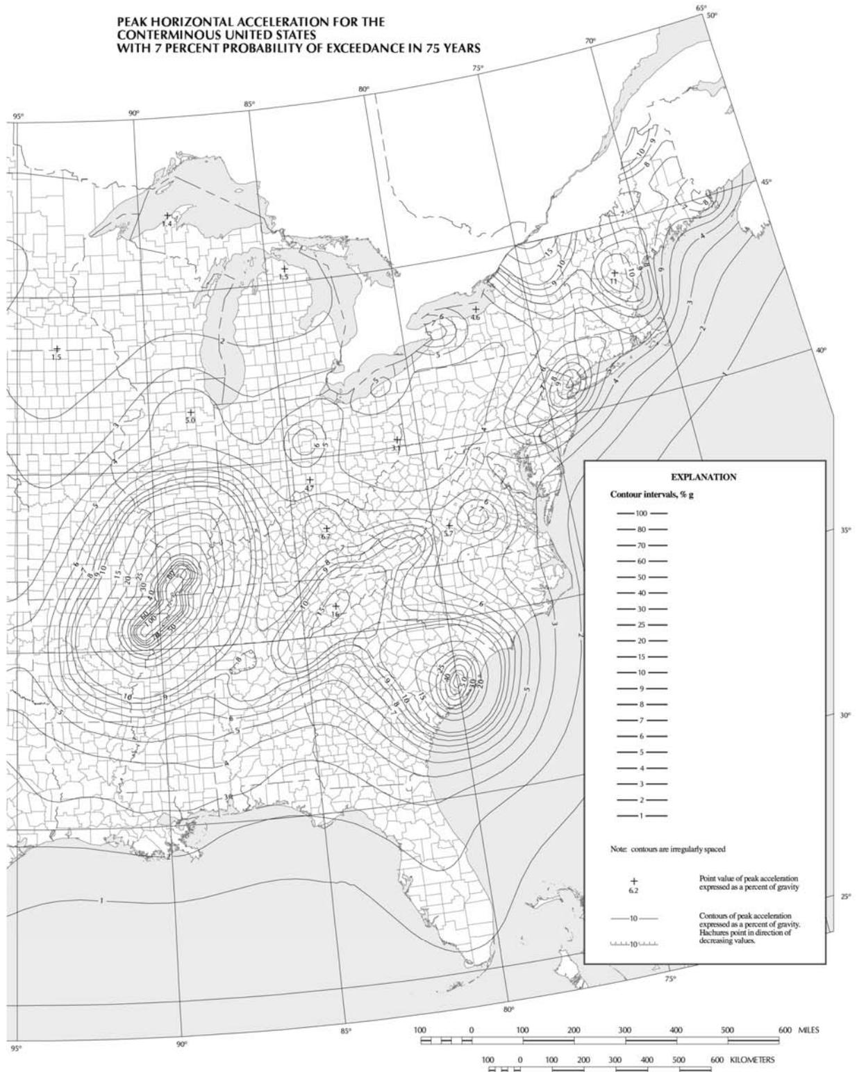
**Figure 3.10.2.1-1 (continued)—Horizontal Peak Ground Acceleration Coefficient for the Contiguous United States (PGA) with Seven Percent Probability of Exceedance in 75 yr (Approx. 1000-yr Return Period)**
