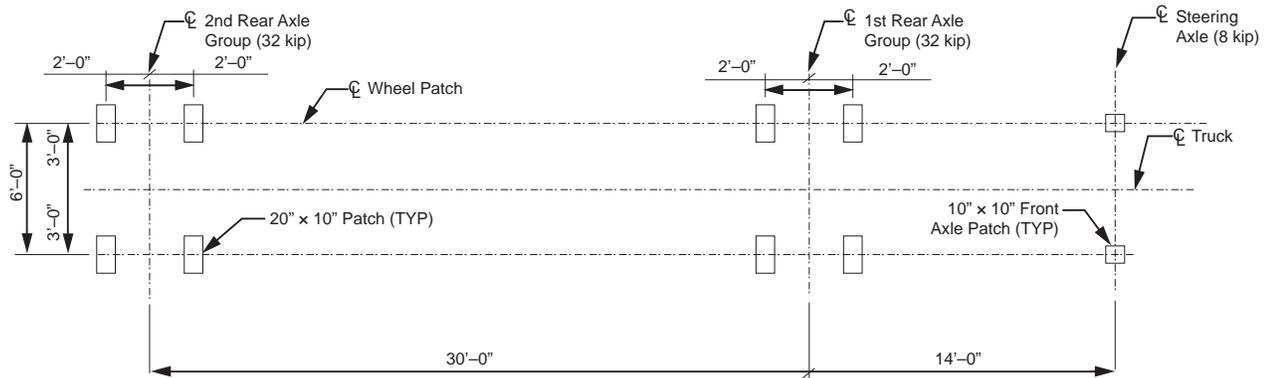
Figure 3.6.1.4.1-1—Refined Design Truck Footprint for Fatigue Design
