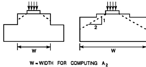
Figure C5.7.5-1—Determination of  $A_2$  for a Stepped Support
