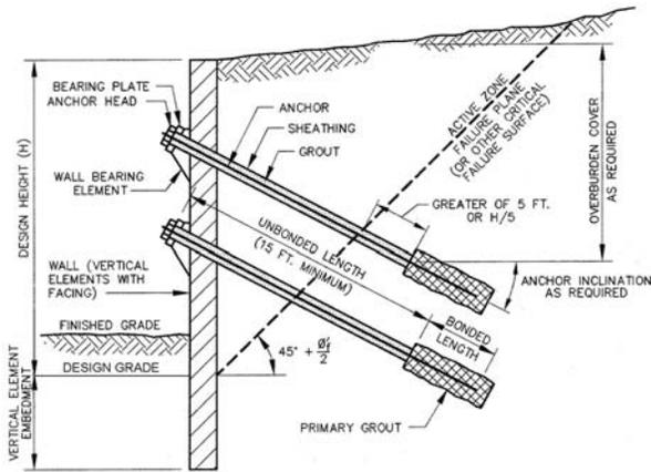
**Figure 11.9.1-1—Anchored Wall Nomenclature and Anchor Embedment Guidelines**
