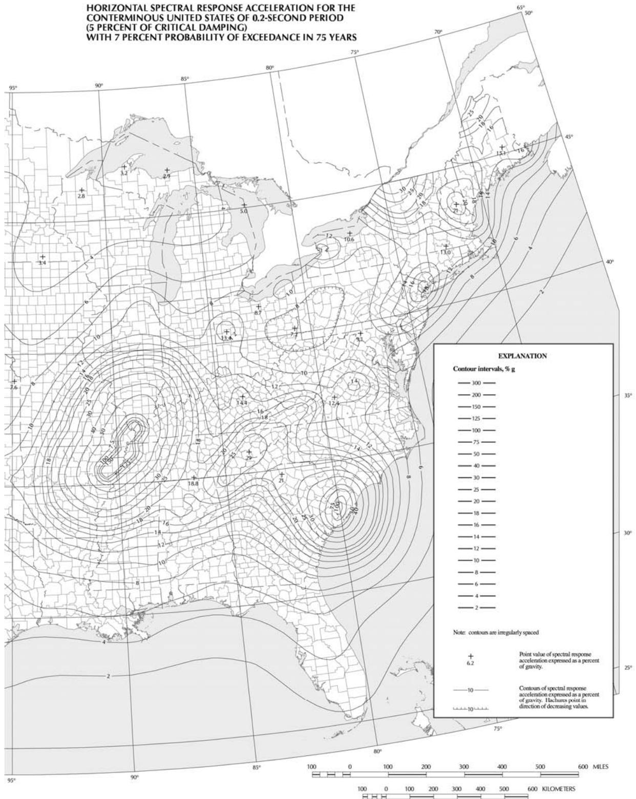
**Figure 3.10.2.1-2 (continued)—Horizontal Response Spectral Acceleration Coefficient for the Conterminous United States at Period of 0.2 s ( $S_S$ ) with Seven Percent Probability of Exceedance in 75 yr (Approx. 1000-yr Return Period) and Five Percent Critical Damping**
