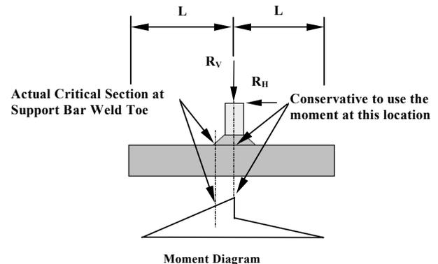
Figure C14.5.6.9.7b-1—Typical Moment Diagram for a Support Bar
