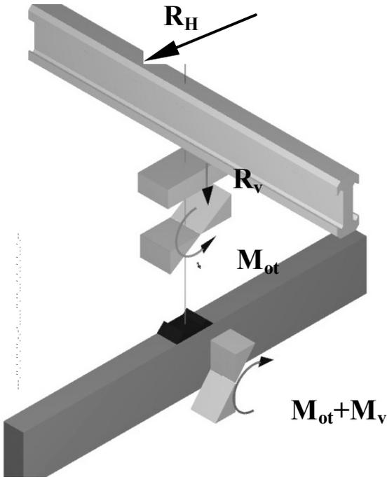
Figure 14.5.6.9.7b-2—Force Effects Associated with Type B Cracking
