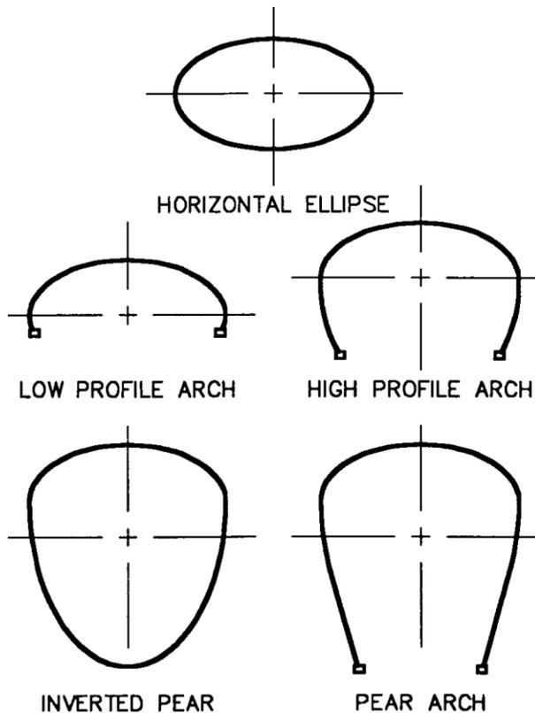
Figure 12.8.1-1—Long-Span Shapes
