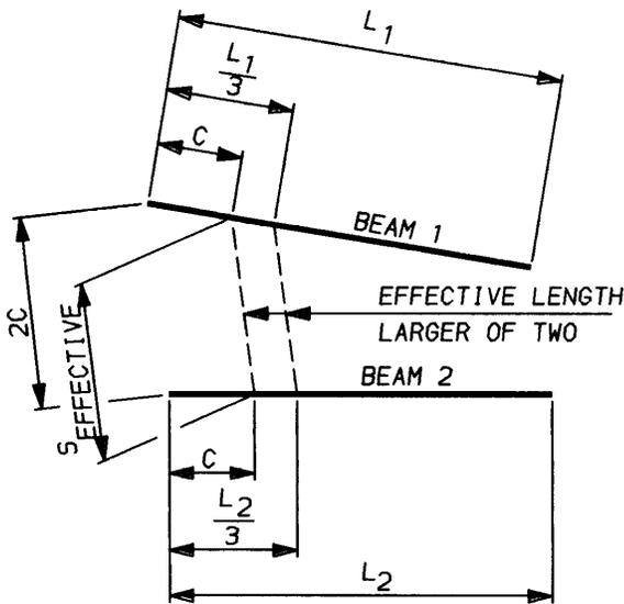
Figure 9.7.2.3-1—Effective Length for Nonuniform Spacing of Beams
