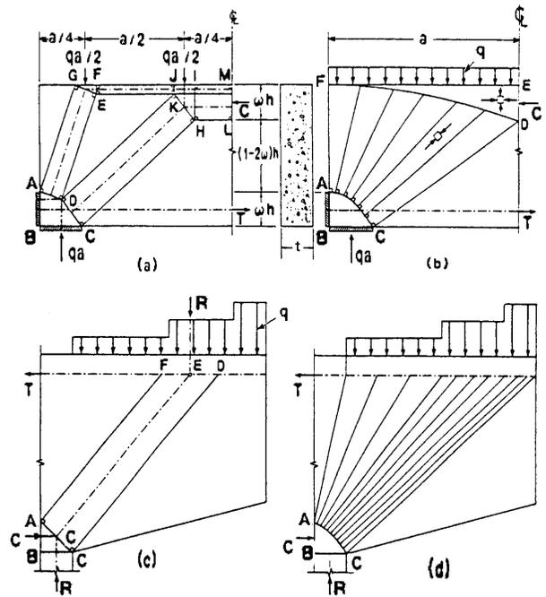
Figure C5.13.2.3-1—Fan Action: (a) Strut-and-Tie Model of Uniformly-Loaded Deep Beam; (b) Fan-Shaped Stress Field; (c) Strut-and-Tie System for Equivalent Single-Load  $R$  Replacing Distributed-Load  $q$ ; (d) Continuous Fan Developed from Discrete Strut
