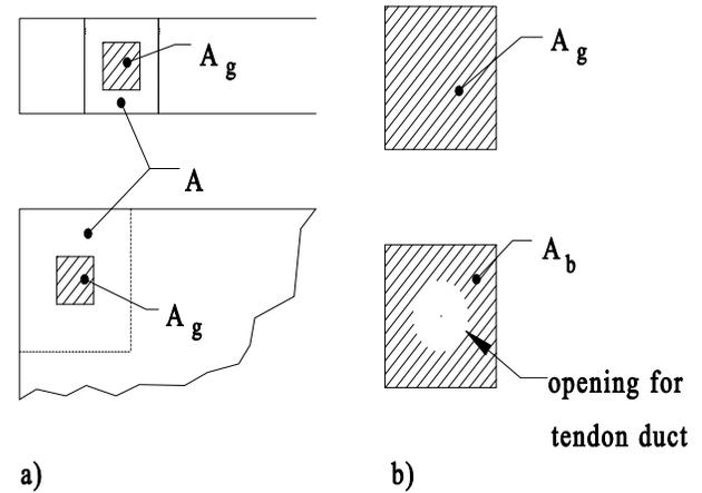
Figure C5.10.9.7.2-1—Area of Supporting Concrete Surface in Eq. 5.10.9.7.2-2
