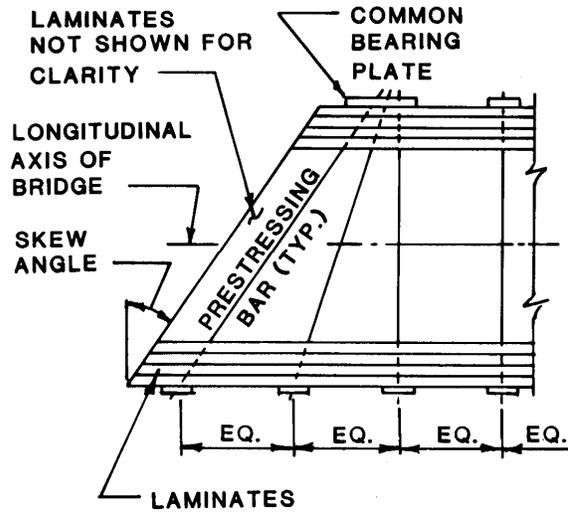
Potential concentration of bearing stresses and sliding of the common bearing plate should be considered in conjunction with the fanned arrangement of prestressing elements shown in Figure 9.9.5.6.1-1.
