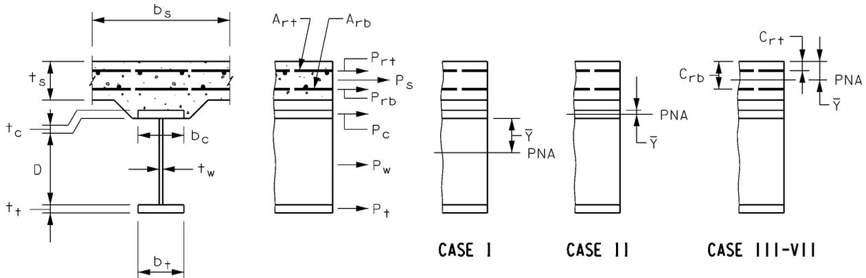
Table D6.1-2—Calculation of  $\bar{Y}$  and  $M_p$  for Sections in Negative Flexure
