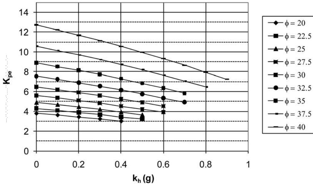
Figure A11.4-3—Seismic Passive Earth Pressure Coefficient Based on Log Spiral Procedure for  $c/\gamma H = 0.1$  and  $0.15$  ( $c$  = soil cohesion,  $\gamma$  = soil unit weight, and  $H$  = retaining wall height or depth of wall over which the passive resistance acts)
