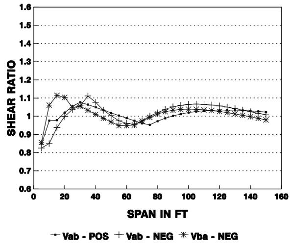
Figure C3.6.1.2.1-4—Shear Ratios: Exclusion Vehicles to Notional Model
