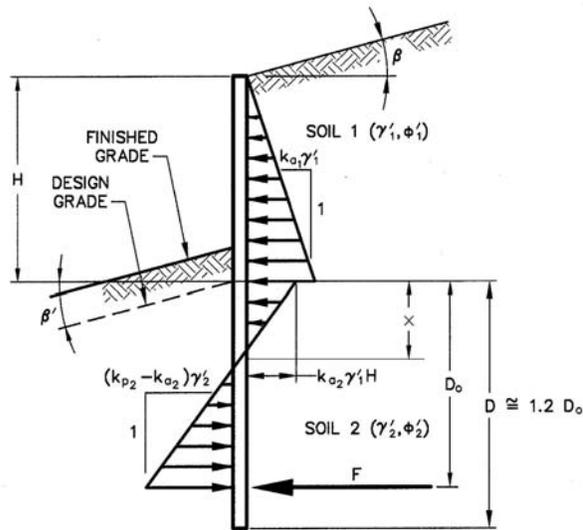
**Figure 3.11.5.6-3—Unfactored Simplified Earth Pressure Distributions for Permanent Nongravity Cantilevered Walls with Continuous Vertical Wall Elements Embedded in Granular Soil Modified after Teng (1962)**
