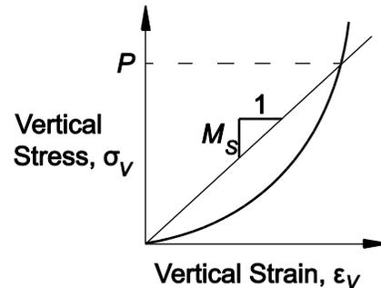
Figure C12.12.3.5-1—Schematic One-Dimensional Stress-Strain Curve of Soil Backfill
