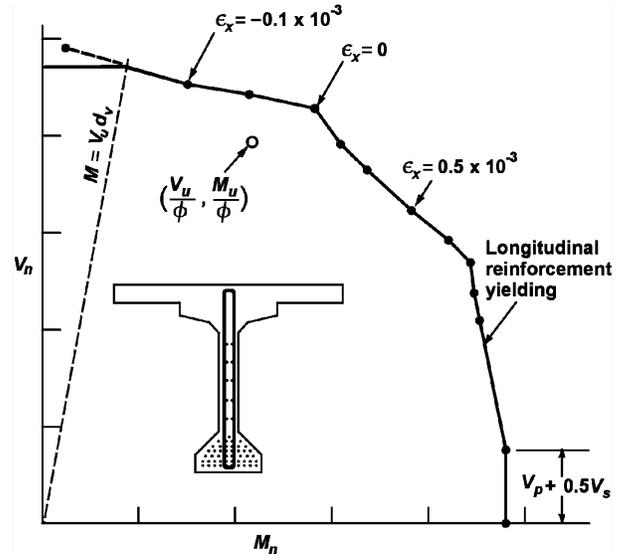
Figure CB5.2-6—Typical Shear-Moment Interaction Diagram
