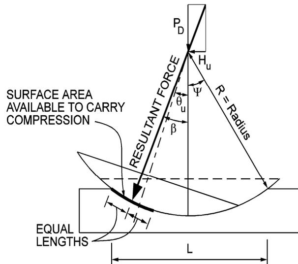
**Figure C14.7.3.3-1—Bearing Geometry**
