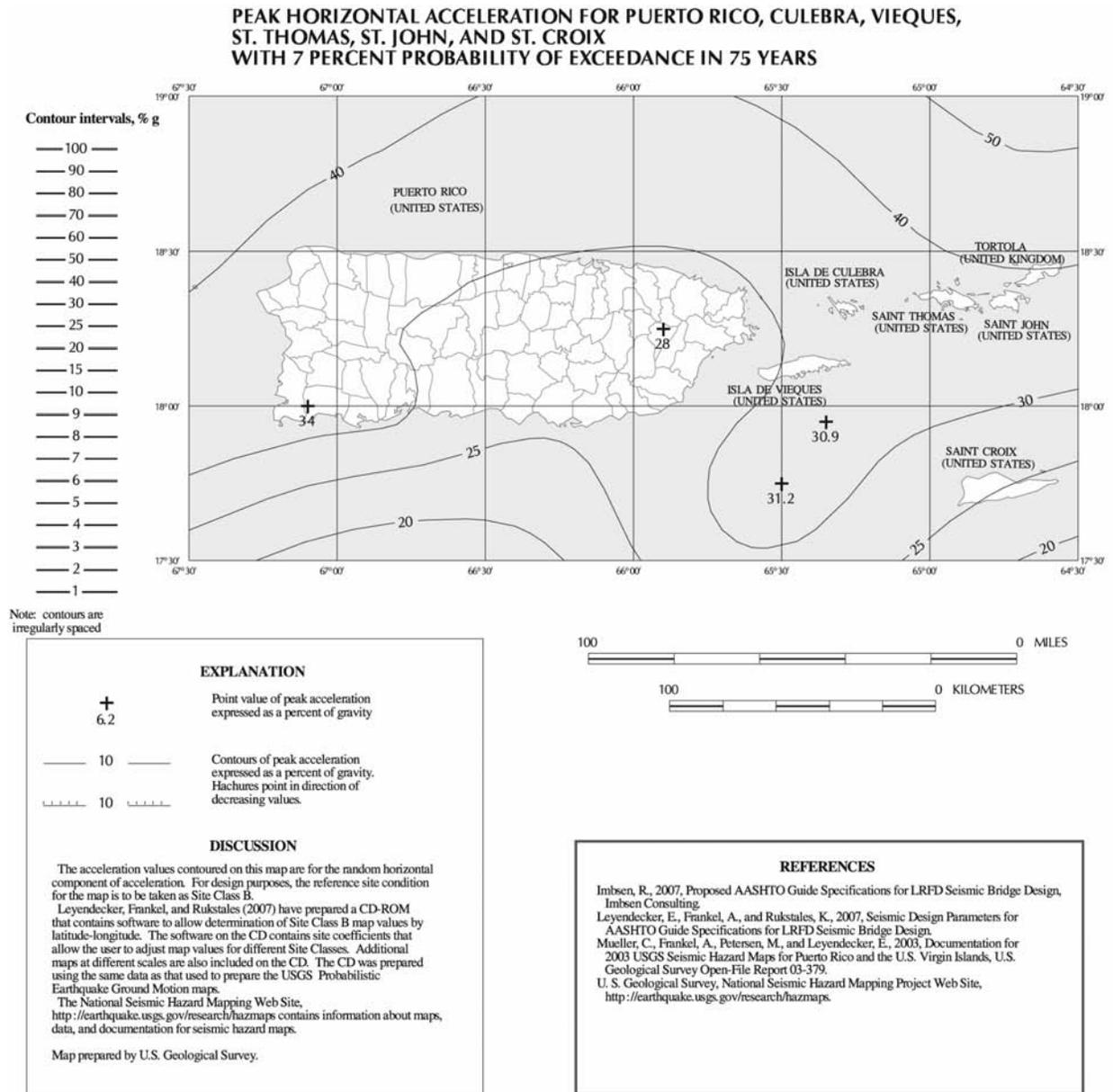
**Figure 3.10.2.1-20—Horizontal Peak Ground Acceleration Coefficient for Puerto Rico, Culebra, Vieques, St. Thomas, St. John, and St. Croix (PGA) with Seven Percent Probability of Exceedance in 75 yr (Approx. 1000-yr Return Period)**
