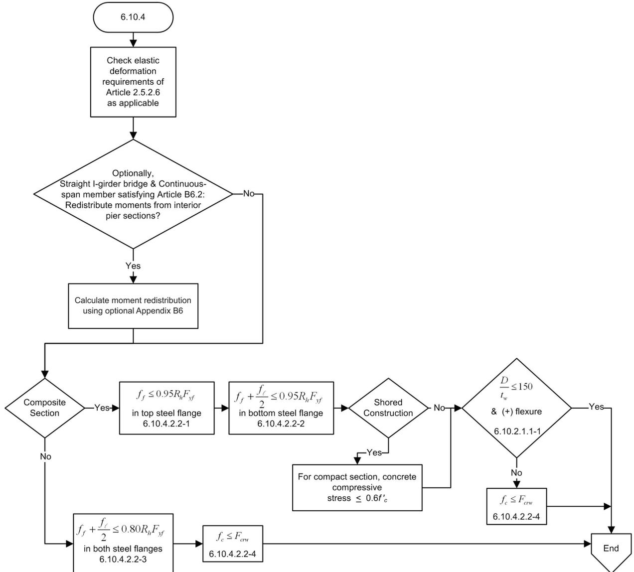
Figure C6.4.2-1—Flowchart for LRFD Article 6.10.4—Service Limit State
