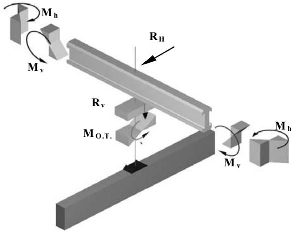
**Figure 14.5.6.9.7b-1—Force Effects Associated with Type A Cracking**
