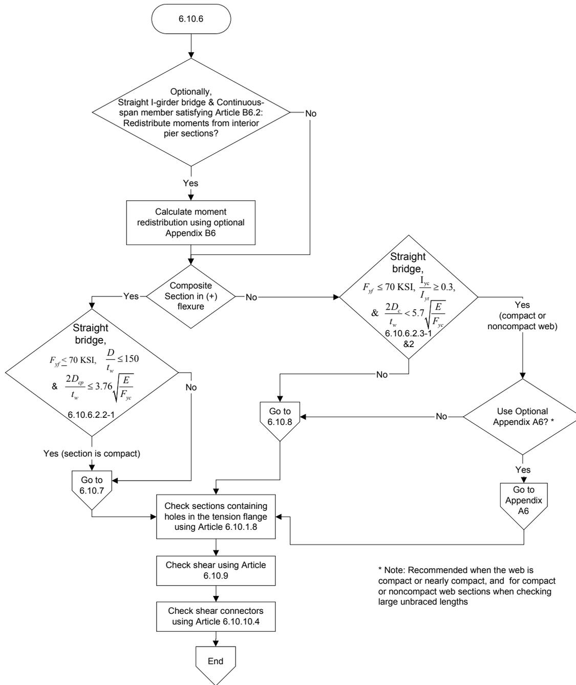
Figure C6.4.4-1—Flowchart for LRFD Article 6.10.6—Strength Limit State
