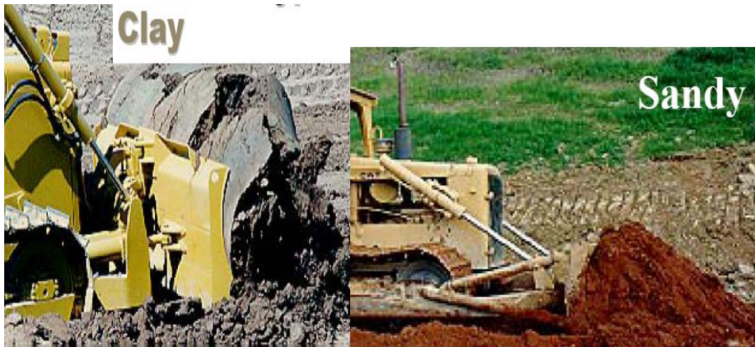
Figure 2.1 clay material boiling in front of the blade and cohesion less and loam in front of the blade
